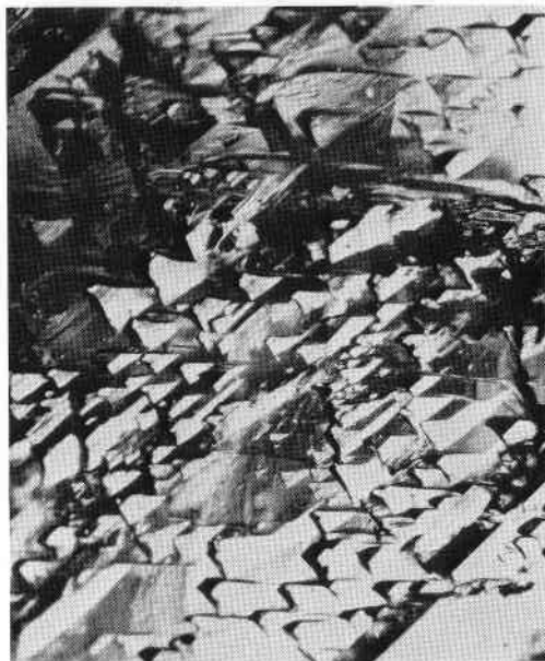
Figure 10. Microphotograph of triangular etch pits on the surface of kunzite from the Pala district.
