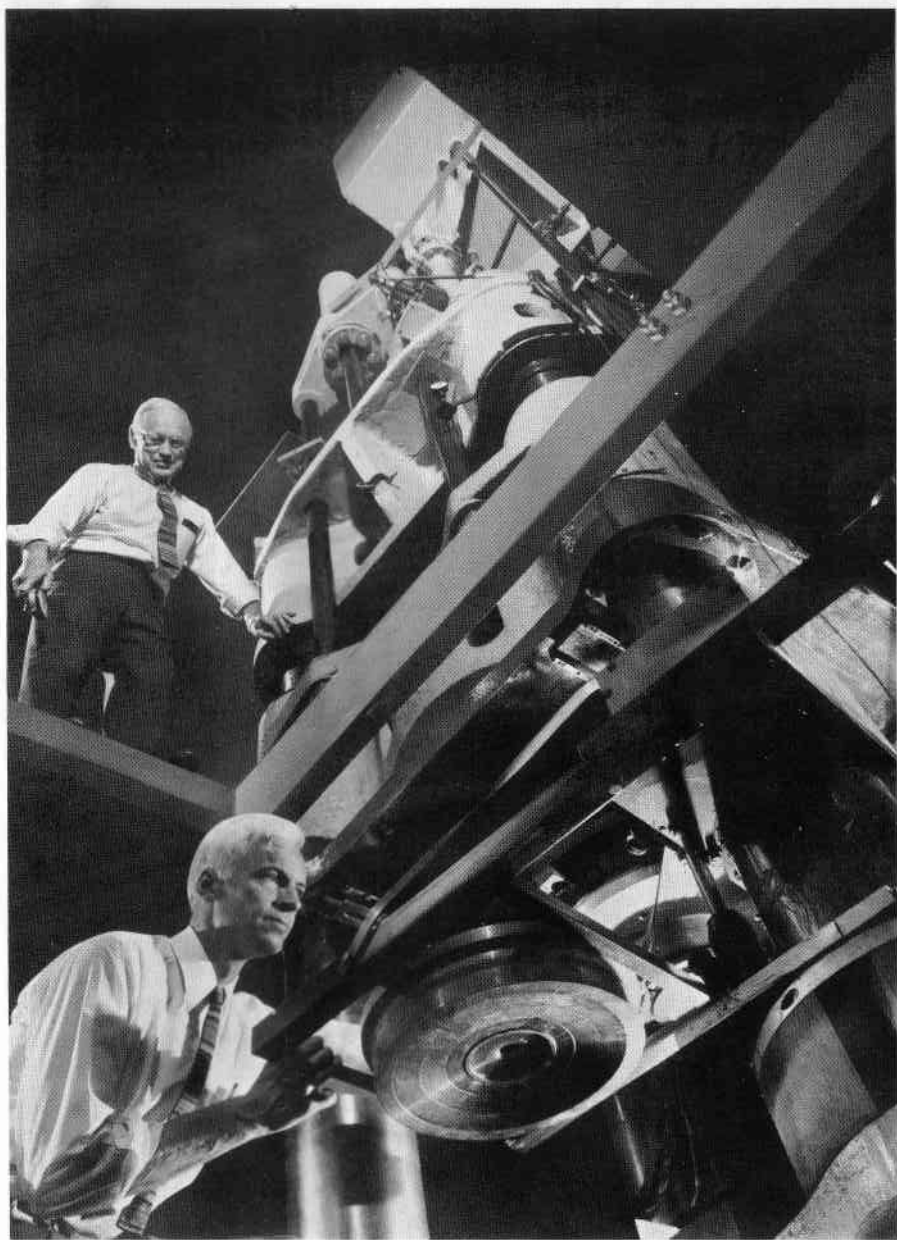
Dr. Herbert M. Strong (upper left) and Dr. Robert H. Wentorf, Jr., developers of the gem diamond processes, ready a giant press for a "run" at the GE Research and Development Center, Schenectady, New York.
