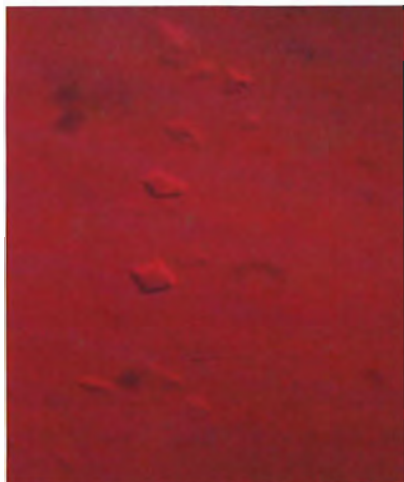
Figure 15. Angular crystals with slightly rounded corners in a Chatham synthetic ruby. Magnified 54 \times .
