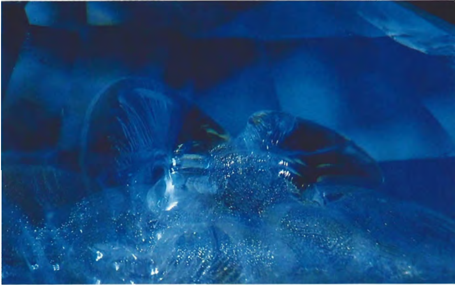
Figure 5. The stress fractures in this sapphire from Sri Lanka resulted from a heat treatment method like the one described in process 3. Photomicrograph by Robert E. Kane.
