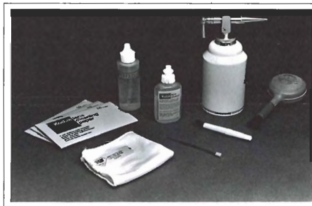
Figure 1. A collection of items useful in cleaning microscope and gem alike. These are, from left to right: lens paper, lint-free gem cloth, lens cleaner (two brands displayed here), needle probe, small camel's hair brush, can of compressed air, and camel's hair blower brush.
