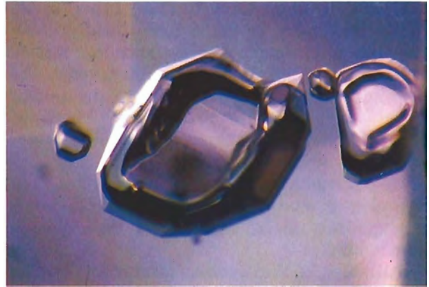
Figure 19. Under combined transmitted and oblique illumination, these negative crystals show not only their detailed form but also the amethystine coloration of their Brazilian quartz host. Magnified 70×.
