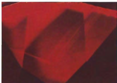
Figure 16. Angular growth lines extending completely through a Chatham synthetic ruby. Magnified 38 \times .
