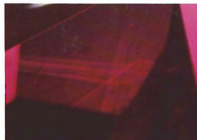
Figure 17. Straight, angular, and intersecting growth lines in a Chatham synthetic ruby. Magnified 39 \times .
