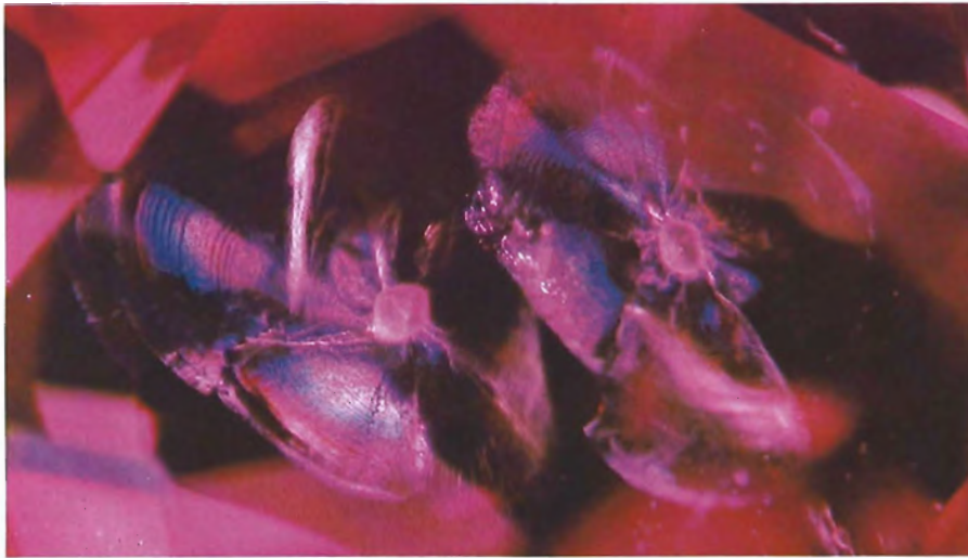
Figure 2. The stress fractures surrounding inclusions in this ruby were produced by a heat treatment method similar to the one discussed in process 2. Magnified 27 \times . Photomicrograph by Robert E. Kane.
