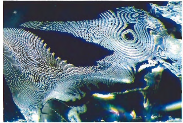
Figure 5. The descriptive term fingerprint readily applies to partially healed fractures such as this one in rock crystal quartz from Brazil. Dark-field illumination, magnified 50 \times .
