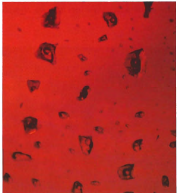
Figure 11. This secondary healing plane of tiny negative crystal fluid inclusions in a spessartine garnet from Virginia is well detailed by transmitted light. Magnified 75×.
