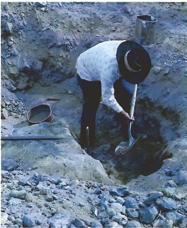
Figure 5. The freed chunks of peridot on matrix are shoveled into a sizing sieve.
