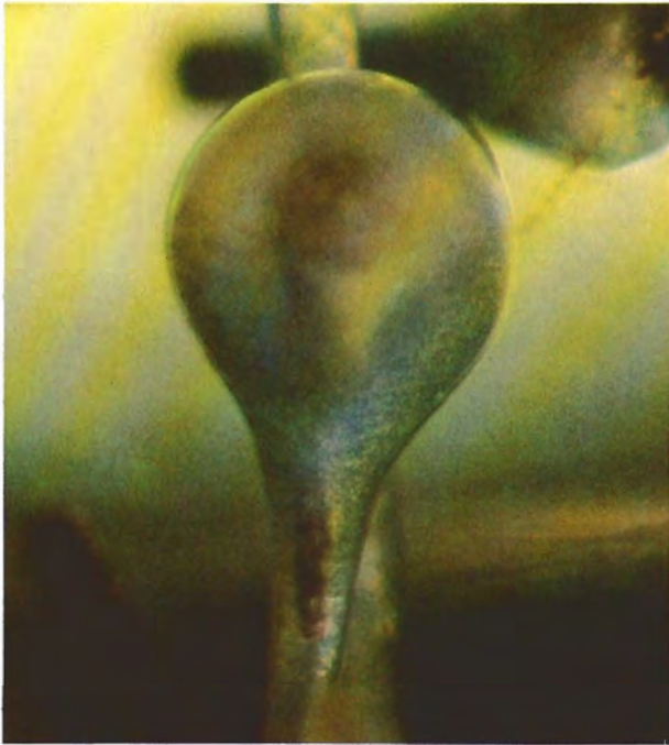
Figure 11. This two-phase inclusion in Mexican opal consists of an acicular crystal of hornblende within a balloon-shaped void. Magnified 45 \times .
