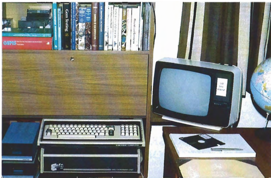
Figure 1. The author's Exidy Sorcerer computer installation. To the left of the keyboard is a Micropolis disk-drive unit. To the right is one of the floppy (magnetic) disks containing the computer program.
