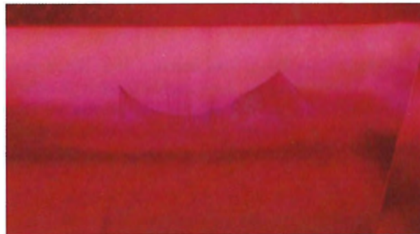
Figure 25. Curved and straight growth features associated with color zoning in a Ramaura synthetic ruby. Diffused and fiber-optic illumination, magnified 30 \times .
