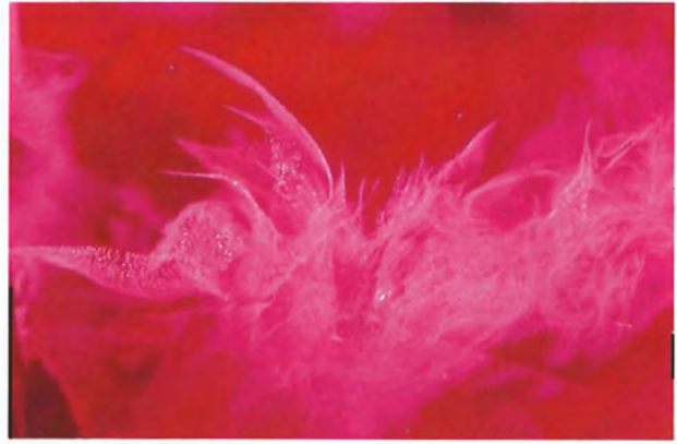
Figure 13. White, wispy veils, fine to moderate in texture, betray the synthetic origin of this Ramaura synthetic ruby. Dark-field and oblique illumination, magnified 40 \times .
