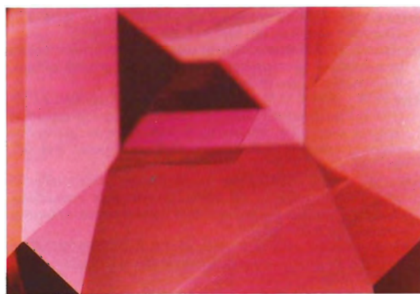
Figure 26. Diffused illumination accentuates different forms of color zoning and growth features in this Ramaura synthetic ruby. Magnified 15 \times .
