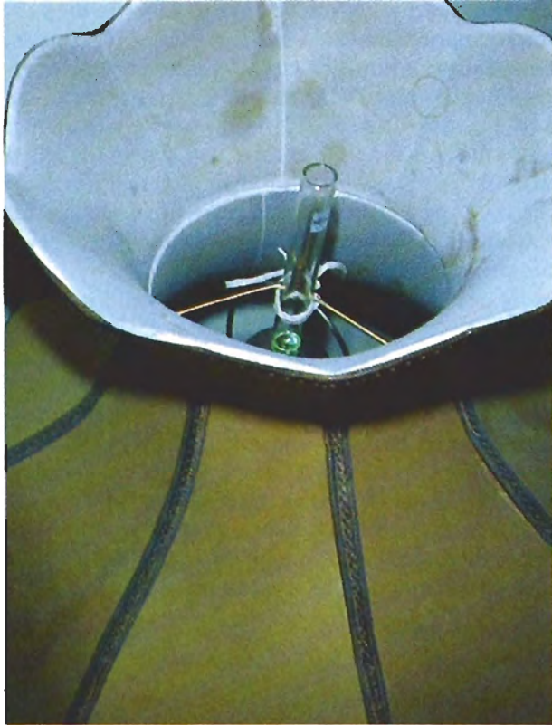
Figure 6. The lightbulb of an ordinary table lamp provides heat for maintaining the oil at a constant high temperature.
