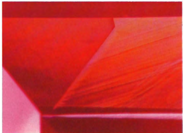
Figure 18. With the built-in iris diaphragm on the Gemolite microscope stage partially closed (over dark-field illumination) to create a shadowing effect in this Ramaura synthetic ruby, several different forms of growth features become evident. Particularly notable is the straight growth band that forms an angle in the center of this photomicrograph. Magnified 30x.
