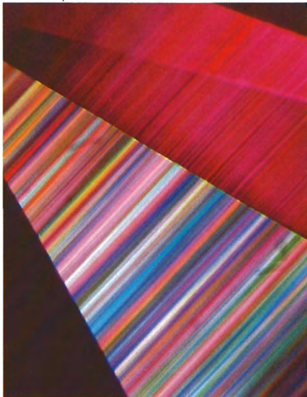
Figure 17. This Ramaura synthetic ruby displayed unusual growth features: at some viewing angles the nearly straight, parallel growth bands appeared similar to the left view in figure 16; at others, a complete iridescence was exhibited; and at still others, as is shown here, both features were observed. In this view, the very slight differences in angle between facets causes the growth features to be iridescent in one and not in the others. Dark-field illumination, magnified 50x.
