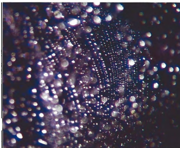
Figure 5. Characteristically oriented fingerprint-like feather consisting of minute spinel inclusions in a taaffeite from the Hattota Amuna gem deposit, Sri Lanka. Dark-field illumination, magnified 30x.
