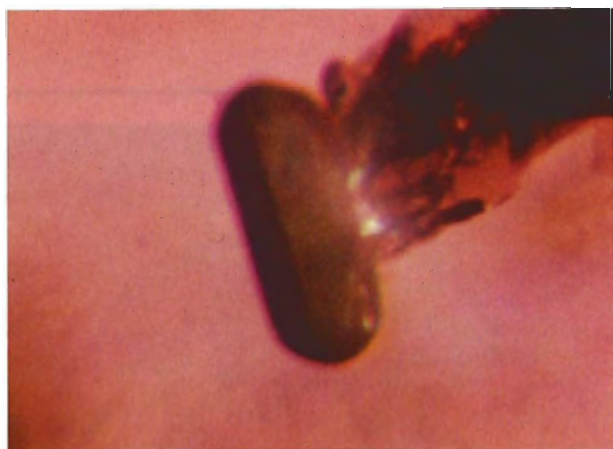
Figure 2. Distinctly developed crystal of apatite in a taaffeite from Sri Lanka. Dark-field illumination, magnified 45×.
