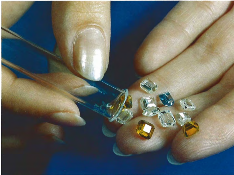
Figure 2. A selection of rough synthetic gem-quality diamond crystals grown by General Electric in 1970. Photo courtesy of General Electric.
