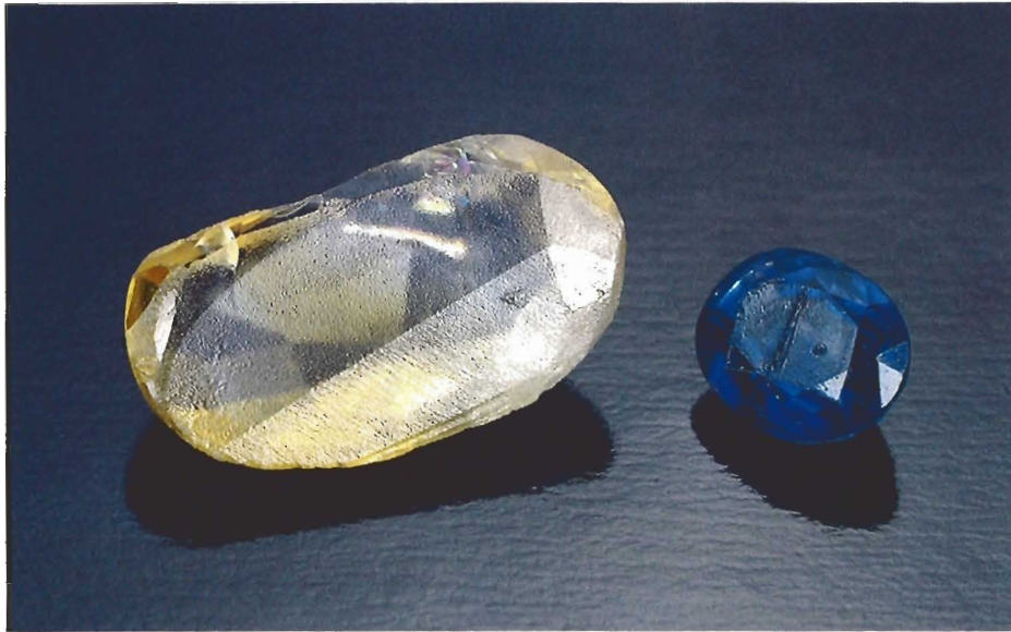
Figure 15. The irregular glass coatings on the surfaces of these treated sapphires (4.91 ct and 0.98 ct) formed as a by-product of heat treatment, specifically, by the melting of a coating solution that was used to prepare the sapphires for heating. Photo ©1984 Tino Hammid.
