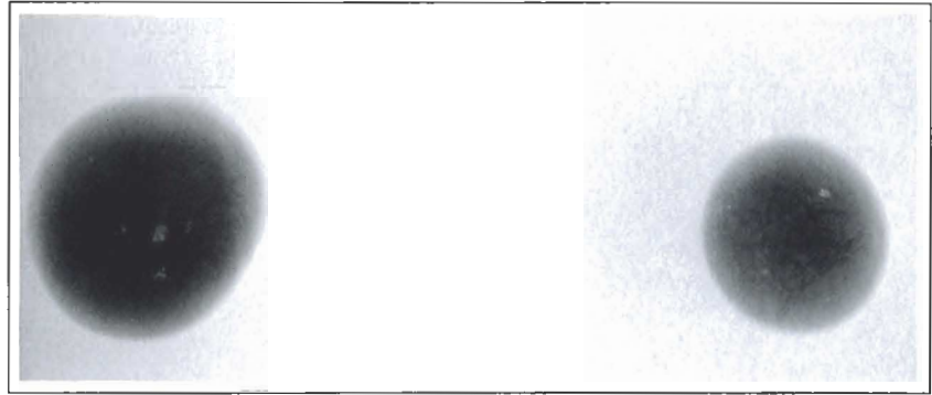
Figure 7. This X-radiograph shows two of the American freshwater cultured pearls examined in the New York and Los Angeles laboratories. The irregular nucleus characteristic of mantle-tissue nucleation is prominent in the pearl on the left and less obvious, though clearly visible on film, in the one on the right.
