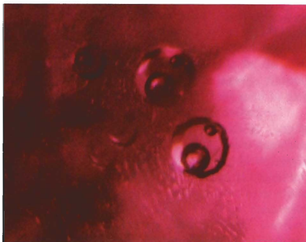
Figure 11. Naturally occurring glass inclusions in a Thai ruby (the largest measures 0.10 mm in diameter). The fact that the three gas bubbles in the largest inclusion are stationary proves that this is a solid-and-gas rather than liquid-and-gas inclusion. Dark-field illumination, magnified 50×. Photomicrograph by John Koivula.
