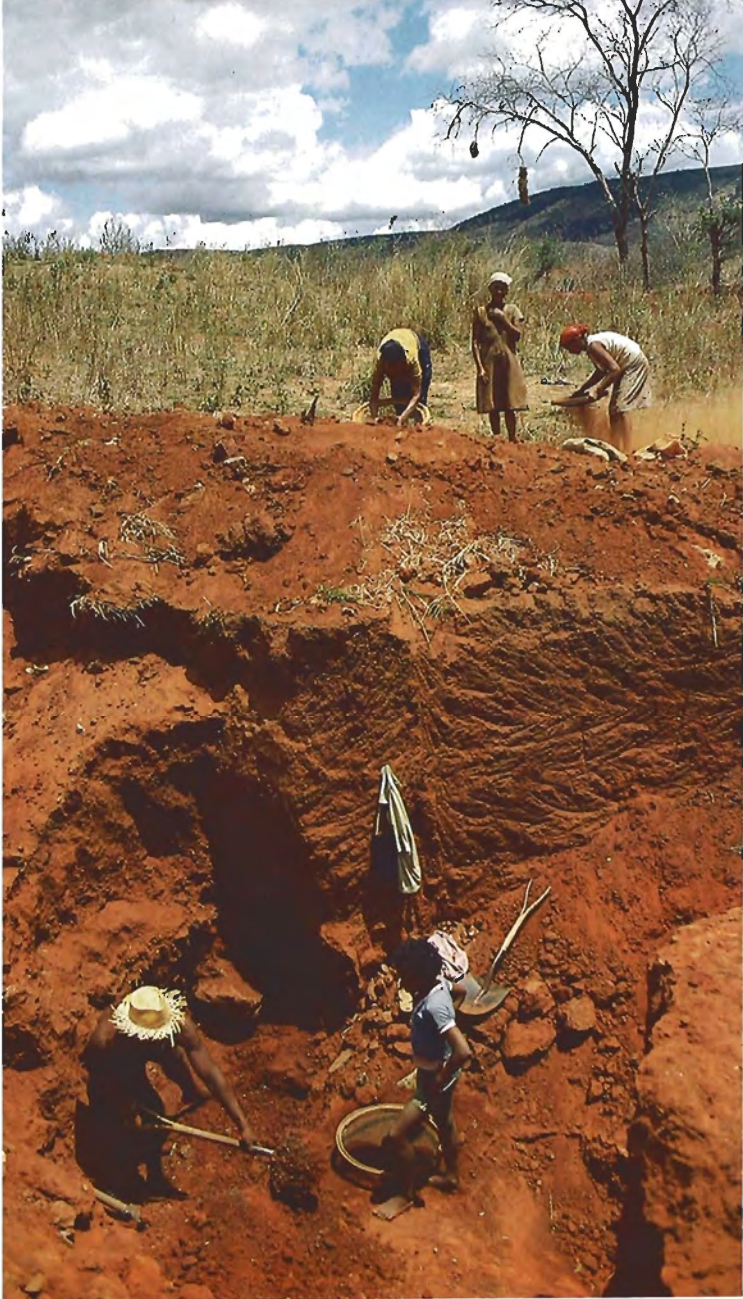
Figure 13. Picks and shovels are used by the garimpeiros, in this case an entire family, to mine the eluvial deposit at Ouro Fino. The material extracted by the father and son is placed in a sieve; the sieves are shaken by the three women above to concentrate the hard nodules of red clay from the remainder of the eluvial soil. Many of these "nodules" contain fractured pieces of fine Ouro Fino rubellite which can be freed by a washing operation.
