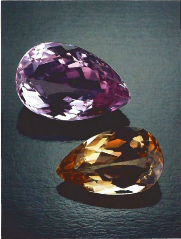
Figure 7. Heat treatment over an open flame turned a yellow topaz from the same lot as the 2.5-ct stone on the lower right into the attractive pink topaz on the upper left. Stones courtesy of P. Flusser, Overland Gems, Los Angeles, CA; photo © Tino Hammid.
