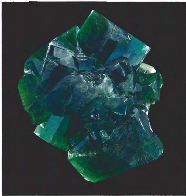
Figure 1. A cluster of flux-grown synthetic emerald crystals manufactured in the USSR. The largest crystal is 3 cm long \times 4.2 cm in diameter. Photo by Susan Gipson.
