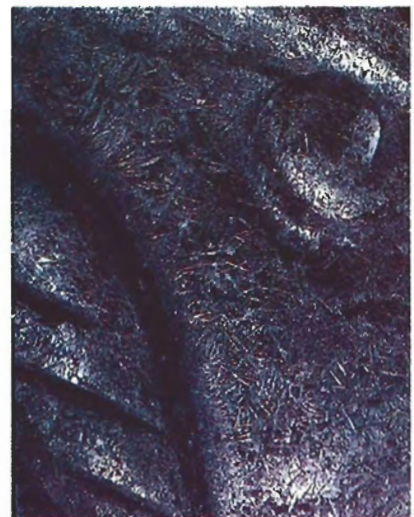
Figure 7. Extensive etching caused by immersion of the fluorite carving shown in figure 6 in a sulfuric acid solution. Magnified 30 \times .
