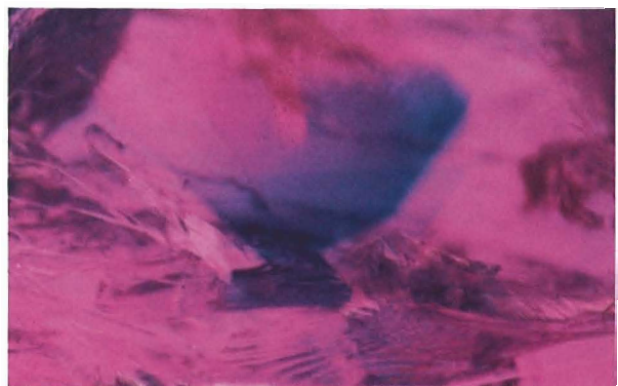
Figure 12. Unusual zones of strong blue color can be observed in some rubies from the Jegdalek mine. Dark-field illumination, magnified 35×. Photo by John Koivula.
