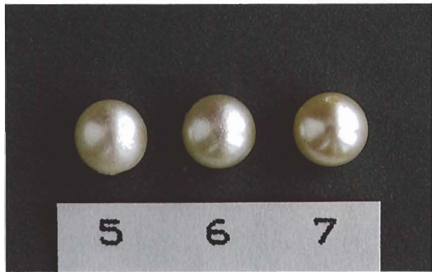
Figure 3. Pearls no. 5 and 6 from the acid cleaning experiments; an abrasive has also been used on no. 6; no. 7 is the untreated color match.
