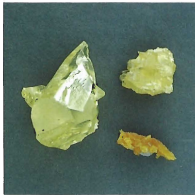
Figure 15. New hydrothermal synthetic zincite on the left, accidental synthetic zincite furnace products on the right.
