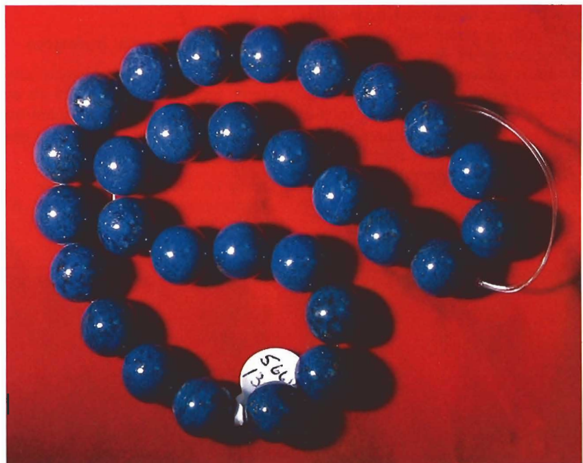
Figure 10. These 10-mm beads of Afghanistan lapis lazuli were found to have been oil treated.
