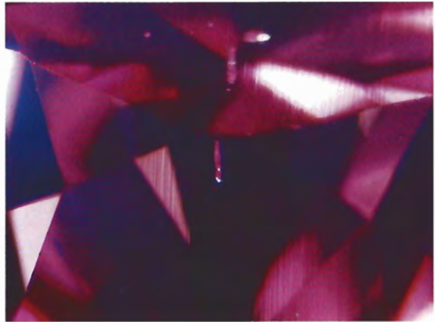
Figure 6. In the 0.59-ct purple-pink diamond, the strong linear banded strain patterns observed with polarized light (left, magnified 30 \times ) correspond directly to the color zoning and graining evident with darkfield illumination (right, magnified 25 \times ).
