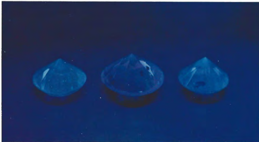
Figure 4. All three diamonds—from left to right here, the 0.59-ct, 0.95-ct, and 0.54-ct stones—fluoresced to long-wave ultraviolet radiation. Photo by Shane McClure.
