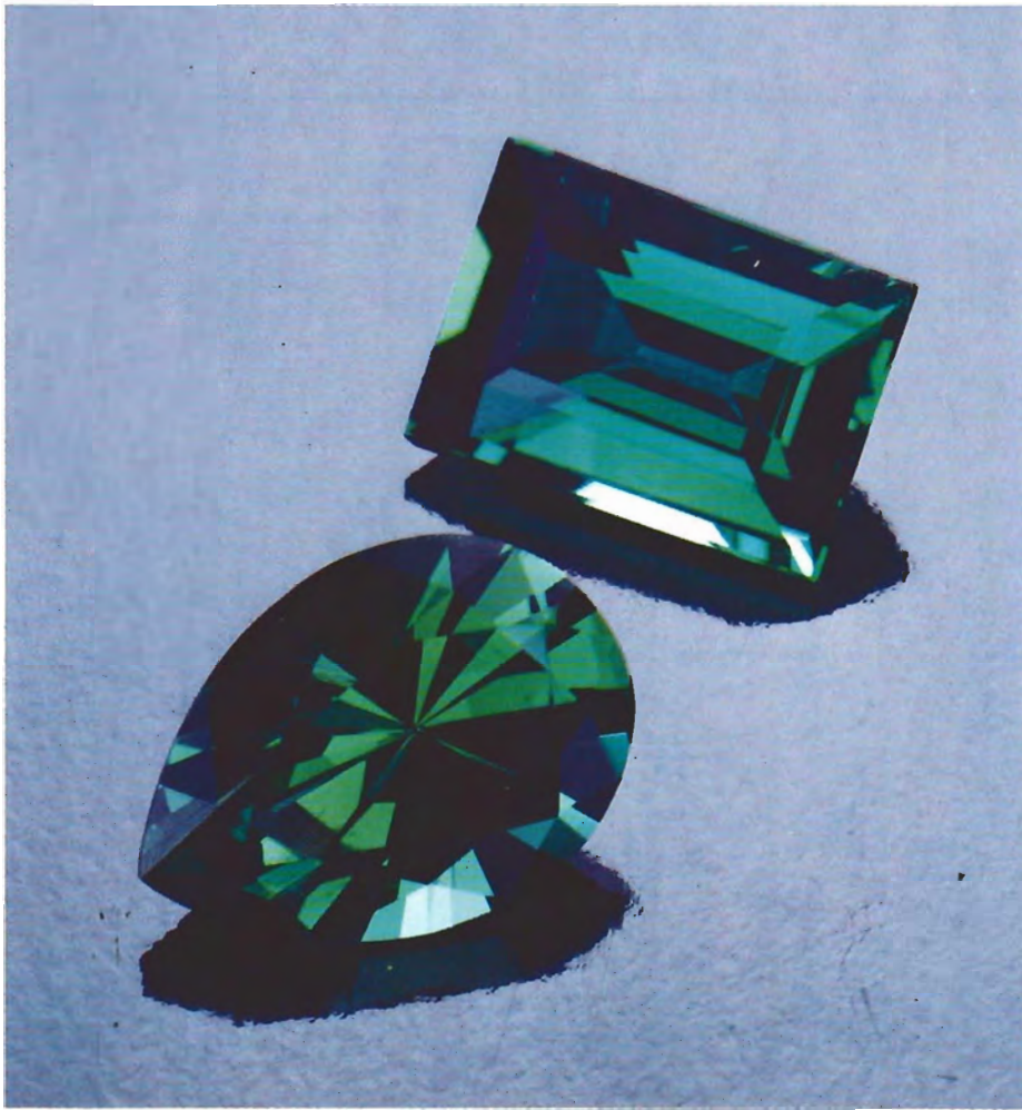
Figure 1. Among the more recent synthetic emeralds introduced are the Biron hydrothermal (top, 0.54 ct) and the Inamori flux (bottom, 0.56 ct) products. Photo © Tino Hammid.
