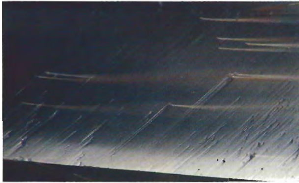
Figure 4. These polishing drag lines on the surface of a topaz extend from the ends of the "inclusions." Shadowed oblique illumination, magnified 25 \times .
