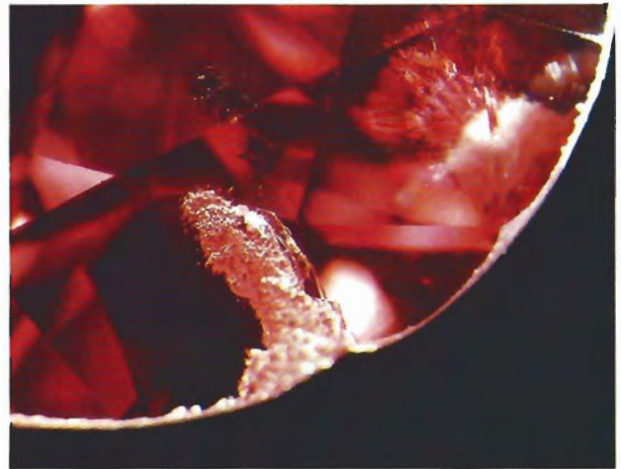
Figure 9. A second cavity in the 0.95-ct diamond begins at the girdle plane. Note the frosted appearance in reflected oblique illumination. Magnified 25 \times .
