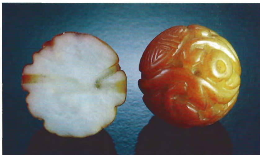
Figure 18. Dyed serpentine bead cut in half. The left side shows shallow dye penetration, while the right side shows the carved surface.
