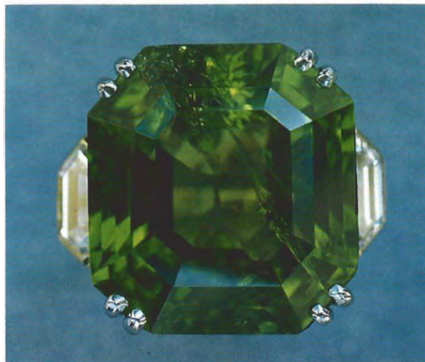
Figure 15. Thermal shock during a repair procedure on the mounting caused extensive internal cracking in this once-beautiful peridot.
