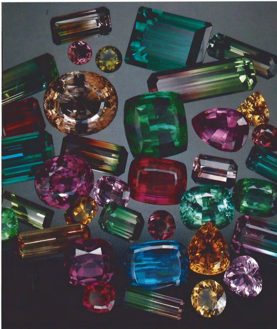
Figure 1. A number of different mechanisms are responsible for the variety of colors found in tourmaline. For example, the blue color of indicolite is caused by dispersed Fe^{2+} , but charge transfer between iron ions often contributes to the color of the green varieties. This article explains the influence of dispersed metal ions in the color of many different gem materials; the other two articles in this series will examine other causes of color such as charge transfer. Photo © Harold & Erica Van Pelt.
