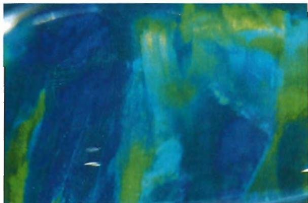
Figure 2. The columnar structure of the color "grains" is evident in this Kyocera opal imitation with black body color. Magnified 20×.
