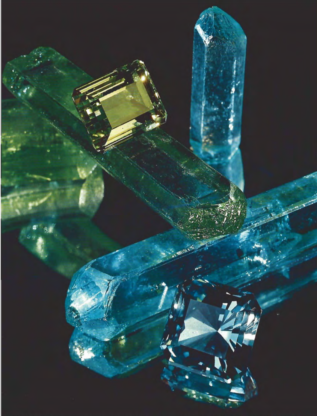
Figure 7. In beryl, Fe^{3+} causes yellow and Fe^{2+} causes blue; green beryl is a mixture of Fe^{3+} and Fe^{2+} . The common practice of heating green beryl modifies the valence state of the Fe^{3+} such that the yellow color is removed and only blue (aquamarine) remains. Photo © Harold & Erica Van Pelt.
