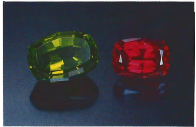
Figure 10. Both green peridot and red pyrope-almandine garnet are primarily colored by \text{Fe}^{2+} . The striking difference in color is caused by the difference in ion coordination, which is octahedral in peridot and distorted cubic in garnet. Photo by Shane McClure.
