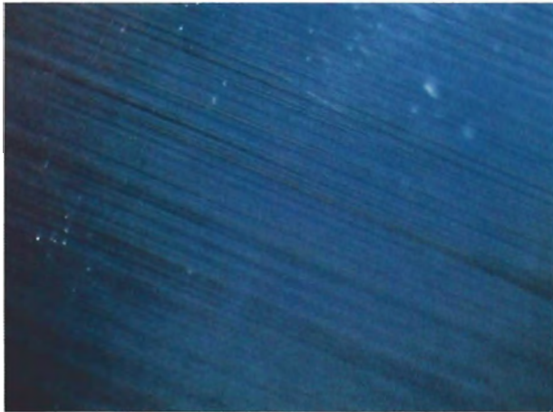
Figure 5. Oblique illumination created with a fiber-optic light unit reveals the nondescript, white-appearing, minute particles—specifically oriented in parallel planes (in association with the undulating striations shown in figure 4)—that give rise to the chatoyancy in this Inamori synthetic cat's-eye alexandrite. The larger white spots are surface features on the stone. Magnified 45 \times .
