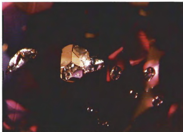
Figure 8. Dr. Edward Gübelin, Dr. Karl Schmetzer, and Mr. Charles Schiffmann identified apatite as an inclusion in the Hematita alexandrites. Stone courtesy of Robert Van Wagoner, Aspen, CO. Magnified 25 \times ; photomicrograph by John I. Koivula.
