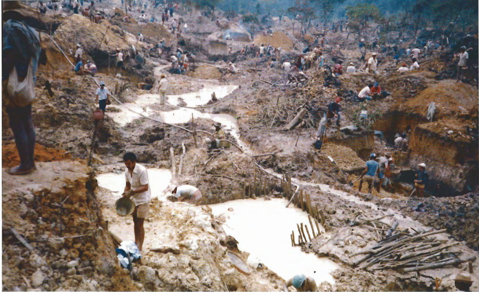
Figure 13. Within a matter of weeks after the Hematita deposit was discovered by local miners and dealers, both sides of this meandering brook, and even the brook itself, were invaded by thousands of miners. Note in the pit on the right the clear demarcation of three layers—an overburden of clay and sand, the heavily quartz- and kaolin-bearing gem gravel, and a dark layer of what appears to be clay below that. The apex of this small, triangular-shaped valley pinches in at the top of the photo. Photo by Agenor Tavares.
