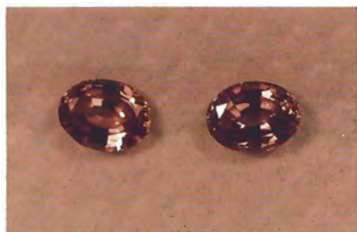
Figure 1. These two 1.50-ct synthetic alexandrites have a color change very similar to that of natural Brazilian alexandrite. Here they are seen in incandescent light.
