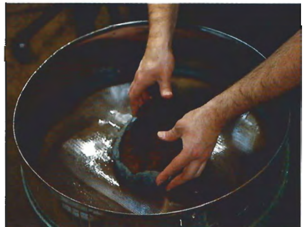
Figure 8. On large stones, it is advisable to cut and polish the table before any other facets. Here, a Recipro-Lap is used to touch up the table on the large citrine. A waterproof clay-like substance has been placed around the girdle to protect the finished portions. Photo by Robert Weldon.
