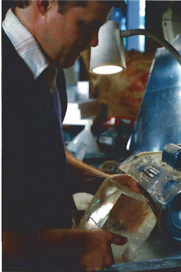
Figure 7. After the stone has been sawed, it is preformed on a coarse grinding wheel that has been mounted in a cabochon-making machine. Here, a calcite is being rough ground prior to dopping. Photo by Robert Weldon.
