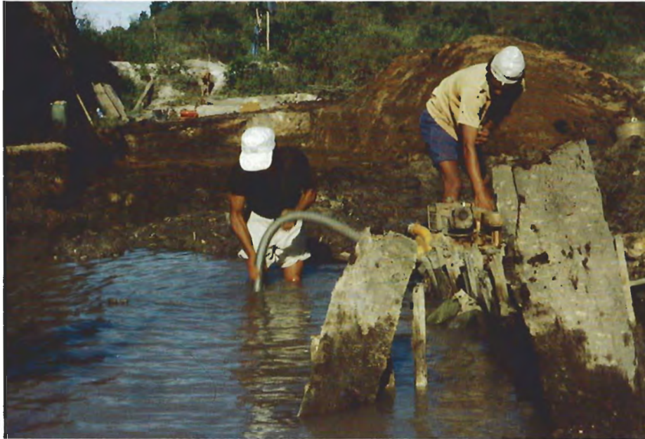
Figure 5. Water is an on-going problem at Barro Preto. Periodically during the day, the miners must pump the water out in order to gain access to the gem-bearing gravels. Photo by Henry Kennedy.
