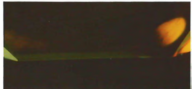
Figure 6. Green transmission and the "umbrella effect" proved that this diamond had been cyclotron treated. Fiber-optic side lighting, magnified 30 \times .
