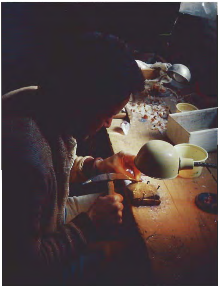
Figure 12. Before cutting-quality amethyst is sold on the open market, pale-colored or fractured sections are usually broken off with a small hammer in a procedure called "cobbing."
