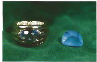
Figure 16. Both of these synthetic spinels were originally sold as topaz. The stone set in the ring measures 11.0 × 6.8 × 7.5 mm; the loose preform measures 15.0 × 10.0 × 10.0 mm.
