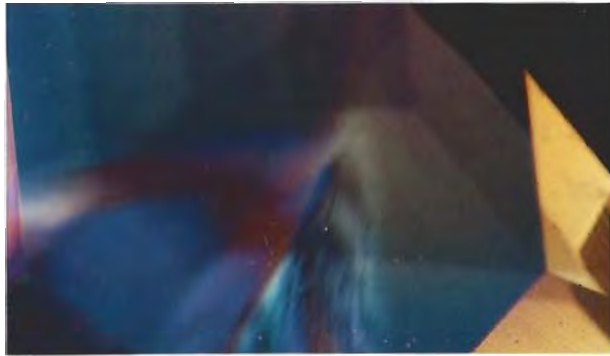
Figure 3. Flame-like Brazil-law twin patterns are also observed in faceted natural amethyst. Photomicrograph by John I. Koivula; polarized light, magnified 4 \times .
