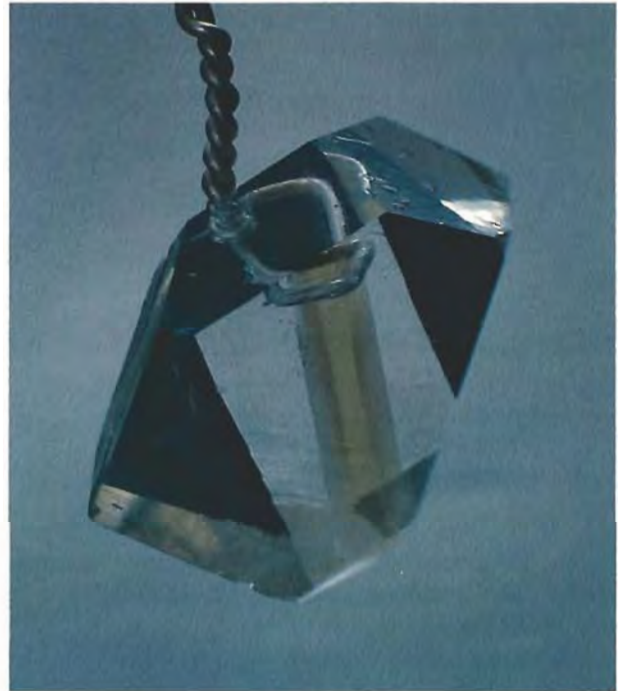
Figure 5. When a Brazil law-twinned amethyst seed plate oriented near-perpendicular to the c -axis direction was used, the resulting 16-mm-long synthetic quartz crystal took a form more closely resembling that of natural quartz. Heat generated during the growth process converted the amethyst seed to citrine. Irradiation would restore the purple color. Photo by Robert Weldon.
