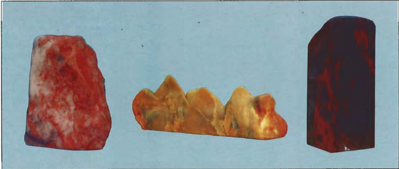
Figure 2. Left: The base rock in this example of chicken-blood stone is referred to as white dong in China. Center: This pen rack is carved from yellow dong chicken-blood stone. Right: This seal has a deep gray dong groundmass. All three specimens are from Changhua.
