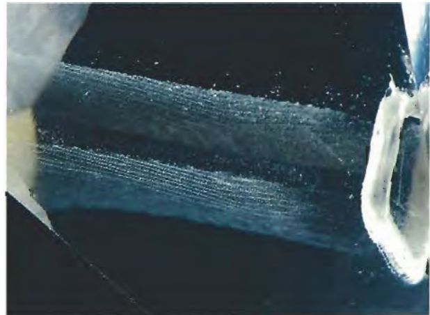
Figure 6. The rib-like structure of the twinning appeared as a phantom at the interface between the seed plate and the synthetic overgrowth. Photomicrograph by John I. Koivula; darkfield and oblique illumination, magnified 4 \times .
