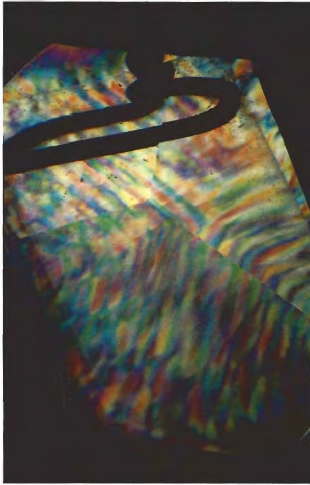
Figure 7. Both of the experimental crystals showed Brazil twinning in the overgrowth as well as in the seed plate. Photomicrograph by John I. Koivula; immersion and polarized light, magnified 3×.
