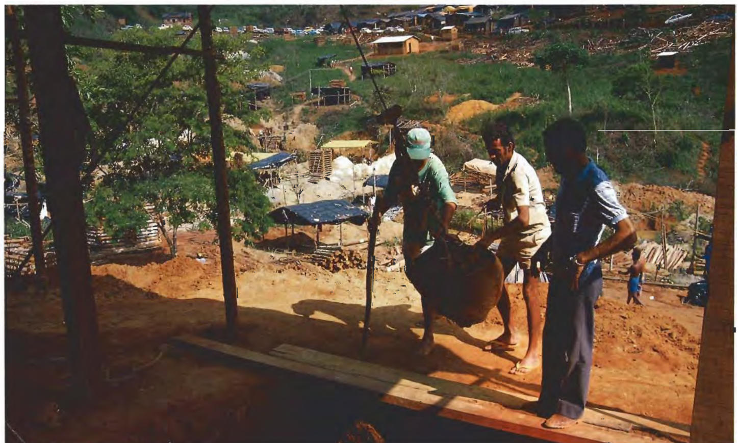
Figure 6. Shafts as deep as 35 m penetrate the schist rock at Capoeirana. Crude buckets are used to remove the soil overburden and the potentially gem-bearing rock. Photo © Bryan Swoboda.
