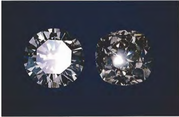
Figure 2. The flat diamond table on the left reflects light evenly, while the concave one on the right condenses the light to a single spot.
