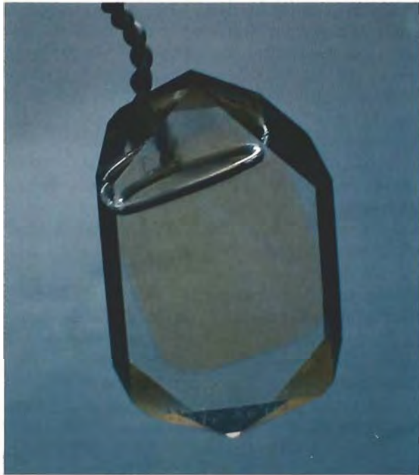
Figure 4. A natural Brazil law-twinned amethyst seed plate oriented near-parallel to the c -axis direction resulted in this 3-mm-thick, 15-mm-long tabular synthetic quartz crystal. Photo by Robert Weldon.
