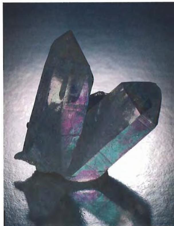
Figure 12. "Rainbow" quartz is reportedly produced by allowing molecules of silver/platinum to adhere to the external surface of the quartz. This cluster weighs 17.86 grams. Photo by Robert Weldon and Maha Smith.
