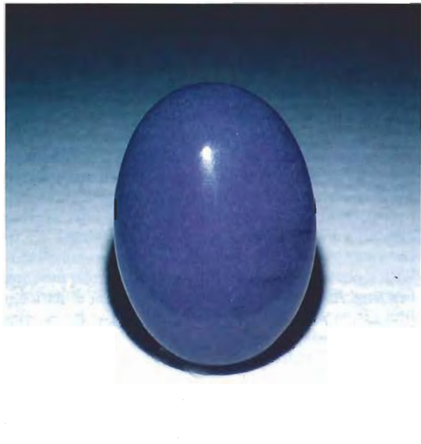
Figure 16. Sold as "purple onyx," this 8.87-ct purple dyed quartzite could be mistaken for sugilite. Photo by Robert Weldon and Maha Smith.
