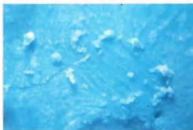
Figure 17. Magnification (at 45 \times ) of the scraped surface of the acid-treated chip of imitation turquoise revealed curls of the plastic binder.
