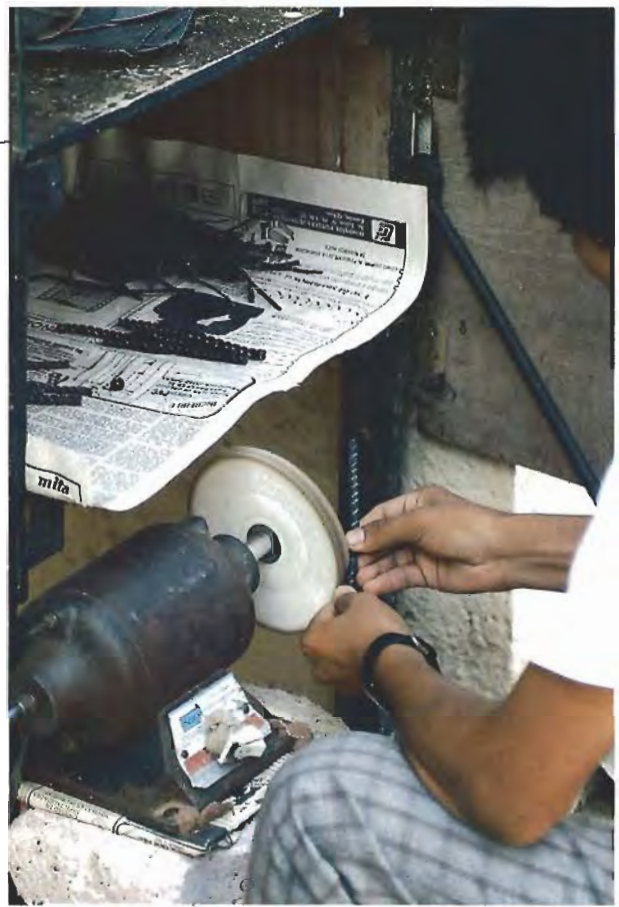
Figure 3. This craftsman in San Miguel de Cozumel uses a lathe-driven cotton buff to polish a piece of Caribbean black coral. Photo by Robert C. Kammerling.
