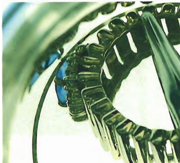
Figure 11. Immersion and diffused illumination reveal the characteristic color concentrations along facet junctions that prove that this ring-set sapphire has been diffusion treated. Photo by Nicholas DelRe.
