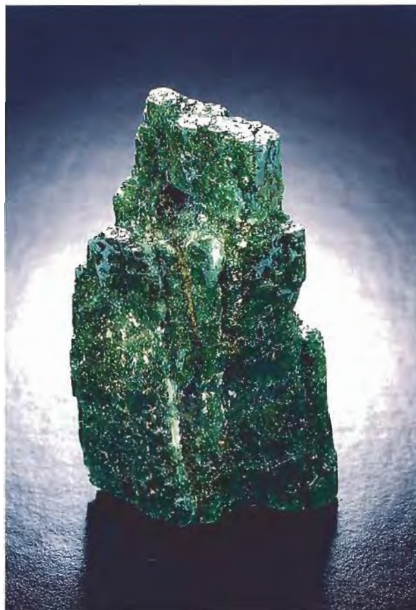
Figure 1. This 76.42-ct “Emeraldolite” specimen consists of a flux-grown synthetic emerald overgrowth on natural white beryl. Photo by Robert Weldon.
