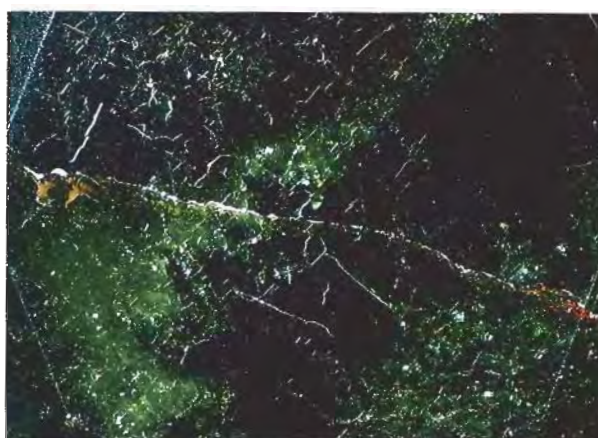
Figure 3. Artificially irradiated black-appearing diamonds typically reveal a dark green coloration through thin, relatively transparent edges when examined with intense illumination. This treated diamond, however, appeared green throughout most of the stone, even under the table as shown here. Photomicrograph by Robert E. Kane; magnified 10 \times .
