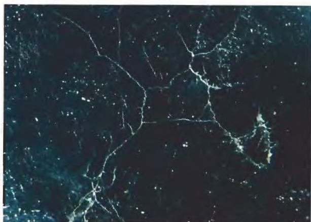
Figure 2. Even with the unaided eye, numerous breaks can be seen reaching the surface of the black diamonds, as illustrated here by one of the round brilliants. Photo by John I. Koivula; oblique illumination.
