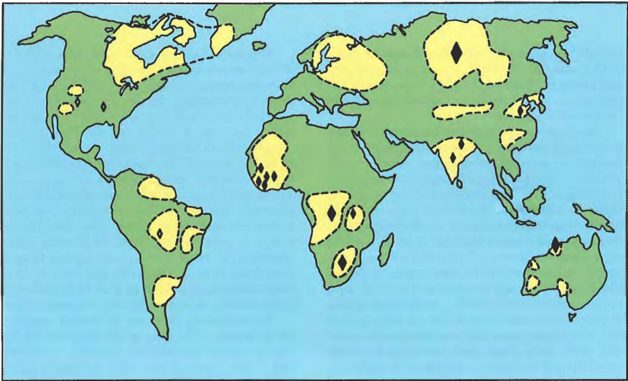
Figure 15. This world map of primary diamond deposits (i.e., those in pipes) shows cratonic areas (dashed lines) with major economic diamond deposits (large solid diamonds), minor economic deposits (small solid diamonds), and subeconomic deposits (small open diamonds). The economic deposits are in kimberlites except for the Australian deposit(s), which are in lamproite. Note that several cratons have no known diamond deposits. From Gurney (1989) and based on data in Janse (1984).
