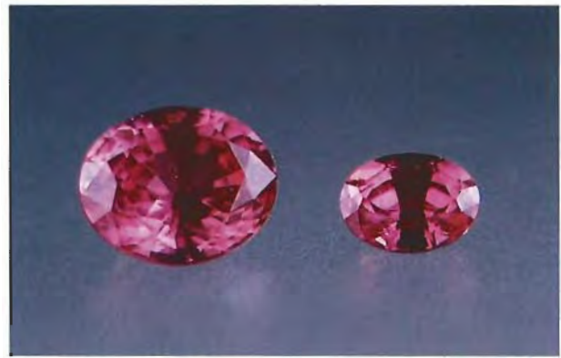
Figure 16. The Czochralski "pulling" method was used to produce these synthetic alexandrites, 3.63 ct. and 1.14 ct. Photo by Maha Smith.
