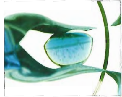
Figure 4. The colorless and green zones in this 3.90-ct cabochon are readily apparent with immersion. Although they suggest that this might be an assembled stone, testing proved that it was natural near-colorless beryl with a zone of emerald.
