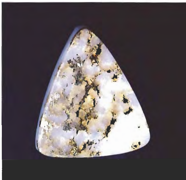
Figure 19. A thin (approximately 1.5 mm) layer of gold in quartz is backed with white ceramic to produce this 17.10 \times 5.00 \times 3.50 mm assembled stone. Photo by Maha Smith.
