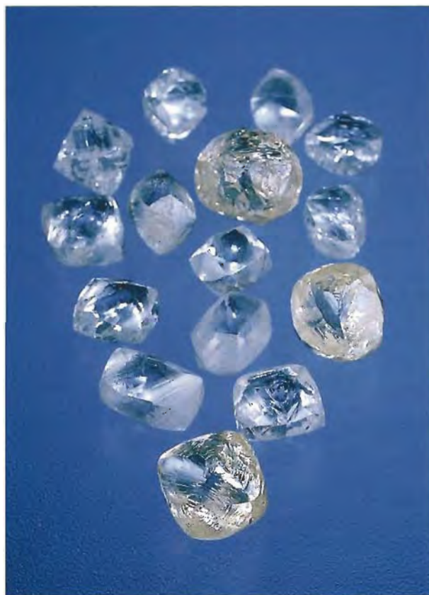
Figure 17. The irregular rounded shapes frequently found on diamonds result when the transporting kimberlite (or lamproite) magmas react with, and dissolve, the diamond, starting with the octahedral edges. Isolation of diamonds from transporting magmas (see figure 16), or very rapid ascent to the surface, can minimize this effect. Photo © GIA and Tino Hammid.
