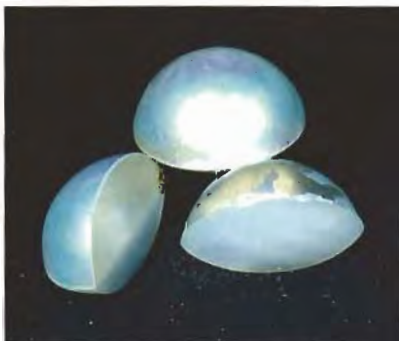
Figure 12. When one of these two 15.5-mm mabe pearls was sawed in half, the mother-of-pearl base, plastic dome, and very thin nacre layer were evident (left). Note also the coating on the plastic dome (right).
