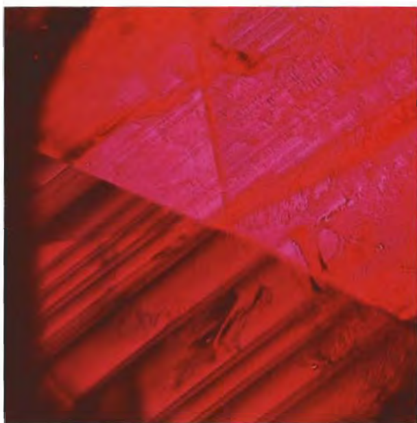
Figure 17. Laminated twinning was observed in many of the Vietnamese corundums. Polarized light, magnified 35 \times ; photomicrograph by Robert E. Kane.
