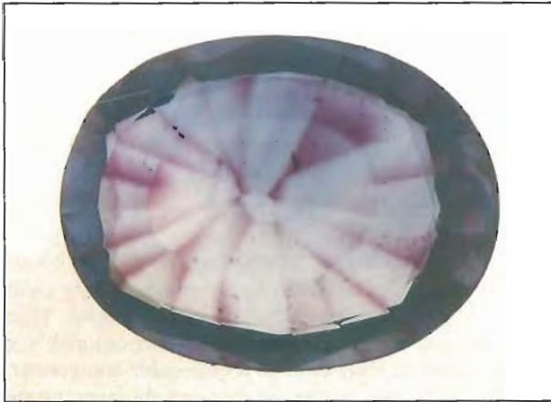
Figure 13. Diffused transmitted illumination reveals that what little diffusion-produced color remained after repolishing this experimentally treated sapphire was concentrated along facet junctions. Photo by John I. Koivula.
