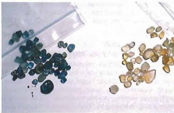
Figure 11. The improvement in color brought about by heat treating sapphires from Dry Cottonwood Creek, Montana, is readily apparent in these photographs showing typical material before (top) and after (bottom) enhancement. Photos by Maha Smith.
