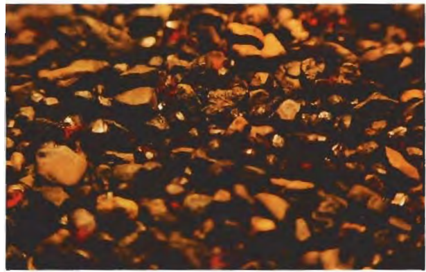
Figure 6. In this garnet concentrate from the Podsedice deposit, red pyropes (up to 5 mm) are easily seen among the other mafic minerals and rock fragments. Photo by J. Schlüter.
