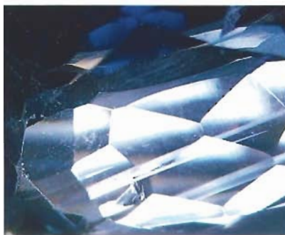
Figure 13. The repeated twinning evident in this 17.95 × 13.90 × 6.80 mm synthetic blue sapphire had led the client to believe it was natural. Magnified 10×.
