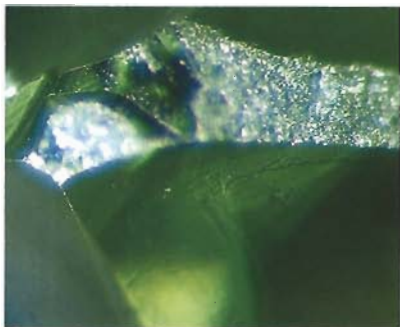
Figure 2. Natural dark green radiation stains were seen on the girdle at each point of this 0.82-ct treated green diamond. Magnified 30×.
