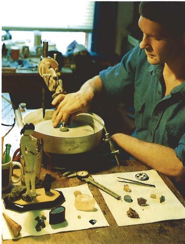
Figure 4. Although standard equipment is used for these cuts, considerable "play" is needed in the faceting head to allow for small adjustments in facet placement. Here, the author is actually touching the lap with his fingertips to maintain maximum control while cutting a freehand curve. Photo by Martha Wilhelm.
