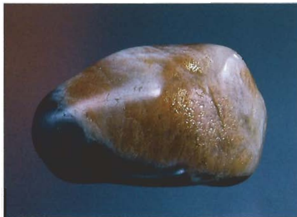
Figure 15. This 40-mm-long tumble-polished pebble consists of an unusual intergrowth of sunstone feldspar and iolite. Photo by Maha Smith.
