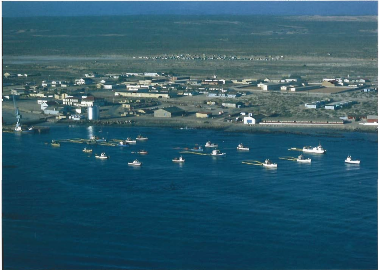
Figure 15. The harbor and village of Port Nolloth are home to numerous small boats used in offshore diamond mining. Most of the boats seen here are converted fishing trawlers, each equipped with a decompression chamber as well as with two 20-cm pumps to recover gravel. Divers who work from these boats use gas mixtures and heated diving suits that enable them to dive as deep as 40 m. Most of these boats, as well as the harbor facilities, are owned by Benguela Concessions.
