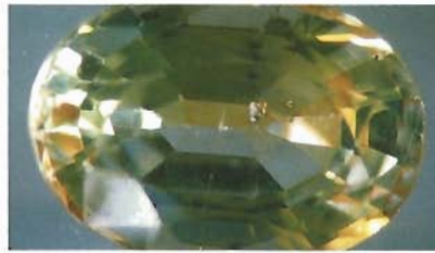
Figure 11. After the sapphire shown in figure 10 had been soaked at room temperature for five hours in concentrated HCl, the depth of color was reduced considerably.
