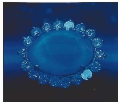
Figure 5. When the stone shown in figure 4 was exposed to long-wave U.V. radiation, the discolored area fluoresced pale blue.
