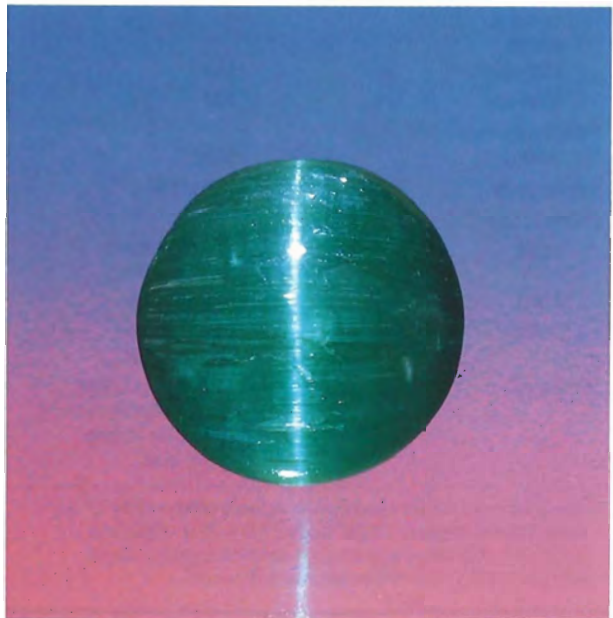
Figure 14. Densely packed acicular growth tubes produced chatoyancy in this 0.95-ct green tanzanite. Photo by Shane F. McClure.
