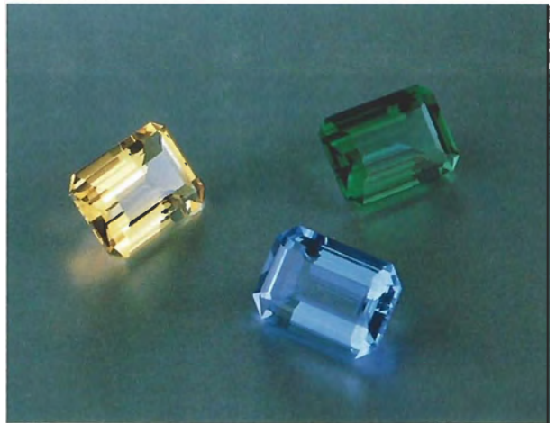
Figure 15. These Russian-grown hydrothermal synthetic quartzes (left to right: 6.18, 6.42, and 6.20 ct) are representative of some of the faceted material now available. Photo by Maha Smith.
