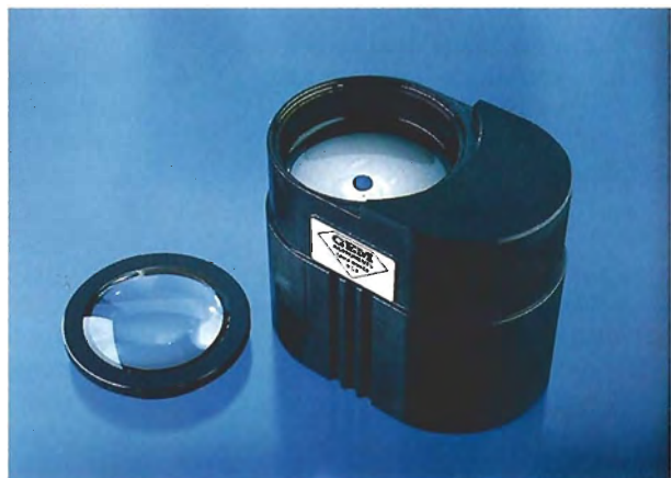
Figure 19. GIA GEM Instruments' new portable Illuminated Immersion Cell is designed to detect diffusion treatment. Photo by Maha Smith.
