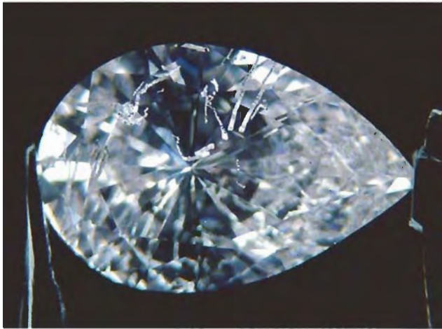
Figure 5. At first glance, there appear to be numerous laser drill holes in this 2.04-ct fancy light pink diamond. Magnified 10×.
