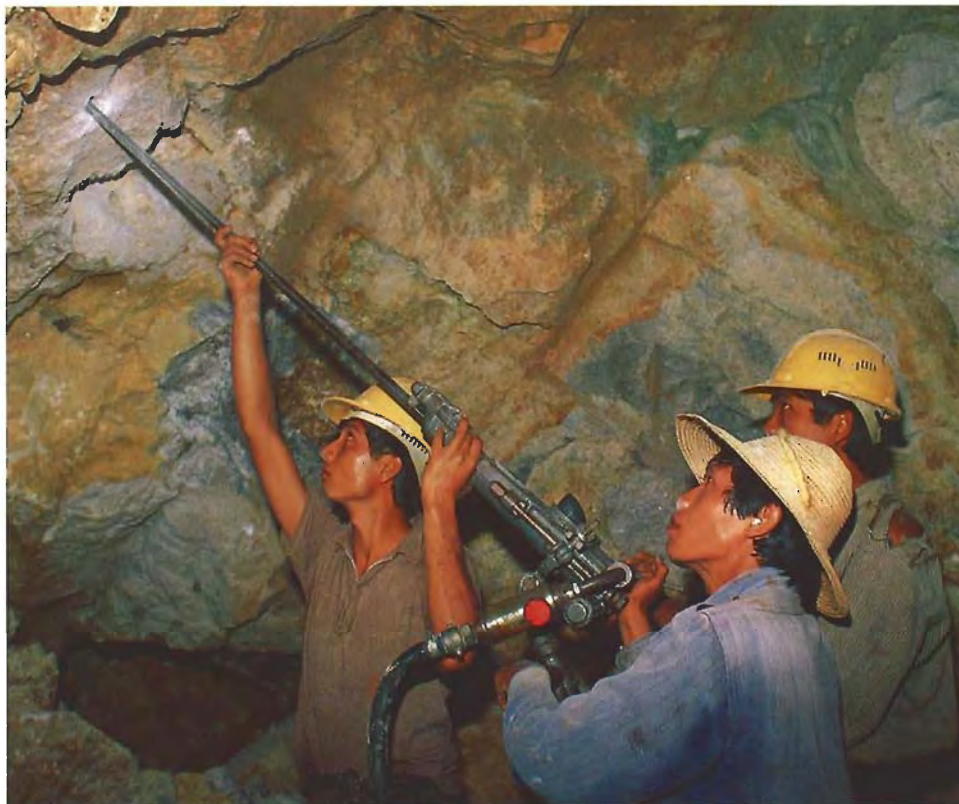
Figure 14. A major tunneling operation underway at the MGE Lin Yaung Chi mine involved the extensive use of explosives to reach the gem-bearing fault zone, that is, the primary occurrence of the gems. A jackhammer was used to drill holes, which were then packed with explosives, sealed with mud, and the fuse lit. Photo by Robert E. Kane.
