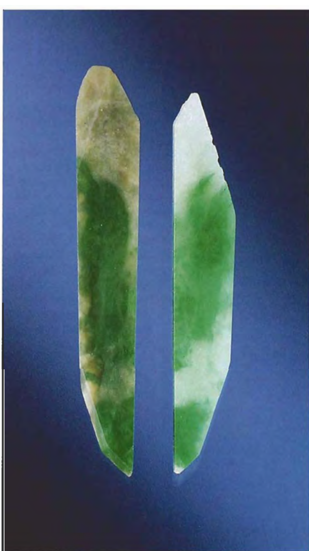
Figure 2. These two jadeite pieces, which weigh 10.32 and 7.69 ct, illustrate the effectiveness of the treatment discussed in this article. They represent two halves of the same sample, one before treatment (left) and the other after bleaching and polymer impregnation (right). Photo © GIA and Tino Hammid.
