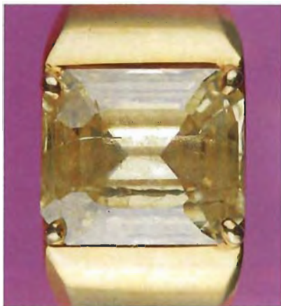
Figure 3. A large fracture became noticeable on the table and pavilion of the "filled" 6.90-ct diamond in this ring after it had been inadvertently left in an ultrasonic cleaner for two hours. In some areas, the filling material had been removed; in others, it had shattered within the fracture.
