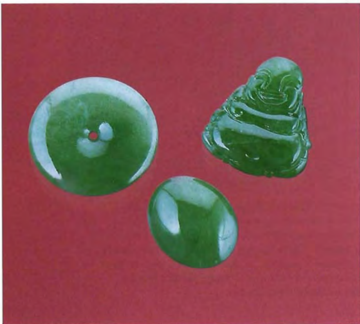
Figure 13. The use of a polymer other than one like Opticon was not evident in the visual appearance of these pieces. The spectrum shown at the top of figure 12 was taken from the carved Buddha; the other jadeites were all found to have been treated with a polymer that had a close spectral match to Opticon. Photo by Shane F. McClure.
