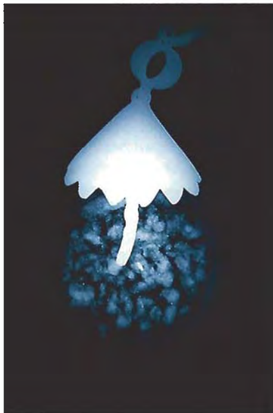
Figure 12. This X-radiograph shows not only that the baroque pearl in figure 10 is hollow, but also that it has been filled with some sort of composite material to anchor the post.
