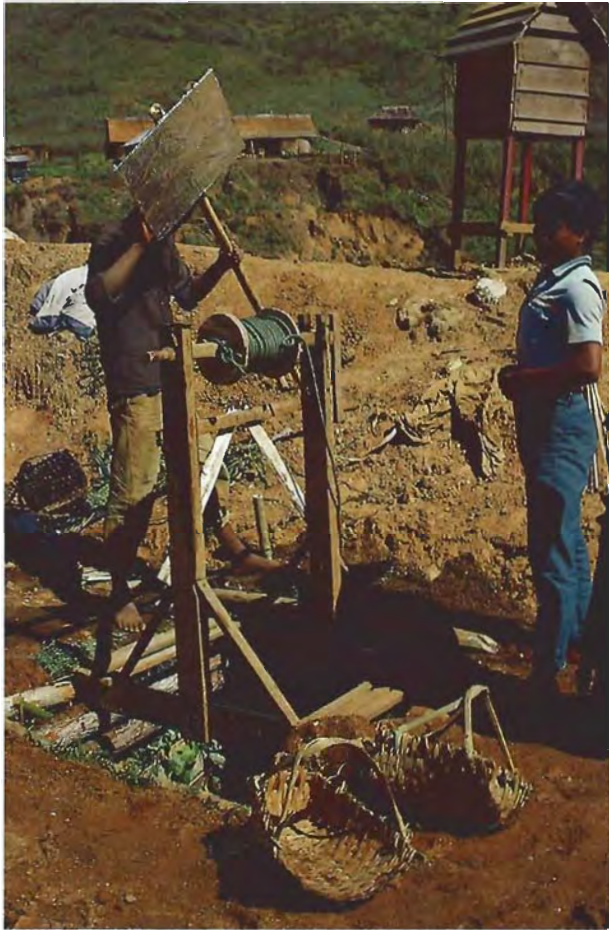
Figure 9. A variation of the classic twinlon mining method, a lebin is a square pit reinforced with timber and large leaves. Note the use of aluminum foil to reflect light into the mine and of a hand-cranked winch to hoist dirt and gem gravel to the surface in tightly woven bamboo buckets. Photo by Holly Kane.
