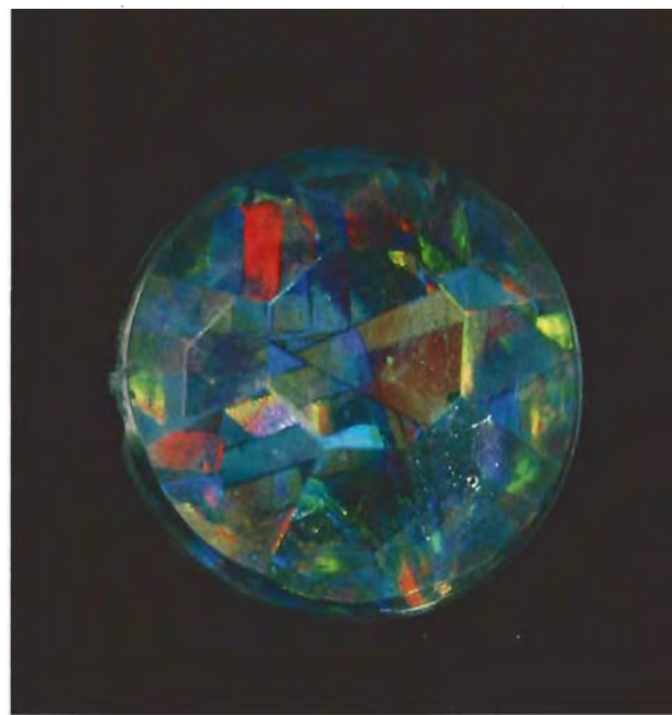
Figure 20. This imitation of crystal opal, approximately 12 mm in diameter, consists of a colorless plastic "gem" that has been backed with a patterned diffraction laminate. Photo by Maha Smith-DeMaggio.
