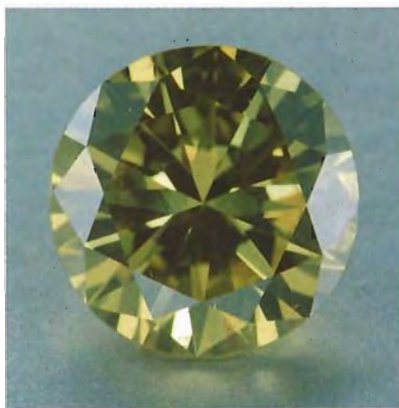
Figure 11. Because of the radionuclide responsible for the radioactivity in this 2.51-ct diamond, a legal (U.S.) release date of approximately 6507 A.D. was calculated.
