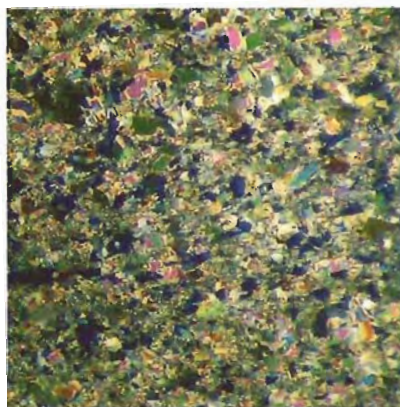
Figure 13. At least two different components can be seen in this thin section of the lapis lazuli imitation illustrated in the Spring 1992 Lab Notes section (p. 55) when it is viewed between crossed polarizers. Magnified 80 \times .
