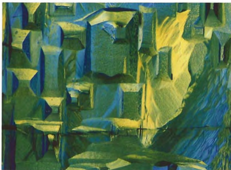
Figure 8. The surface texture on the prism face of this Luumäki yellow beryl crystal is typical of the material found at this locality. Prolonged natural etching has produced the stepped, mosaic-like surface features, with etch pits and hillocks. Photomicrograph by Kari A. Kinnunen; transmitted Rheinberg illumination (blue/yellow dual-circular filter to enhance the three-dimensional effect) and shadowing; magnified 8 \times .
