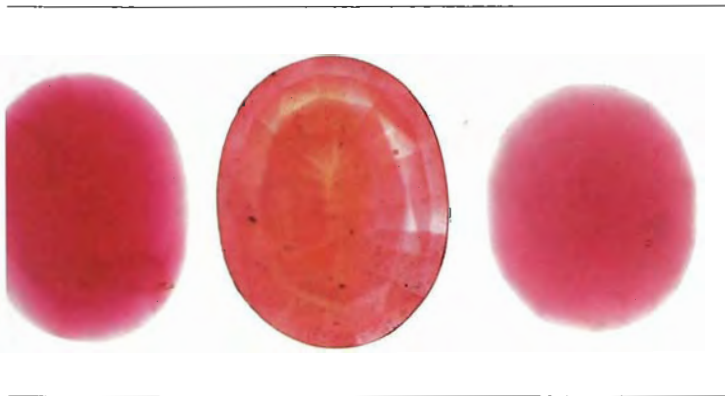
Figure 17. With immersion (here, in methylene iodide), the significantly greater relief of the diffusion-treated stone (center) as compared to synthetic (left) and natural (right) ruby is readily apparent. Photo by Shane F. McClure
