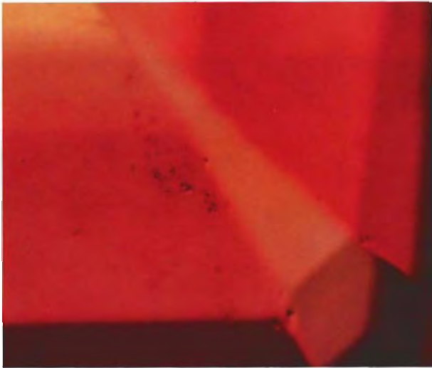
Figure 8. In general, the predominantly pink-to-red-to-purple diffusion-treated stones showed more areas that were totally devoid of diffused color than have been noted in blue diffusion-treated stones. Photomicrograph by Shane F. McClure; magnified 28 \times .
