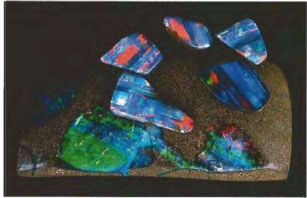
Figure 4. Just as it precipitated throughout the Winton formation, opal can be seen here filling cracks and voids in the host ironstone. Specimen is approximately 75 mm × 28 mm wide. Photo by Rudy Weber; © Australian Opal and Gemstone Photographic Library.
