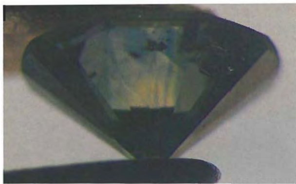
Figure 3. The arrangement of darker blue, lighter yellow, and near-colorless internal growth sectors in sample 2 is seen here with diffused light. The small opaque areas represent metallic flux inclusions. The arrangement of internal growth sectors is less obvious in the other two faceted stones. Photomicrograph by John I. Koivula.
