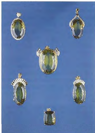
Figure 4. The uniformity of color, and the fact that the optic axes of all six yellow-green beryls (12–35 ct) are perpendicular to the table, suggests that all may have been cut from the same piece of rough.
