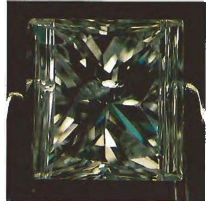
Figure 8. Large grooves have been cut into the pavilion of this 0.27-ct diamond, apparently so it could be used in an "invisible" setting. Magnified 10×.
