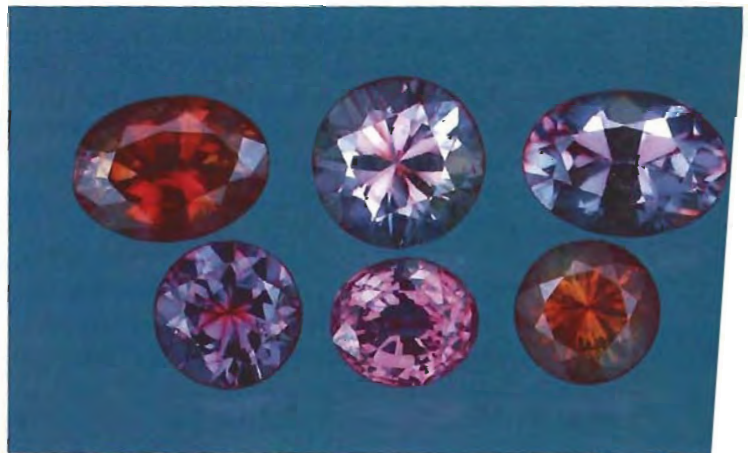
Figure 3. These stones, ranging from 0.55 to 3.35 ct, represent some of the less successful results of early experimentation to produce pink-to-red diffused color in corundum. Photo by Shane F. McClure.
