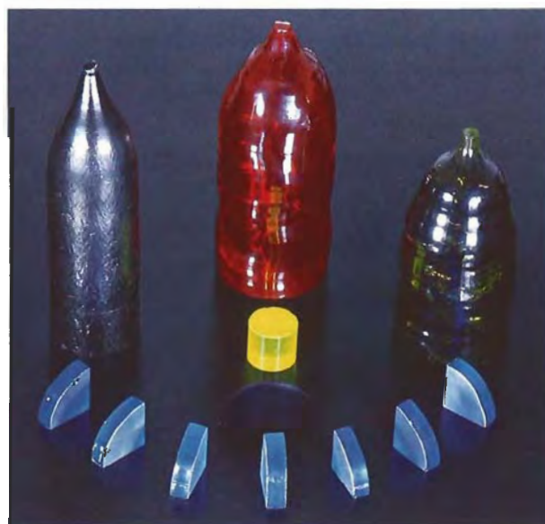
Figure 23. Crystal-pulling techniques are being used increasingly to produce materials with gem applications, such as these specimens of synthetic corundum (e.g., the red boule, 18 cm long × 7.5 cm in diameter) and YAG (e.g., the blue wedges, 2.8 cm long × 1 cm thick). Courtesy of Manning International; photo by Nicholas DelRe.
