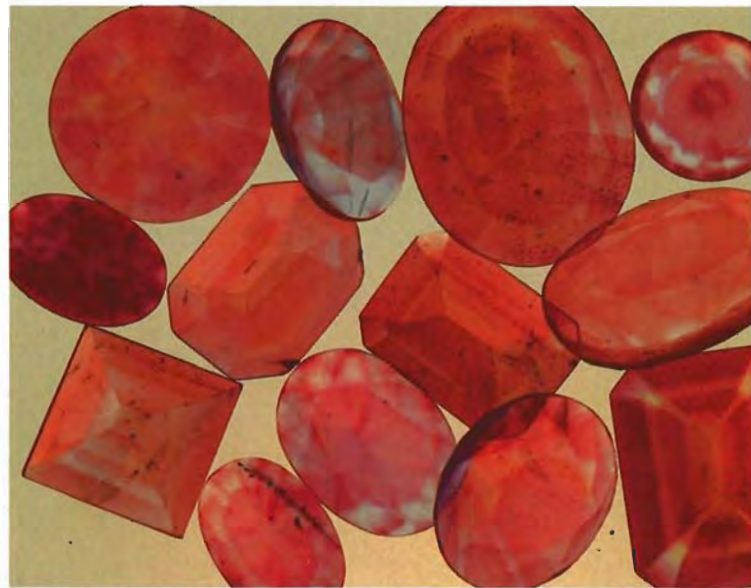
Figure 15. The uneven distribution of diffused color in many of the test stones was easily seen when immersion (here, in methylene iodide) was used in conjunction with diffused transmitted light. Photo by Shane F. McClure.
