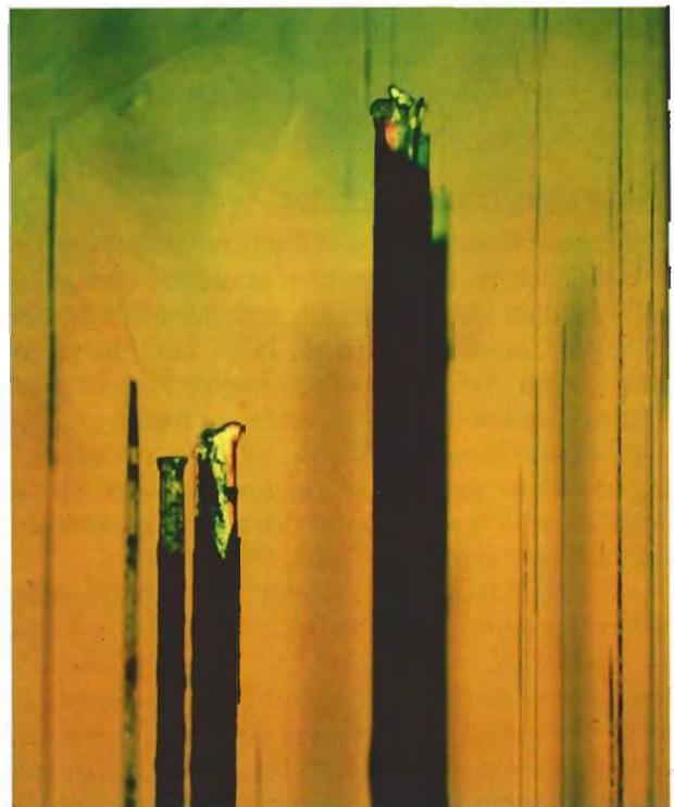
Figure 10. Growth tubes parallel to the c-axis were found to be characteristic of Luumäki beryl. Small syngenetic mineral inclusions (albite) can be seen here in the ends of the needles. Photomicrograph by Kari A. Kinnunen; transmitted crossed polarized light, magnified 20 \times .
