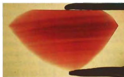
Figure 2. Slightly curved color banding, typical of a melt-grown synthetic, was detected in this 3.59-ct synthetic alexandrite with magnification and immersion in methylene iodide. Magnified 15x.
