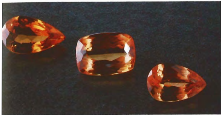
Figure 16. These flame-fusion synthetic corundums, 4.55–6.87 ct, have been fashioned for use as Imperial topaz simulants. Courtesy of L. P. Gems; photo by Maha DeMaggio.
