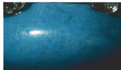
Figure 14. This odontolite cabochon shows the parallel banding frequently seen in this material. Magnified 17x.
