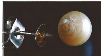
Figure 17. Note the relationship of the eroded area on this 7-mm cultured pearl to the area protected by the earring cup.
