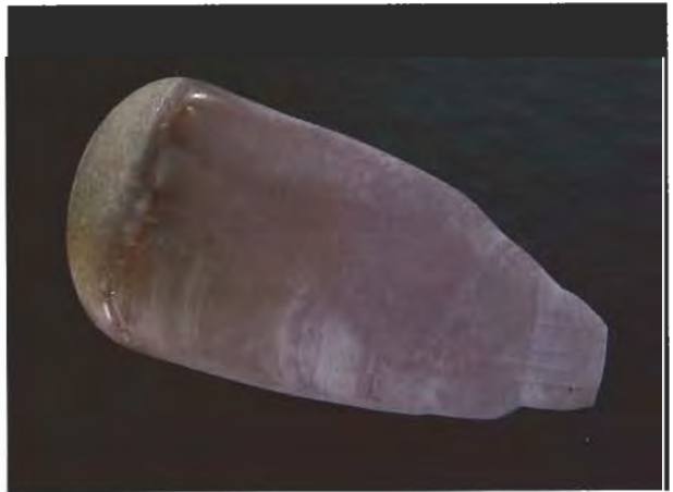
Figure 24. This 84.5-ct synthetic spinel boule was produced in the former German Democratic Republic to help satisfy internal demand for inexpensive gem materials. Photo by Maha DeMaggio.
