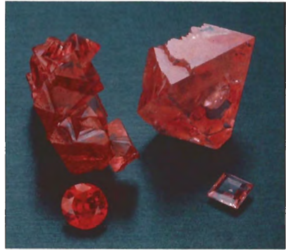
Figure B-1. These flux synthetic gahnites (0.47–23.25 ct) were grown on an experimental basis at Bell Laboratories. Courtesy of Dr. Kurt Nassau; photo by Robert Weldon.
