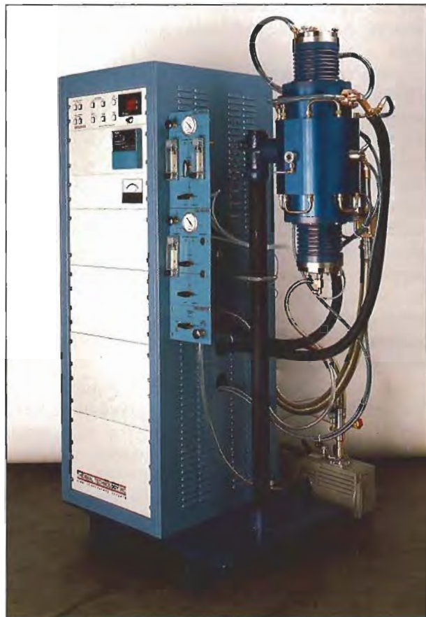
Figure 8. The Crystal Research heat-treatment experiments were conducted using a Thermal Technology Group 1000A graphite hot zone furnaces identical to this one. The cylindrical device to the right is the furnace itself. The furnace body, muffle tube extensions, and end plates are water cooled, which is why this 2200°C-capable furnace is so compact. The equipment rack to the left contains a 20-kw power supply, a programmable temperature controller, and the gas flow controls. Photo courtesy of Thermal Technology, Inc.
