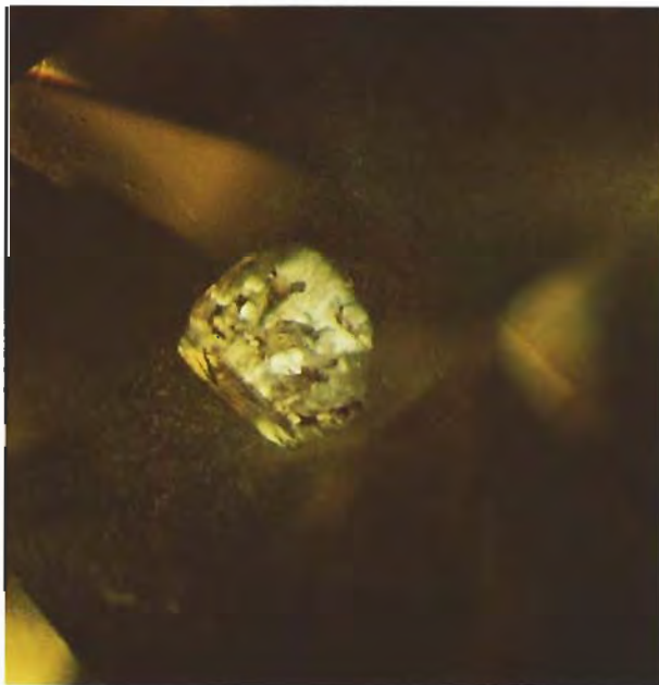
Figure 14. This large metallic inclusion, accompanied by numerous pinpoint inclusions, was seen beneath the table facet of HPHT-treated sample 21475 (see also figure 5). Note the rectangular area marked by graining; the border of this rectangular area is outlined by sectors that luminesce green to visible light. Photomicrograph by John I. Koivula; magnified 35 \times .
