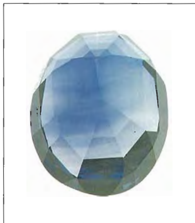
Figure 14. When the stone in figure 13 was removed from its mounting, immersion revealed the angular nature of the color zones.
