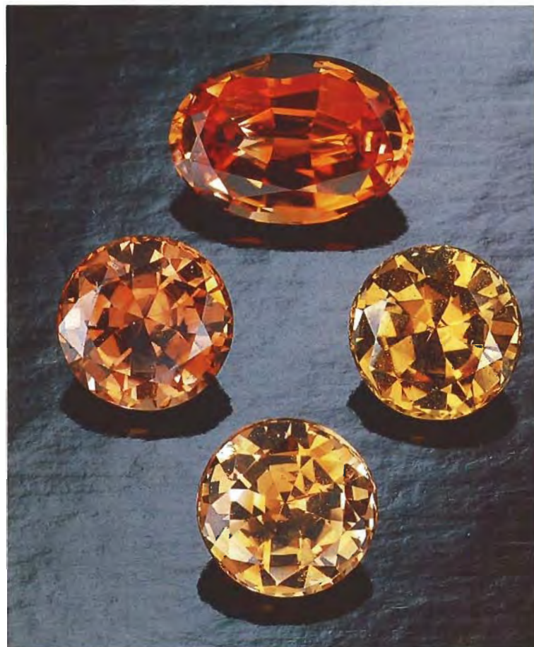
Figure 16. When yellow coloration from heat treatment like that used on the stones in figure 14 is induced in pale pink stones that contain a low concentration of chromium, this range of colors is produced. While the percentage of pale pink stones from the deposit that can achieve these colors is not high, the number of stones is still very large. Photo © GIA and Tino Hammid.
