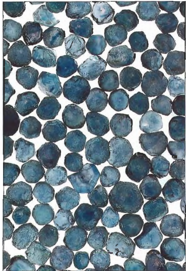
Figure 22. These rough blue sapphires were produced by heat treating the pale material shown in figure 7. The wide range of color saturation mirrors the wide range of rutile concentration. The yield of the material shown here from the near-colorless, pale blue, and pale green material of figure 7 is 50%. Photo © John L. Emmett.
