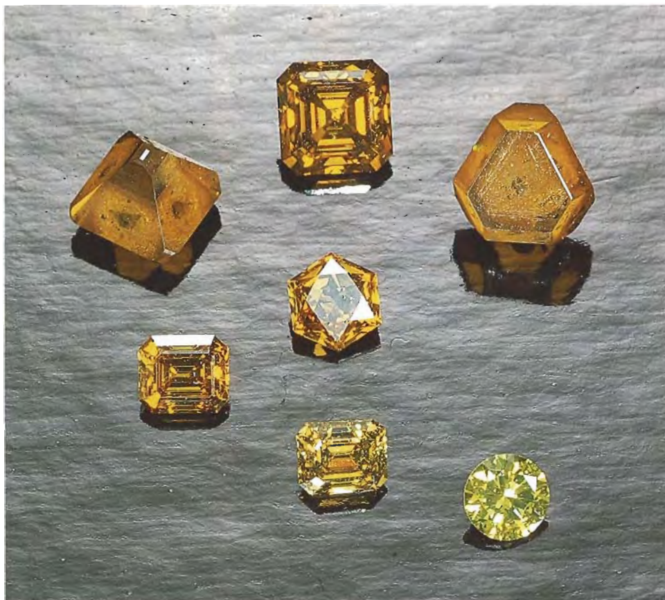
Figure 1. These synthetic diamonds—two as-grown crystals (0.78 and 0.88 ct), three as-grown faceted stones (0.18–0.51 ct), and two faceted stones treated at high pressure and temperature (0.14–0.21 ct)—were manufactured in Novosibirsk, Russia. They represent the core sample of this study. Photo by Robert Weldon.
