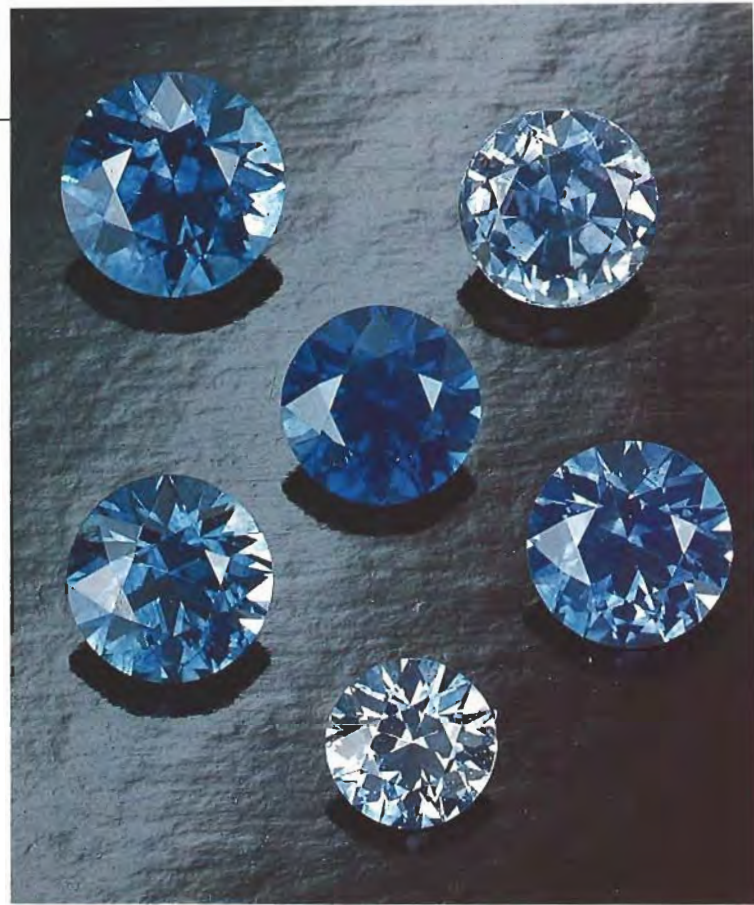
Figure 23. The faceted blue sapphires pictured are cut from material like that shown in figure 22. These stones are representative of the color range and clarity that is produced by heat treating the pale green and blue stones shown in figure 7. Photo © GIA and Tino Hammid.
