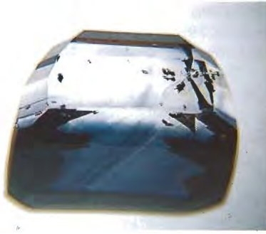
Figure 12. A side view of the stone in figure 11 reveals that the color is confined to a thin layer under the table. Magnified 10 \times .
