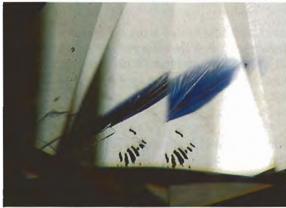
Figure A-3. Also unlike most other Koss-filled diamonds examined as part of this study, the brightfield flash colors in this group of stones (which were sent directly to Koss for treatment) were blue and violet. Photomicrograph by Shane F. McClure; magnified 33 \times .
