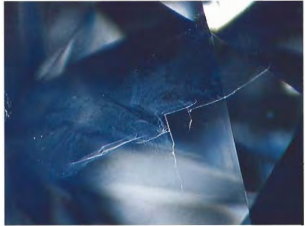
Figure 21. Cloudy areas within the filler were a common feature in Goldman Oved-treated diamonds. Photomicrograph by Shane F. McClure; magnified 40x.
