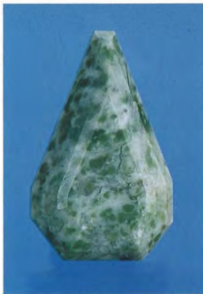
Figure 4. This 47.31-ct cut-cornered, faceted triangle is a rock composed primarily of white grossular garnet and green diopside.
