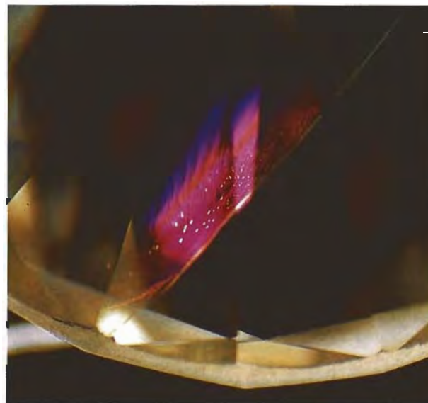
Figure 4. Many of the recent Yehuda-treated diamonds display more than one vivid flash-effect color at a single viewing angle. The most predominant colors seen with darkfield illumination in recently treated stones are pink, violet, and purple. Photomicrograph by Shane F. McClure; magnified 28x.
