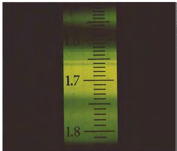
Figure 13. Atypical “satellite readings” can be seen on the refractometer scale when the table facet of an unusual 8.79-ct tourmaline is tested. Photo by Maha DeMaggio.
