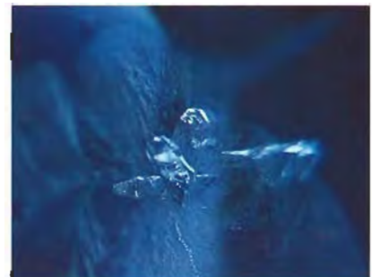
Figure 15. When the same sapphire was cooled cryogenically and reexamined at 63 \times magnification, it became clear that the "crystals" are actually negative crystals with two-phase CO 2 inclusions.
