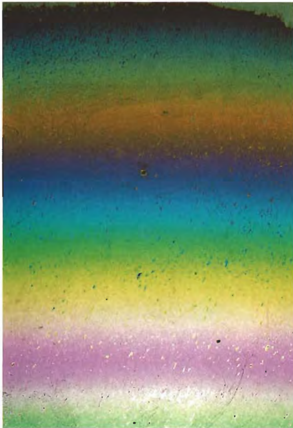
Figure 37. The interference spectrum can be seen by looking at a quartz wedge between crossed polarizers. The dark-gray color occurs where the interference film is the thinnest; colors vary to yellow, blue, red, yellow again, etc., and finally to repeated pinks and greens, as the film gets thicker. Compare this with the iridescent fracture in figure 35. Photomicrograph by John I. Koivula.
