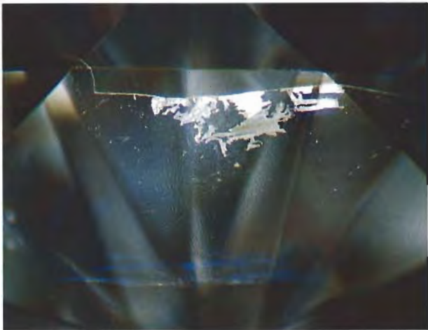
Figure 12. A fine, transparent flow structure was detected in several of the Goldman Oved-filled diamonds examined for this study. Photomicrograph by Shane F. McClure; magnified 40 \times .
