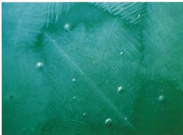
Figure 12. Magnification reveals gas bubbles and fibrous inclusions in the specimen shown in figure 11. Photomicrograph by Maha DeMaggio; magnified 40x.
