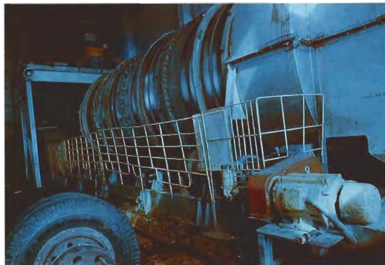
Figure 9. Disaggregation of the emerald-bearing rocks at the Malysheva processing plant is accomplished in a rotating drum, or scrubber.
