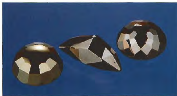
Figure 16. "Platigem," a platinum-aluminum-copper intermetallic compound, comes in a subtle range of colors. These stones weigh, from left, 12.63, 10.52, and 11.63 ct. Photo by Maha DeMaggio.
