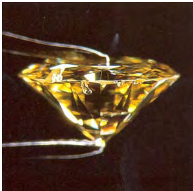
Figure 6. Damage to the diamond in figure 5 is related to the combination of a thin girdle and shallow crown angles, as can be seen in this profile view.
