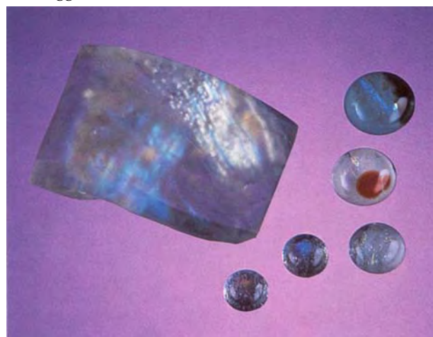
Figure 24. These cabochons of dichroic glass could be mistaken for opals. The large free-form piece, by Susan Slayton, measures 34.38 × 24.24 × 10.61 mm and weighs 64.82 ct; the round cabochons, by Nancy Goodenough, range from 1.30 to 4.40 ct (the largest is 10.4 mm in diameter). Photo by Maha DeMaggio.
