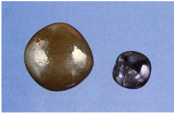
Figure 2. These 1.66 and 0.28 ct diamond "pearls" were polished by selective dissolution in hot sodium carbonate. The larger "pearl" measures about 5.76 × 5.58 mm. Photo by Maha DeMaggio.
