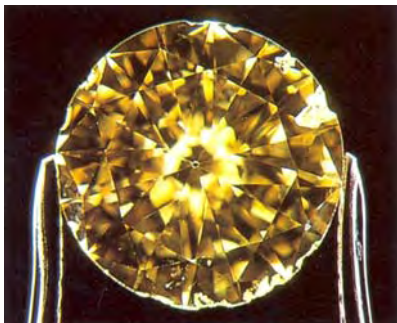
Figure 5. Many chips can be seen on the girdle of this 2.66 ct round-brilliant-cut diamond, which was originally set in a four-prong lady's ring.
