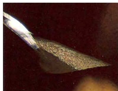
Figure 2. An etched feather can be seen in the pavilion of the Kelsey Lake diamond shown in figure 1. Magnified 57x.
