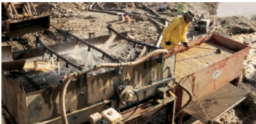
Figure 17. At the Benitoite Gem mine, material is fed first into a layered screening apparatus fitted with high-pressure water jets, and then into a gravitational separation jig. Pieces over 25 mm are separated by the screening apparatus and checked for specimen potential, while material between 3 and 25 mm is washed into the jig where the heavier benitoite is trapped in several parallel trays. Photo by Brendan M. Laurs.
