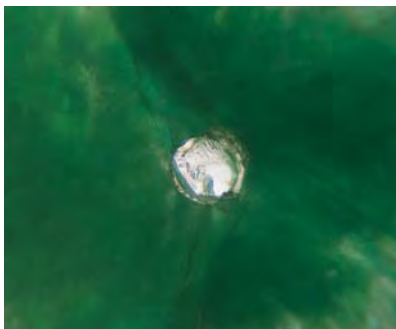
Figure 8. Excess polymer is visible in this hole drilled in the carving shown in figure 7. Magnified 20x.
