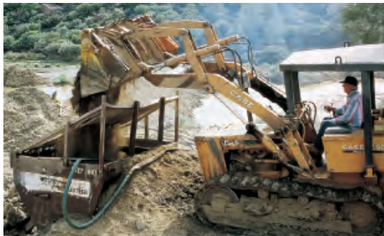
Figure 16. The mine owners at the Benitoite Gem mine process colluvial and alluvial material using mechanized equipment. Here a loader dumps material through a grizzly and into a hopper. Rocks larger than 15 cm roll off the grizzly and are examined individually; stones smaller than 15 cm are washed down a chute to the apparatus pictured in figure 17. Photo by Brendan M. Laurs.
