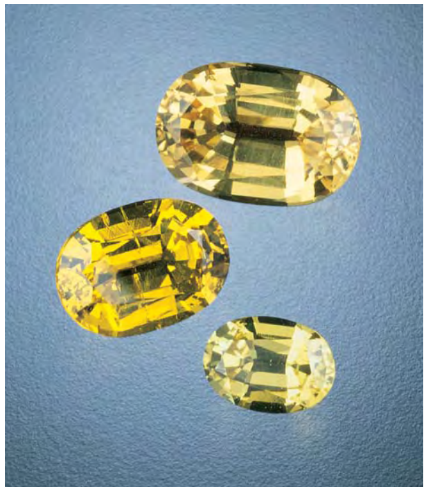
Figure 10. Yellow Tairus hydrothermal synthetic sapphires are colored predominantly by \text{Ni}^{3+} . Photo © GIA and Tino Hammid.
