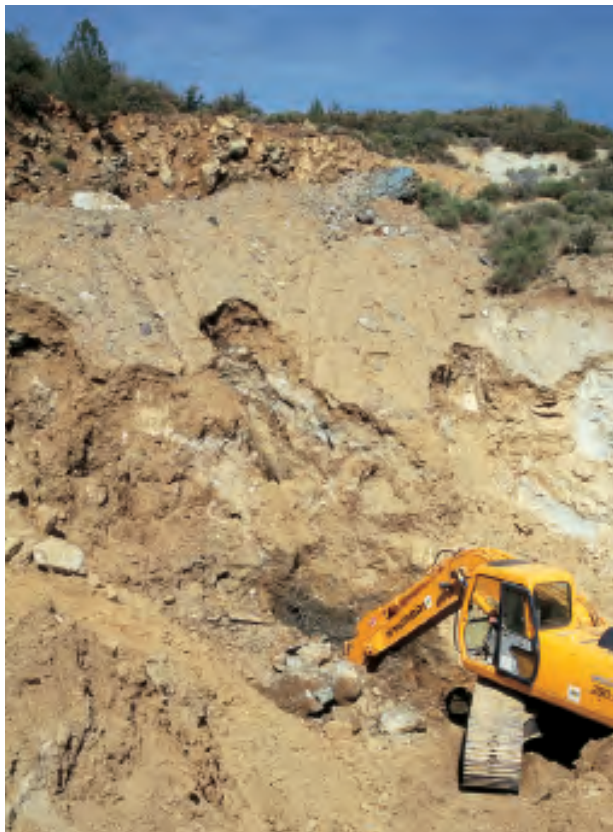
Figure 20. The backhoe is excavating the newly discovered western extension of the deposit at the Benitoite Gem mine. Boulders of altered blueschist, some bearing benitoite, are piled near the left rim of the pit. The high wall of the main pit can be seen on the skyline. Photo by Brendan M. Laurs.
