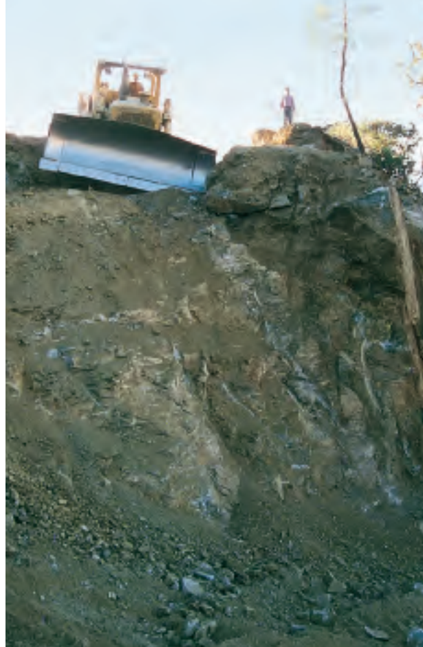
Figure 12. The Junnila claim was excavated with heavy equipment in 1995. Benitoite was recovered from the narrow, vertical zone of resistant blueschist that is visible here beneath the slender pine tree. Photo by William Larson.
