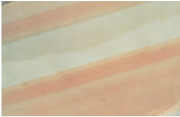
Figure 5. Prominent light to dark pink bands are visible in this faceted synthetic pink quartz. The color banding parallels the orientation of the colorless seed plate in the center. Photomicrograph by Shane F. McClure; immersed, diffused light, magnified 11 \times .
