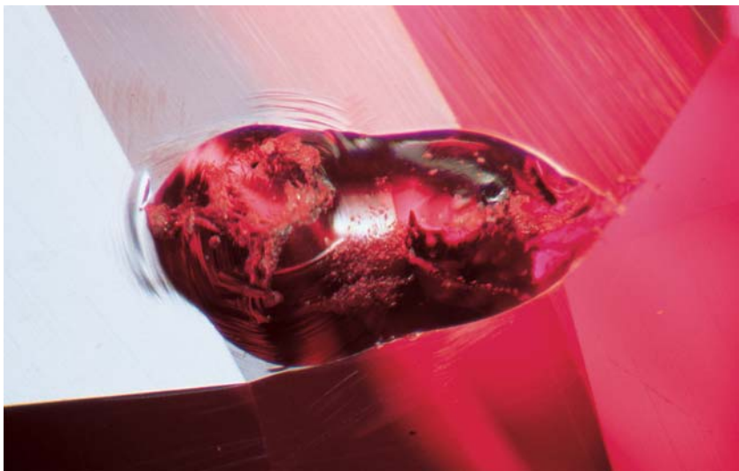
Figure 7. A rotary tool was used to partially repolish this 2.6-mm-long pit in the surface of a ruby, probably to remove evidence of heat treatment. Notice the curved grooves made by the tool in the faceted surfaces near the edge of the pit.
