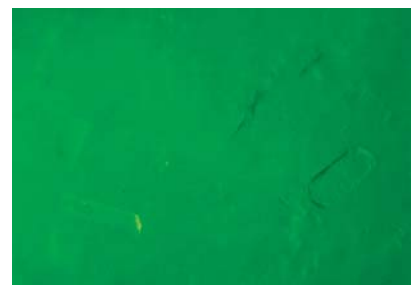
Figure 4. Raman microanalysis of the two largest included crystals in this jadeite cabochon showed that they were zircon. Magnified 15x.
