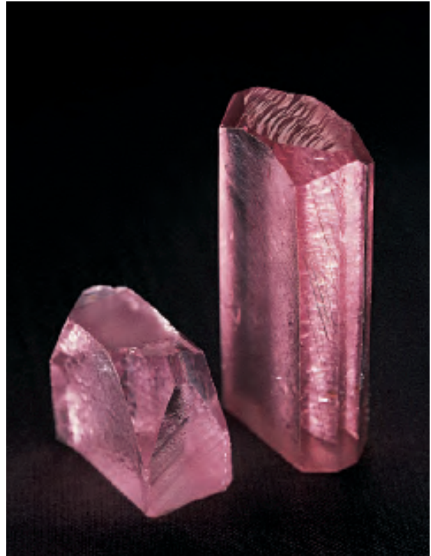
Figure 16. These two samples of synthetic pink quartz are shown here three years after they were irradiated, at which time they were both the same color. However, the crystal on the right (52 mm long \times 10 mm thick) was kept in the dark for the three years, whereas the crystal segment on the left (23 mm long and 12 mm thick) was one of several that were exposed to sunlight throughout this period. The fact that there is very little difference in color between the two samples indicates that the color appears to be stable over time. Photo by Mikhail A. Bogomolov.
