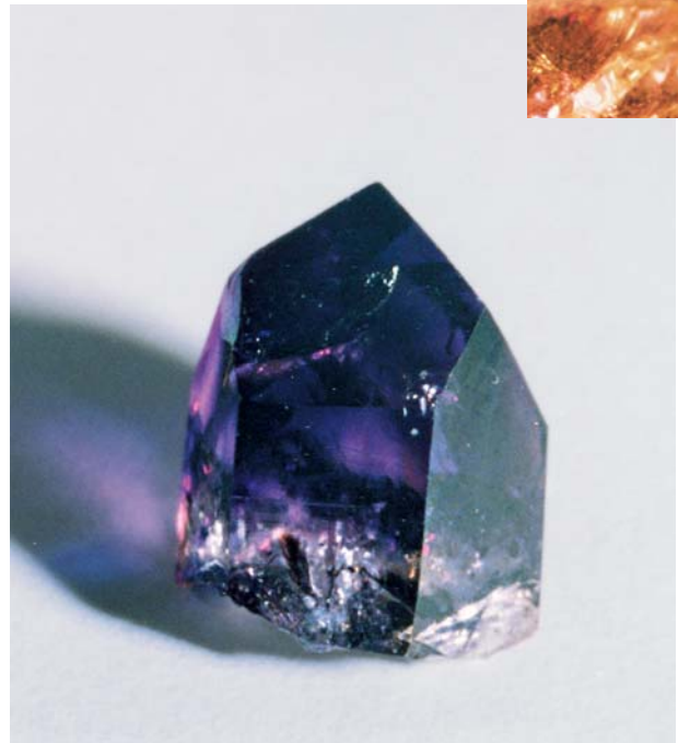
Figure 11. The shape of this approximately 1 cm wide synthetic amethyst crystal, one of several examined recently in China, resembles that of a natural crystal. Because these crystals are grown on dome-shaped seeds, there was no obvious seed plane. Inset: These “nail-head” inclusions extend from the curved seed into the synthetic amethyst. Macro photo by Zhang Tao, NGTC; photomicrograph by Shen Meidong, magnified 25x.
