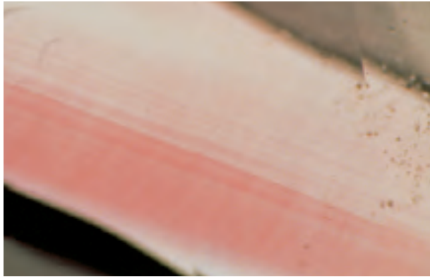
Figure 9. Faint stream-like structure lines are oriented perpendicular to the prominent color bands in this 7.63 ct faceted natural pink quartz from Brazil. Photomicrograph by Shane F. McClure; magnified 16 \times .
