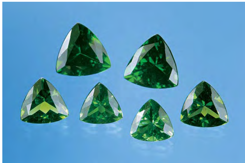
Figure 7. These six modified triangular brilliants (2.05–4.93 ct) were represented as natural “green obsidian,” but they proved to be manufactured glass.
