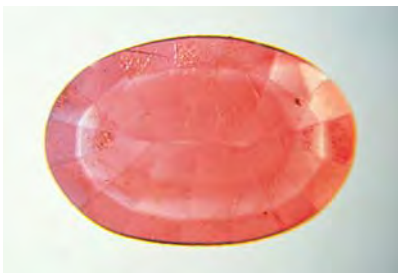
Figure 2. When immersed in methylene iodide and placed over diffused transmitted light, this 0.69 ct oval mixed-cut corundum showed both the color concentrations on facet junctions and the spots devoid of color that indicate that it was colored by diffusion treatment.
