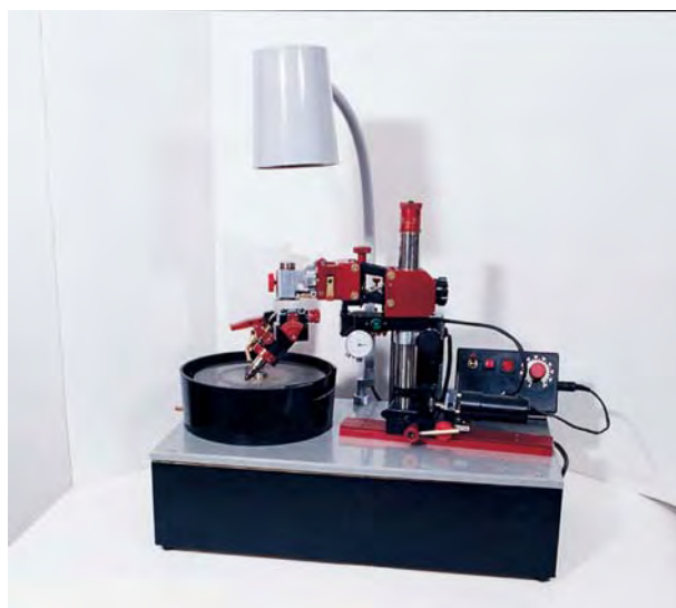
Figure 22. This new faceting machine, Imperial Gem Instruments' "Diamante," can be used to perform all steps in faceting both diamonds and colored stones. Photo by Nick Michailidis.
