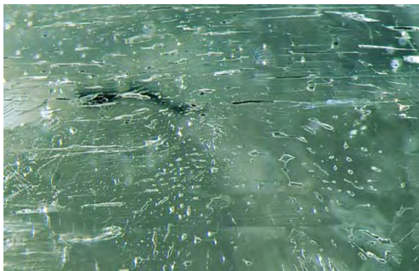
Figure 16. Fluid and two-phase (fluid and gas) inclusions such as these were seen in a topaz from Klein Spitzkoppe. Photo © Bruce Cairncross; magnified 24x.
