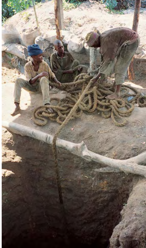
Figure 23. These Tanzanian miners are using a rudimentary rope-and-bucket system to remove dirt and debris from the flooded mine shaft. Photo by Jeff Schneider.
