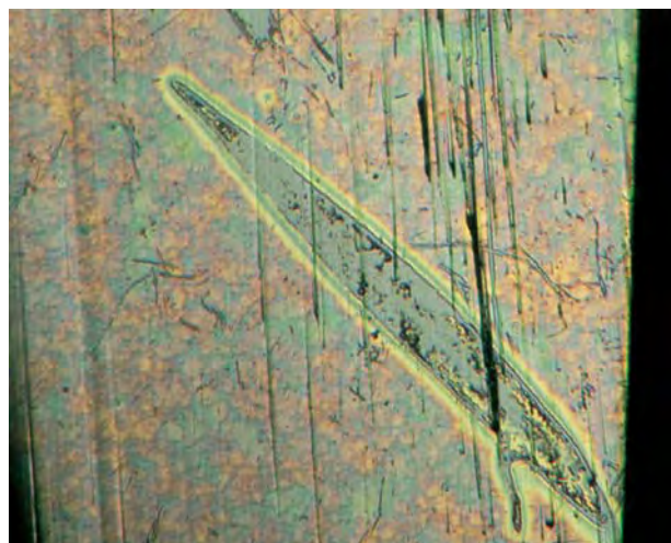
Figure 18. The pink surface coating on this topaz was easily scratched with a pin, as seen here in reflected light. Photomicrograph by Shane F. McClure; magnified 23 \times .
