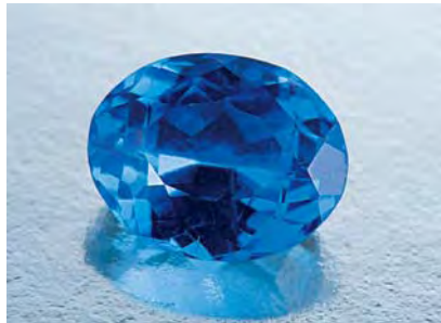
Figure 2. Before exposure to light, this 3.34 ct oval Maxixe-type beryl was dark blue (left). Eight hours of exposure in a solar simulator caused this stone to fade considerably (right). The faded color is both less saturated and lighter in tone than the original, resulting in an appearance that is both paler and grayer.
