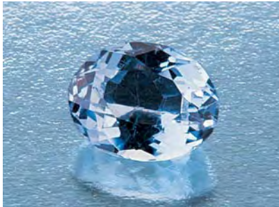
Figure 2. Before exposure to light, this 3.34 ct oval Maxixe-type beryl was dark blue (left). Eight hours of exposure in a solar simulator caused this stone to fade considerably (right). The faded color is both less saturated and lighter in tone than the original, resulting in an appearance that is both paler and grayer.
