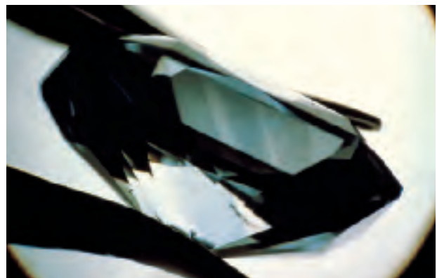
Figure 13. Color zoning is often observed in blue diamonds. This photograph, taken at 10 \times magnification, shows parallel banding of colorless and blue areas. The position of the zones can have a significant impact on the face-up color (but typically not the clarity) of the diamond. Photo by Stephen Hofer, © GIA.
