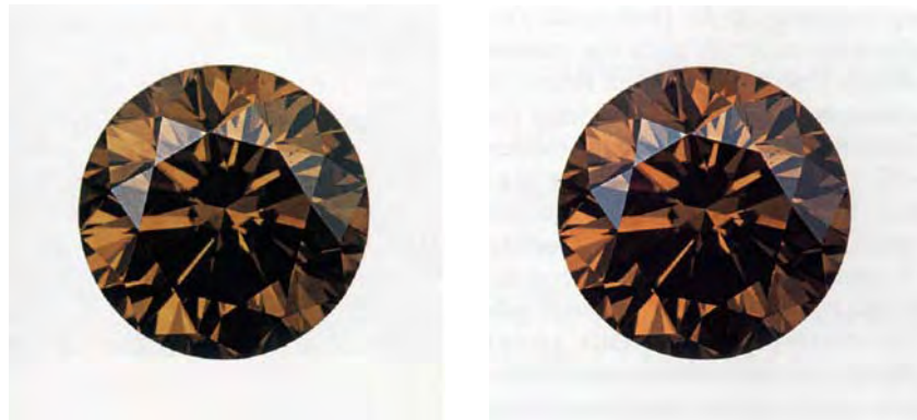
Figure 6. Beneath the overall brown color, this 0.51 ct synthetic diamond shows a color change from a greenish yellow hue in daylight (left) to an orange hue in incandescent light (right).
