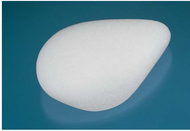
Figure 23. This 99.90 ct free-form promoted as “cultured snow quartz” is actually fused silica glass with a high density of gas bubbles. It makes a convincing imitation of quartzite. Photo by Maha DeMaggio.
