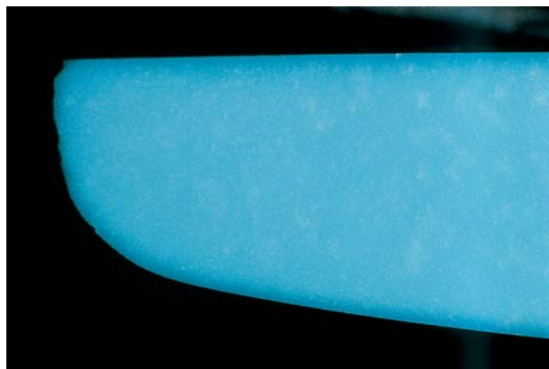
Figure 6. This cross section of a cabochon that was surface treated to improve color shows a narrow rim of more saturated color. The depth of this rim ranged from 0.2 to 0.5 mm in the samples we examined. Photomicrograph by Shane F. McClure; magnified 14 \times .
