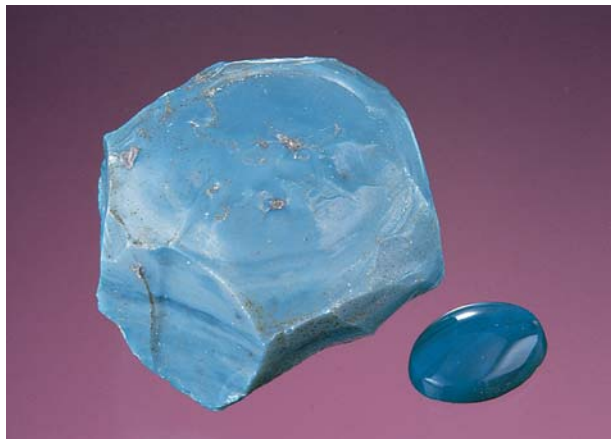
Figure 24. This 338.6 ct piece of rough and 8.92 ct cabochon are manufactured slag glass from central Sweden. Photo by Maha DeMaggio.
