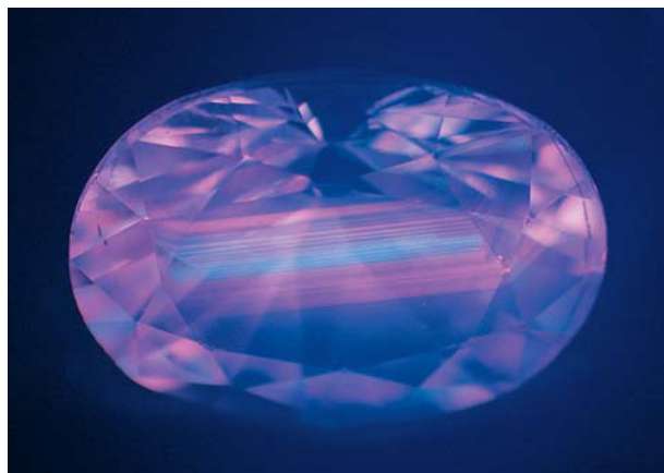
Figure 8. Although cathodoluminescence has been used to reveal the characteristic straight growth bands in this natural colorless sapphire, these bands often can be observed with long-wave UV radiation or immersion microscopy. Photomicrograph by Shane Elen; magnified 3.5x.
