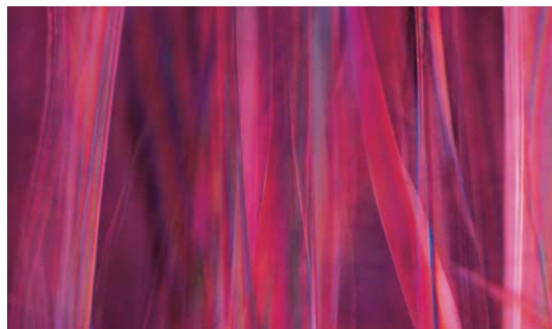
Figure 30. Colorful “Plato lines” are observed in the synthetic sapphire block when it is viewed down the optic-axis direction in cross-polarized light. Photomicrograph by John I. Koivula; magnified 10×.
