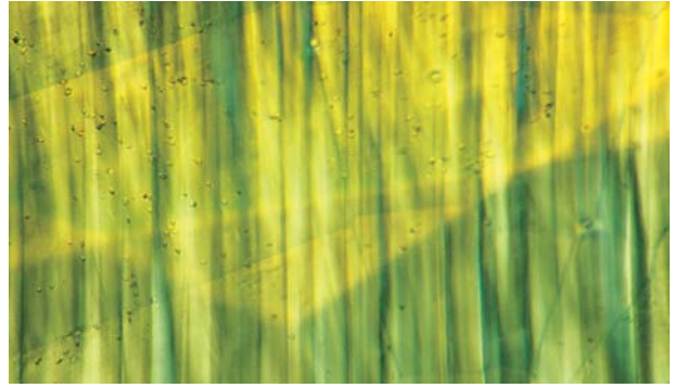
Figure 14. In this faceted blue-green synthetic sapphire, as in the synthetic ruby in figure 13, one can see striations representing oriented subgrain boundaries between the long, thin microcrystals. Immersion, crossed polarizers, magnified 70x.
