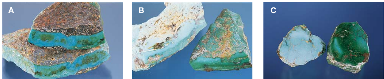
Figure 3. These samples (nos. 220–222a,b; 20–40 mm long) of rough “Emerald Valley” turquoise illustrate the results of treatment on different qualities of material. Half of each sample was treated by the Zachery process, and the other half was left untreated for comparison. Little change is visible in the treated half (top) of the high-quality (low-porosity) material in A. The medium-quality turquoise in B shows distinctly higher color saturation in the treated half (right sample), as does the low-quality material in C (also right). Photos by Maha DeMaggio.
