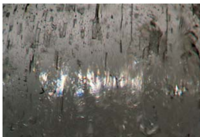
Figure 15. A group of parallel reflective planar inclusions with striations was responsible for the cat's-eye effect in this taaffeite. Magnified 30×.
