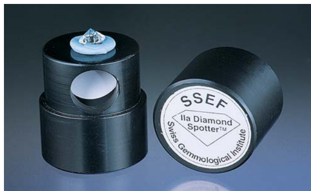
Figure 25. The SSEF Diamond Spotter (left, 4.0 × 2.8 cm diameter) is one of the newer instruments invented to help gemologists deal with some of the latest identification challenges. Even with the table down, the green fluorescence visible on the screen below the 1.08 ct diamond on the SSEF Diamond Spotter (right) indicates that the diamond is type IIa or IIb. Photos by Maha Tannous.
