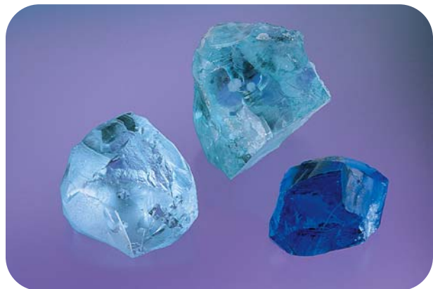
Figure 14. Natural aquamarine (left), glass imitation aquamarine (middle), and glass imitation tanzanite (right, 4 × 3 cm) are all easily separated by a dichroscope. Aquamarine, like tanzanite, will show the characteristic pleochroism of the natural gem, while the glass imitations will show no pleochroism. Photo by Maha Tannous.
