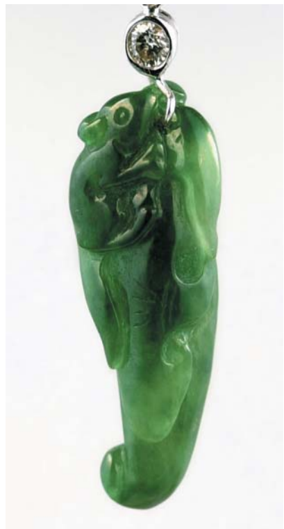
Figure 8. This attractive jadeite carving (37.48 × 15.19 × 11.85 mm) was dyed, impregnated, and assembled.
