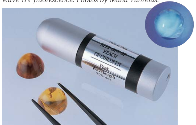
Figure 12. The lipstick-size (5.5 × 1.5 cm) long-wave portable ultraviolet lamp from Nebula, Redwood City, California, is one of the most durable UV lamps introduced in the last few years. Inset: Natural amber generally fluoresces blue under long-wave UV fluorescence. Photos by Maha Tannous.
