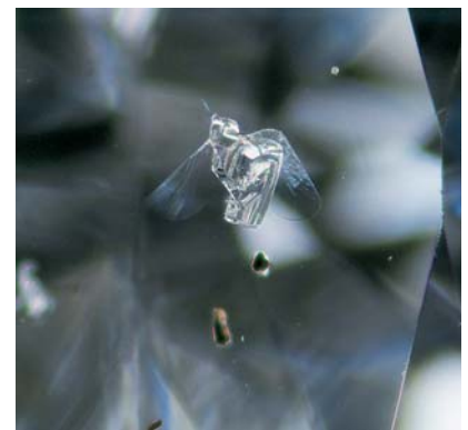
Figure 5. Although initially this large white feature appeared to be a crystal with feathers, it is actually a void that was created when a mineral inclusion was dissolved away. The reddish brown crystals near it were identified as chrome spinel by Raman analysis. Magnified 63×.
