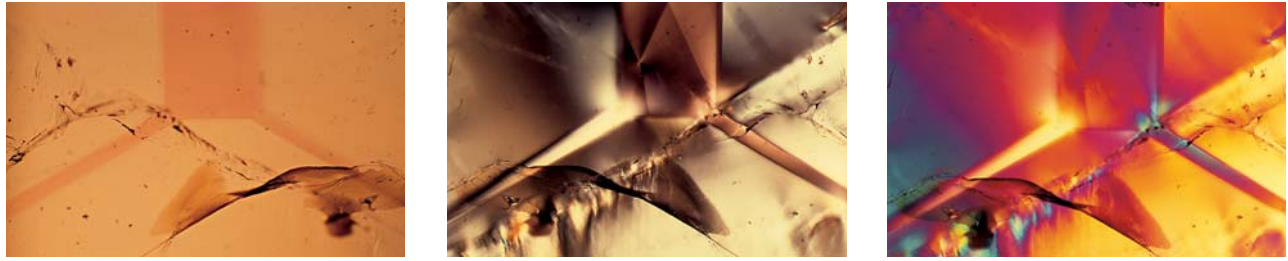
Figure 20. These images show strain patterns in a slice of liddicoatite from Madagascar cut perpendicular to the c-axis. The left view shows the color zoning, whereas the center and right photos were taken with cross-polarized light to show the anomalous birefringence; the image on the right was taken with a first-order red compensator. Although not one of the study samples, it has been confirmed as liddicoatite by electron microprobe analysis (J. Koivula, pers. comm., 2002). Photomicrographs by John I. Koivula; magnified 20×
