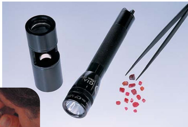
Figure 8. It is the author's opinion that the darkfield loupe, with the standard flashlight attachment, is the single most significant development in portable gemological instruments for the serious gemologist. Inset: In the absence of a darkfield loupe, the effect may be approximated with an oblique illumination technique that simply requires placing the gem material in question on the glass of the light source and covering the exposed portion with a finger to create a shadow effect while simultaneously securing the gem in place. Photo by Maha Tannous; inset by Jason Stephenson.
