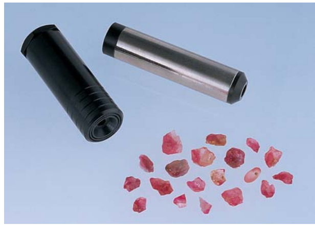
Figure 13. The OPL (Orwin Products, Ltd.) calcite dichroscope (left, 4.0 × 1.4 cm) is one of the smallest dichroscopes on the market. It is most useful with faceted gems under 10 ct. The OPL diffraction grating spectroscope (right, 5.5 × 1.3 cm) is the smallest and most portable spectroscope on the market. Mastering this instrument takes practice, but it can be one of the most important tools for the traveling gemologist. Photo by Maha Tannous.
