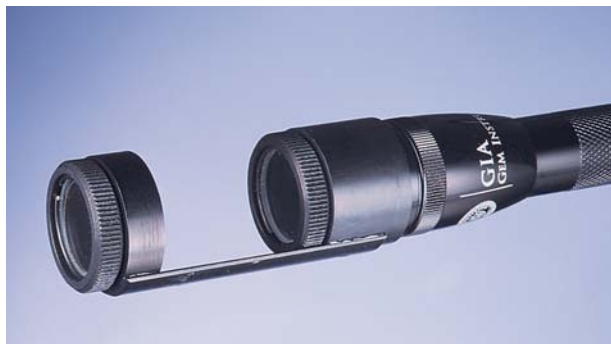
Figure 16. Attaching a polariscope to the end of a Mini Maglite provides an excellent portable tool for determining pleochroism and optic character. Photo by Maha Tannous.
