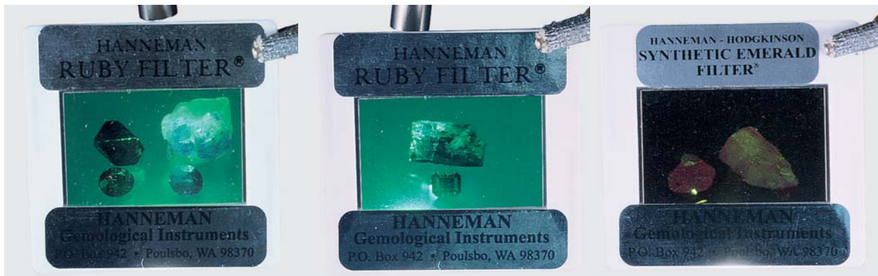
Figure 21. In the photo on the left, a faceted red spinel and a red spinel crystal both appear dark gray through the Hanneman Ruby Filter, whereas a faceted ruby and a ruby crystal on calcite matrix both appear blue through the same filter. In the center photo, a large red beryl crystal and faceted red beryl both appear grayish through the Hanneman Ruby Filter. On the far right, a faceted green YAG and a Chatham synthetic emerald crystal both appear pink when viewed through a Hanneman-Hodgkinson Synthetic Emerald filter. Photos by Maha Tannous.
