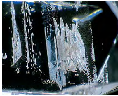
Figure 3. Large, white, irregular flux inclusions were present in both samples of synthetic bromellite examined for this study. Magnified 40x.
