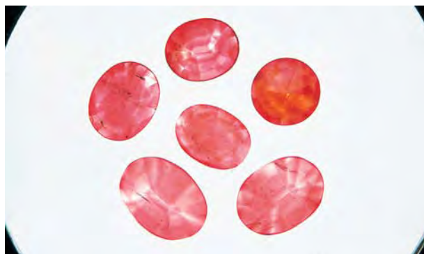
Figure 6. The uneven distribution of color was easily seen when the samples were immersed (here, in methylene iodide) and viewed with a diffused transmitted light source. Photo by Maha Tannous.
