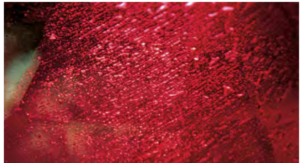
Figure 9. A high concentration of aligned inclusions occurred during the initial deposition of the synthetic overgrowth. As a result, these inclusions clearly demarcated the boundary between the host gemstone and the synthetic overgrowth. Magnified 22 \times .
