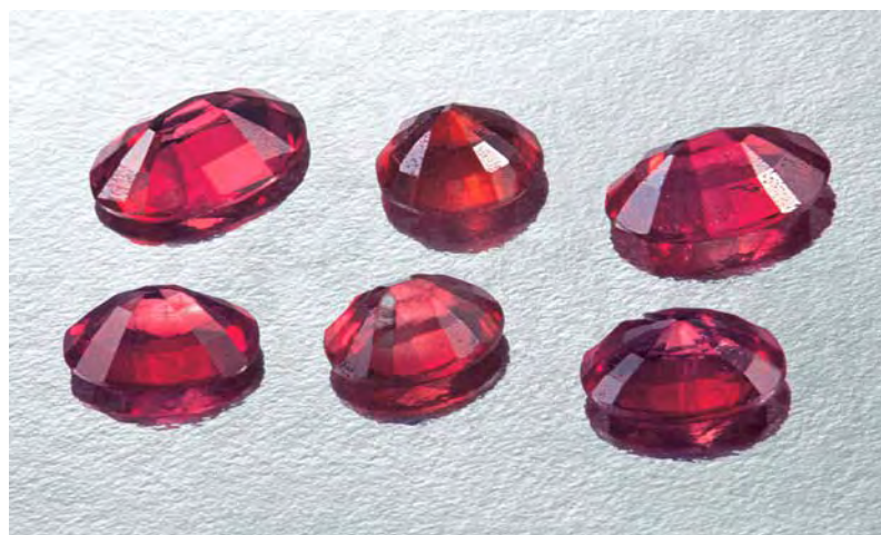
Figure 2. When viewed face down, most of the synthetic-overgrowth corundum samples readily showed uneven coloration between adjacent facets. The degree of visibility, however, was very dependent on the thickness of the overgrowth layer. Photo by Maha Tannous.
