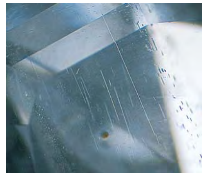
Figure 6. Numerous thin needles, which did not display any particular orientation within the stones, were seen in all the faceted bromellites and helped confirm their origin as natural. Magnified 29x.
