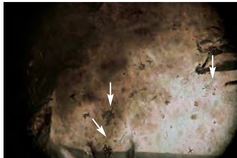
Figure 5. When this brown beryl was viewed parallel to the optic axis, skeletal ilmenite inclusions with brown halos could be seen (left; magnified 30×). Perpendicular to the optic axis, several thin, very dark brown lamellae were visible (right; magnified 40×). Photomicrographs by E. Fritsch.
