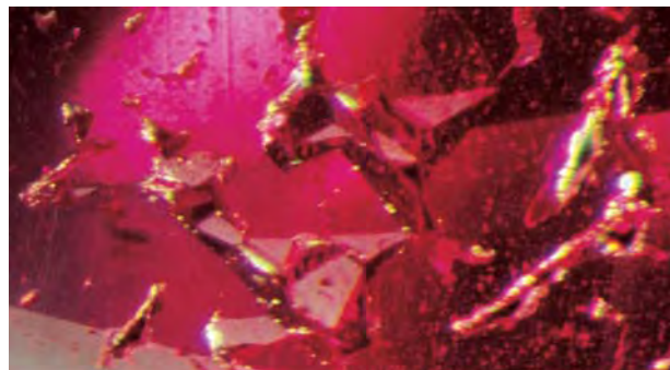
Figure 5. Many indentations or cavities at the surface of these stones extended the full depth of the overgrowth layer, down to but not beyond the boundary with the natural corundum. Typically, the walls of these indentations displayed a stepped morphology consistent with the formation of many small external crystal faces. Magnified 50 \times .
