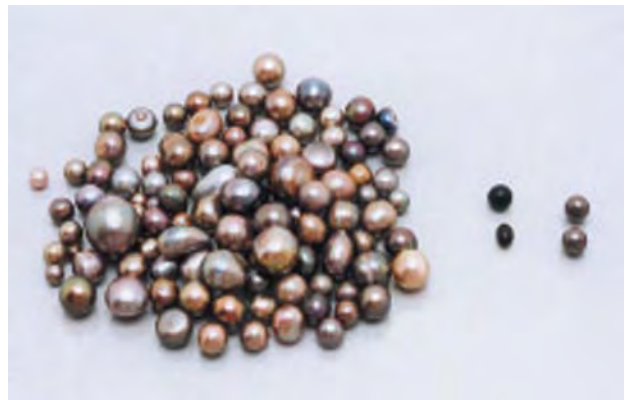
Figure 25. The samples on the left are representative of three parcels of natural pearls obtained by SSEF for identification last April. In one of the parcels were the two black samples in the middle (~3 mm each, which proved to be plastic imitations) and the two silvery gray spheres (4.75 mm each) on the right, which are made of steel. Photo by Michael S. Krzemnicki; © SSEF Swiss Gemmological Institute.
