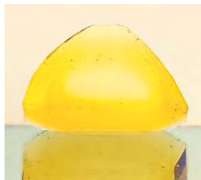
Figure 12. When immersed in methylene iodide, this nearly 20 ct sapphire shows an orangy yellow layer of color following the outline of the facets, which indicates that it was subjected to a bulk-diffusion process.
