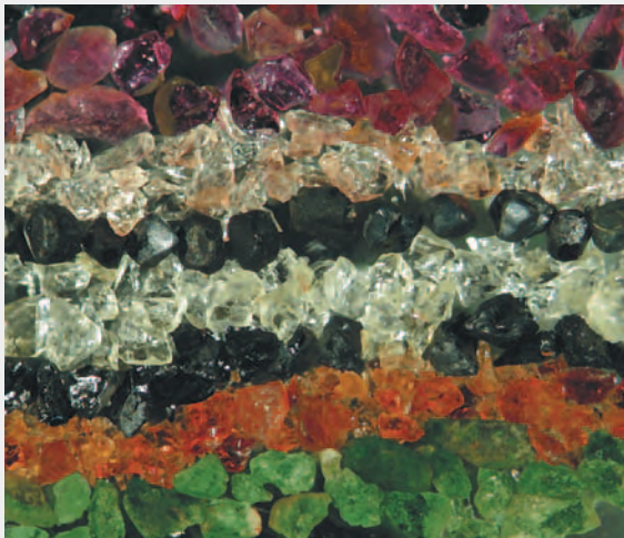
Figure A-2. Several indicator minerals are used to explore for kimberlites in Canada. These include, from top to bottom: Cr-pyrope garnet, eclogitic garnet, Cr-spinel, olivine, picroilmenite, Ti-pyrope garnet, and Cr-diopside. Photo by Penny R. Maki-Scott, Saskatchewan Research Council.
