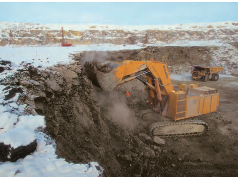
Figure 11. Shown here in winter 1998, diamond mining at Ekati's Panda pit is done with large excavators and trucks. The truck in the background can carry 240 tonnes of rock. Courtesy of BHP Billiton Diamonds Inc.
