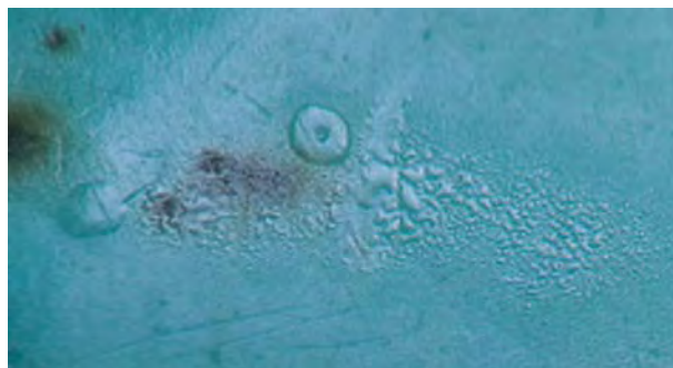
Figure 7. Crowningshield provided one of the earliest reports on the “sweating” of wax-treated turquoise when exposed to a hot point in a 1959 “Highlights at the Gem Trade Lab in New York,” a precursor to today’s Lab Notes section. Photomicrograph by Shane F. McClure; magnified 23×.
