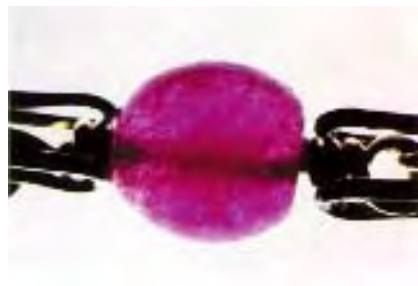
Figure 12. With diffused lighting, dye concentrations can be seen in this bead even without magnification (left). The dye concentrations in this aggregate are found in the spaces between and around the individual quartz grains, as well as in small surface-reaching fractures and fissures within the grains, as seen here at 120× (right).
