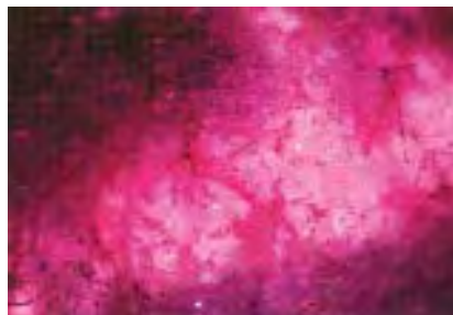
Figure 12. With diffused lighting, dye concentrations can be seen in this bead even without magnification (left). The dye concentrations in this aggregate are found in the spaces between and around the individual quartz grains, as well as in small surface-reaching fractures and fissures within the grains, as seen here at 120× (right).
