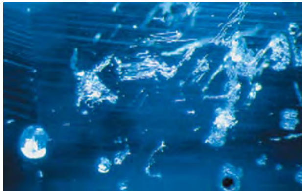
Figure 37. Elongated cavities in the synthetic spinel were oriented in two directions, at approximately 135° to one another. Also present were rounded negative crystals. Photomicrograph by H. A. Hänni, © SSEF; magnified 50×.
