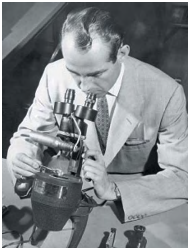
Figure 4. During his several decades in the laboratory, Bob Crowningshield used the microscope for many of his discoveries. This photograph, taken in the 1950s, shows him using an early-version Diamondscope, a binocular gemological microscope with lightfield and darkfield illumination that had been developed by GIA in the 1930s and ‘40s.
