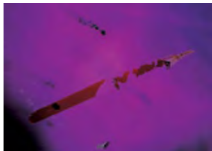
Figure 9. The most common inclusions observed in the Nigerian amethyst examined were deep red needles of hematite (left, magnified 10×). Thin plates of hematite also were seen occasionally (center, magnified 20×). The primary fluid inclusion on the right (magnified 15×) contains liquid and gaseous carbon dioxide, as shown by cooling and heating experiments. A "tail" of hematite extends from the base of this fluid inclusion. Photomicrographs by John I. Koivula.
