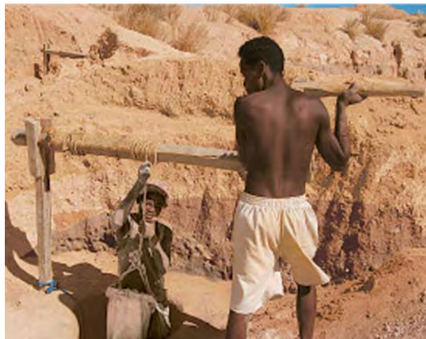
Figure 13. Narrow shafts in the Ilakaka region, some reaching 20–30 m deep, are accessed by primitive windlass systems. The miner sits inside a cloth bag, which is also used to raise the gem-bearing gravel to the surface. Photo by Brendan Laurs.
