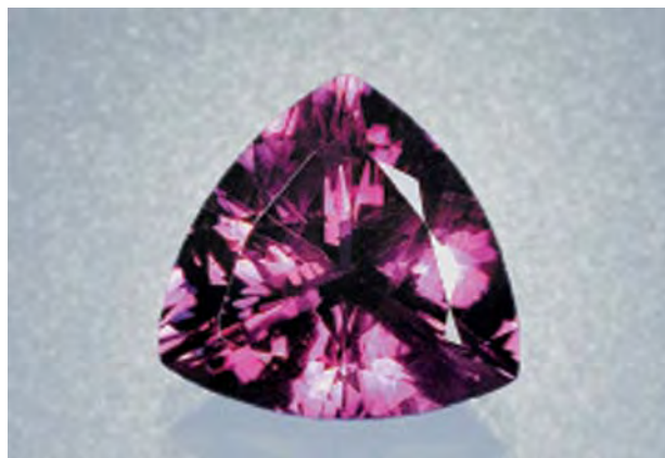
Figure 44. Amethyst from Thunder Bay, Ontario, fades with prolonged exposure to sunlight, but the color can be restored by X-ray irradiation. This color behavior is quite common for amethyst. The particularly fine example of Thunder Bay amethyst shown here is from the Panorama mine, and weighs 5.92 ct. Courtesy of Brad Wilson.
