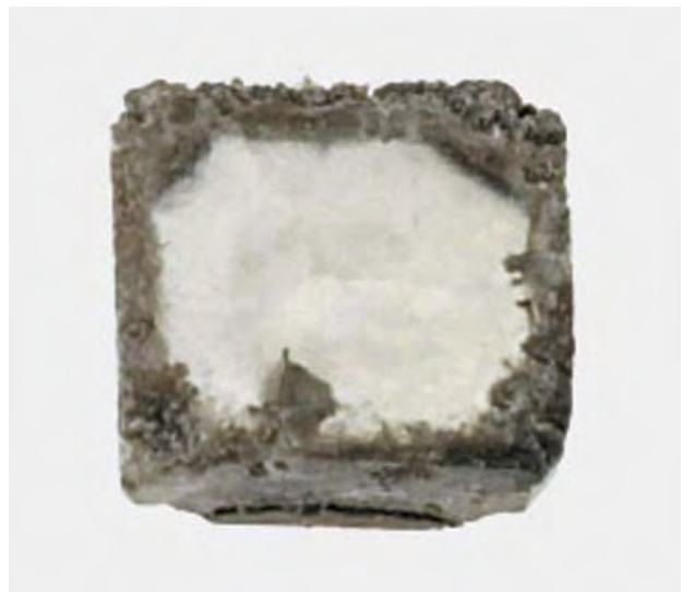
Figure 34. This very light brown 0.87 ct CVD laboratory-grown diamond crystal has a dark rim that is composed of diamond-like carbon or graphite. Courtesy of Apollo Diamond Inc.; photo by Elizabeth Schrader.
