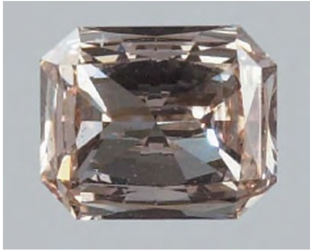
Figure 9. As these samples illustrate (left, no. 48921b at 0.14 ct; right, no. 49806b at 0.28 ct), the CVD-grown diamonds were faceted to get the best yield from the tabular crystals. The sample on the right, which was equivalent to Fancy brownish yellow, was cut from a near-colorless crystal (see table 1). It is likely that the color changed during faceting, as has been known to occur with natural diamonds. Photos by Elizabeth Schrader.
