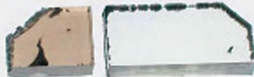
Figure A-3. A CVD synthetic diamond crystal was sawn in two, and the 0.18 ct as-grown portion on the left (no. 58768) was retained as a control sample while the 0.36 ct portion on the right was HPHT annealed. The brown as-grown sample became light gray after HPHT annealing. Photo by Wuyi Wang.
