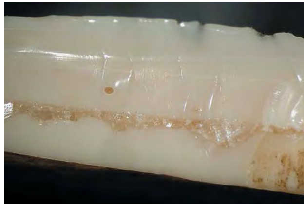
Figure 41. A broken fragment of the plastic "walrus tusk" showed conchoidal fractures, air bubbles, and a layer of crushed calcite crystals, proving its manufactured nature. Photo by H. A. Hänni, © SSEF.
