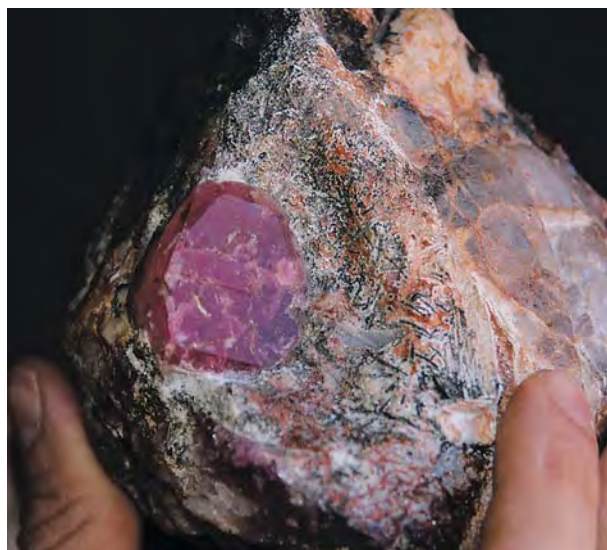
Figure 9. This pezzottaite specimen has been cleaned of dirt and clay, but otherwise shows the appearance as recovered from the mine. The pezzottaite crystal measures 3.6 cm in diameter, and is associated with “cleavelandite” feldspar (bladed albite, here partially covered with Mn-oxides) and quartz. Courtesy of Federico Pezzotta; photo by Brendan Laurs.
