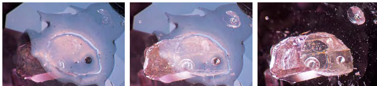
Figure 19. This sequence of photomicrographs shows two resin-filled cavities on the pavilion of a Sri Lankan spinel under different lighting conditions. In the left and center images—taken with darkfield and surface-reflected fiber-optic illumination, respectively—excess filler on the surface and its relationship to the filled cavities is evident. The image on the far right clearly shows the largest apatite-shaped cavity as well as the gas bubbles in the fillers in both pits. Magnified 10 \times .
