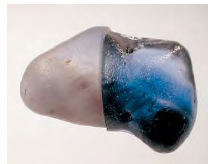
Figure 18. This 9.74 ct sample (approximately 16.1 \times 10.3 \times 6.3 mm) was sawn in two prior to the heat treatment experiment, and the half on the left was retained as a control. Note the dramatic change in color in the half on the right following treatment.
