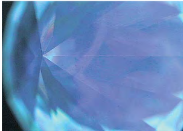
Figure 6. This De Beers DiamondView image of the Fancy Light yellow diamond with Ni-N-related optical centers shows irregular patterns of blue fluorescence, indicative of natural origin. Photo by J.-P. Chalain, © SSEF.
