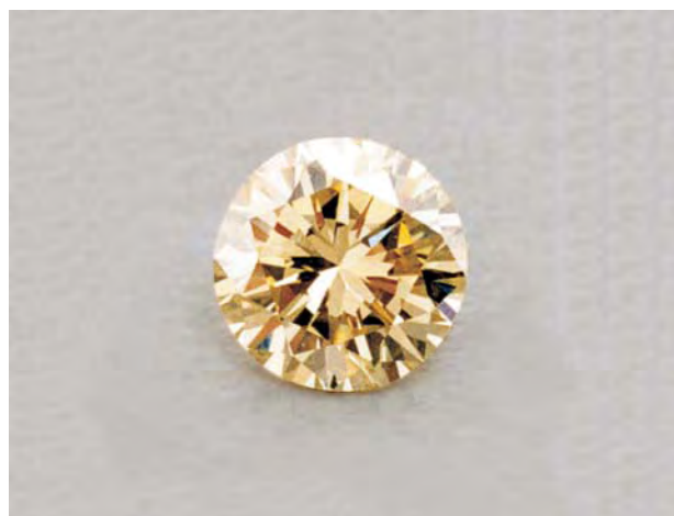
Figure 5. This 2.95 ct Fancy Light yellow natural diamond was found to contain Ni-related absorption features in the UV-visible region that have previously been associated only with synthetic diamonds. Photo by M. Krzemnicki, © SSEF.
