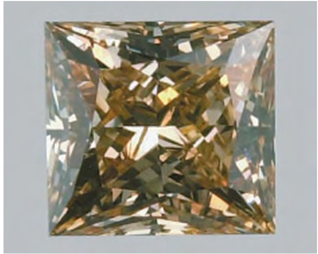
Figure 9. As these samples illustrate (left, no. 48921b at 0.14 ct; right, no. 49806b at 0.28 ct), the CVD-grown diamonds were faceted to get the best yield from the tabular crystals. The sample on the right, which was equivalent to Fancy brownish yellow, was cut from a near-colorless crystal (see table 1). It is likely that the color changed during faceting, as has been known to occur with natural diamonds. Photos by Elizabeth Schrader.
