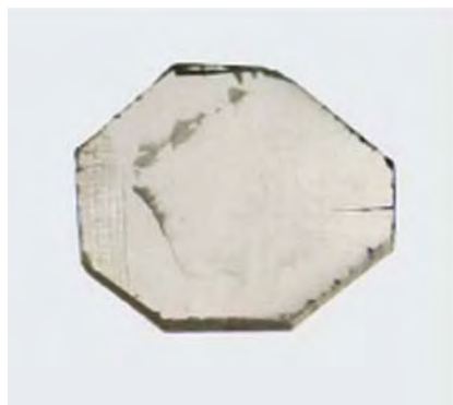
Figure 4. These CVD-grown synthetic diamond crystals illustrate the typical tabular shape of this material. The crystal on the left (no. 48921a) weighs 0.34 ct, while the one on the right (no. 56923) weighs 0.57 ct. The large, flat upper faces on both are the growth surfaces where new diamond material crystallized by chemical vapor deposition at high temperatures but low pressures. Photos by Elizabeth Schrader.
