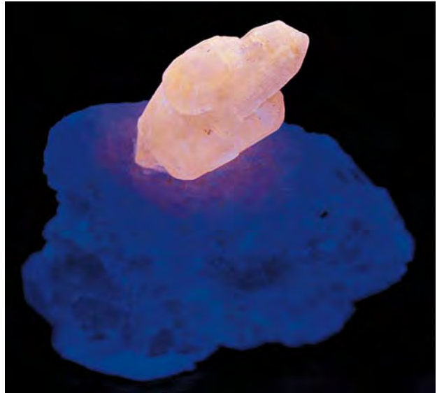
Figure 8. On exposure to long-wave UV radiation, the afghanite crystal in figure 7 fluoresced a strong, bright orange. Photo by Maha Tannous.
