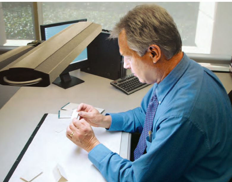
Figure 4. Diamond manufacturers and dealers typically view and assess diamond appearance and cut quality in offices with fluorescent desk lamps. Objects in the room, including the observer, can block or affect light shining on the crown of a polished diamond. Photo by A. Gilbertson.
