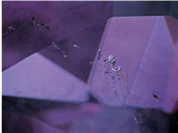
Figure 11. Primary fluid inclusions, such as those shown here, were common in the Four Peaks amethyst examined. The largest inclusion measures 0.7 mm long. Photomicrograph by J. I. Koivula.
