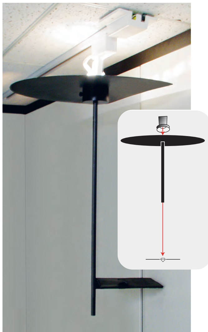
Figure 8. This configuration was used to train observers to see differences in fire in polished diamonds. Inset: In this schematic diagram, spot incandescent lighting from above is blocked and channeled into a long tube that shines a narrow beam of directed light onto a polished diamond. Photo by A. Gilbertson.
