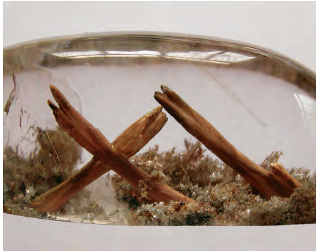
Figure 30. The faked inclusions form interesting patterns, and appear to emanate from areas of naturally occurring mica or chlorite within the quartz. Photo by J. Hyrsl.
