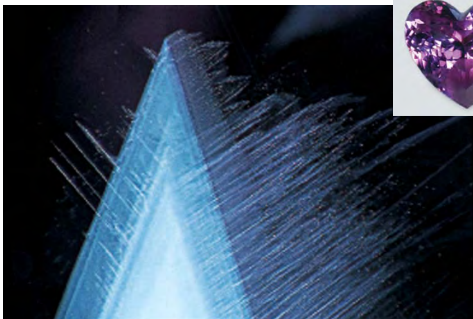
Figure 16. This 27.13 ct cut stone (inset; photo by J. Lowell) displayed an unusual white, wedge-shaped growth zoning pattern that was especially visible in reflected light when the sample was illuminated with a fiber-optic light source. Photomicrograph by J. I. Koivula; magnified 5 \times .
