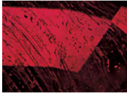
Figure 16. The glassy fillings in these clarity-enhanced rubies all contained numerous flattened gas bubbles (left) and elongated and irregular voids (right). Magnified 27 \times .
