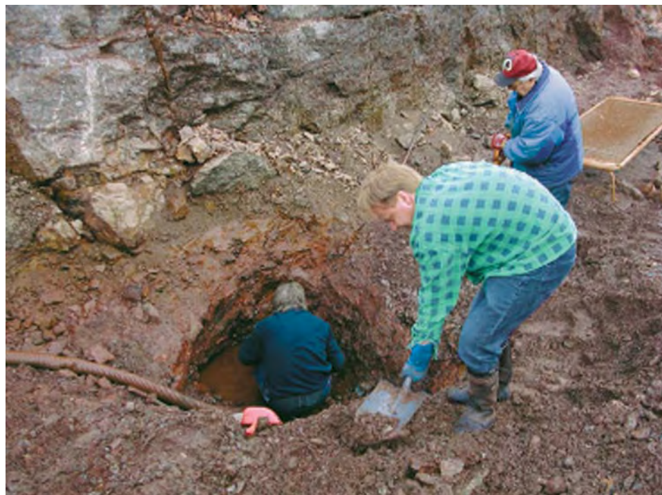
Figure 8. Mining activities have resumed at the gem beryl pegmatite near Luumäki, Finland. Heavy machinery is used to reach the gem-bearing zones, which are then carefully mined by hand to avoid damaging the crystals. Photo by P. Lyckberg.
