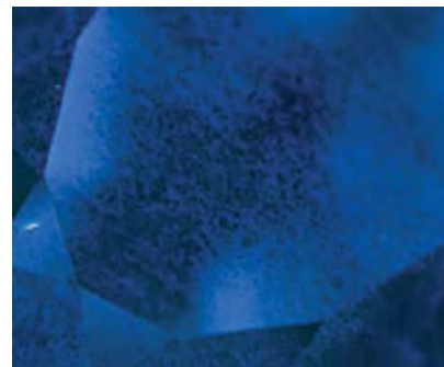
Figure 5. This luminescence image of the 2.60 ct oval-shaped diamond was collected using the De Beers DiamondView. A blue luminescence and networks of polygonized dislocations are evident; such dislocation networks are characteristic of natural diamond.
