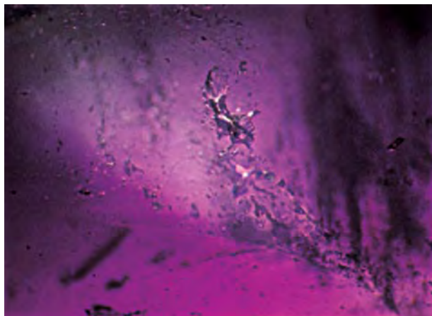
Figure 13. Veil-like patterns of secondary fluid inclusions were commonly observed in the amethyst samples studied. Photomicrograph by J. I. Koivula; magnified 20x.
