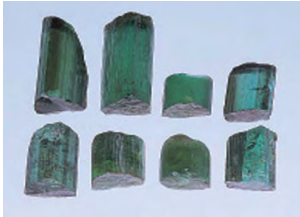
Figure 23. Heating experiments were conducted on the bottom portions of these four crystals of DR Congo tourmaline, while the top untreated portions were retained for comparison. All samples were heated in air as follows (from left to right, with weight of original crystal in parentheses): 427°C over a period of 5 hours (31.61 ct), 482°C over 6 hours (34.84 ct), 566°C over 8 hours (19.11 ct), and 621°C over 9 hours (19.89 ct). No appreciable change in the green-to-blue colors was seen in any of the heated portions, but abundant microcracks significantly reduced their transparency. Donated to GIA collection (nos. 30834–30837) by New Era Gems; photo by Maha Tannous.
