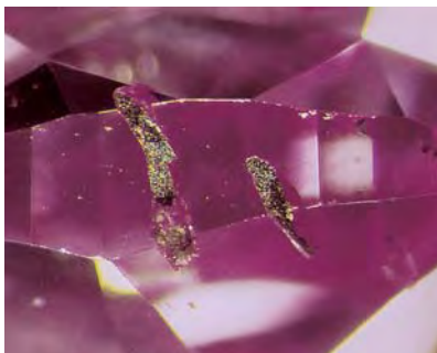
Figure 9. This photomicrograph shows the residue-filled surface cavities along the girdle of the diamond. Chemical analysis by EDXRF revealed the presence of Fe and Ca in the residue. Magnified 60 \times .
