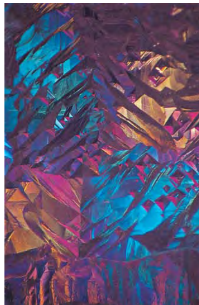
Figure 5. Viewed between crossed polarizers with 10× magnification, intense strain colors in the 2.03 ct diamond highlight the cubic etch pits and related surface contours.
