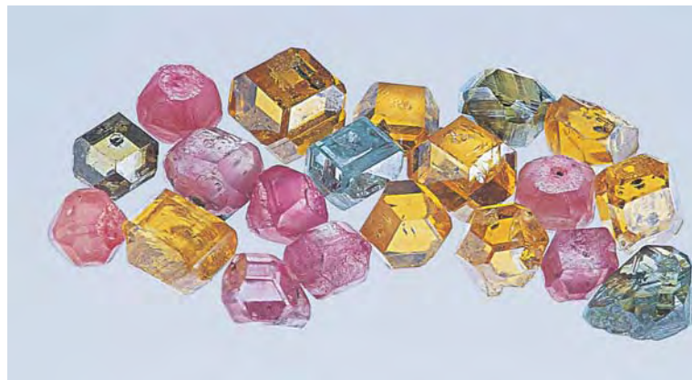
Figure 3. HPHT-grown synthetic diamond crystals are usually cuboctahedral in shape, as illustrated by these colored synthetic diamonds from Chatham Created Gems, which weigh between 0.44 and 1.74 ct. Photo by Maha Tannous.
