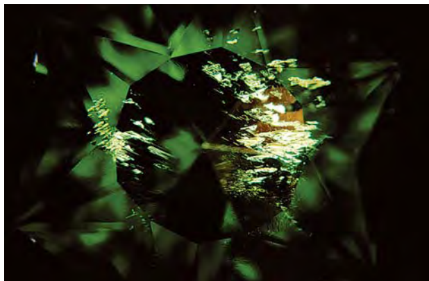
Figure 32. The inclusions in the Arizona peridot were grouped essentially parallel to one another, possibly due to crystallographic orientation. Photomicrograph by E. Fritsch; magnified 2 \times .
