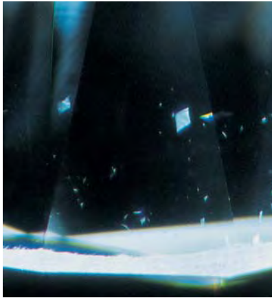
Figure 13. This 0.32 ct near-colorless synthetic diamond, submitted to the lab for a grading report, revealed opaque metallic-appearing inclusions, "pinpoints," and numerous parallelogram-shaped platelets. Reflected light, magnified 35 \times .
