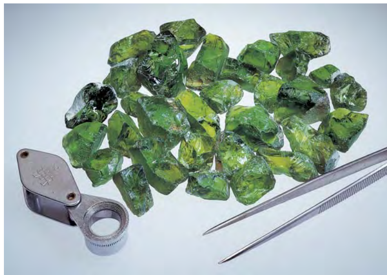
Figure 3. This representative selection shows 330 g (1,650 ct) of the larger peridot pieces from the 8 kg (40,000 ct) parcel, from which some of the gems seen on the cover and in figure 1 were cut. The rough has been placed on a light-box (typically composed of a translucent white plastic top, illuminated from below with fluorescent lighting), which is often used to evaluate colored gem rough. Photo by Jeff Scovil.
