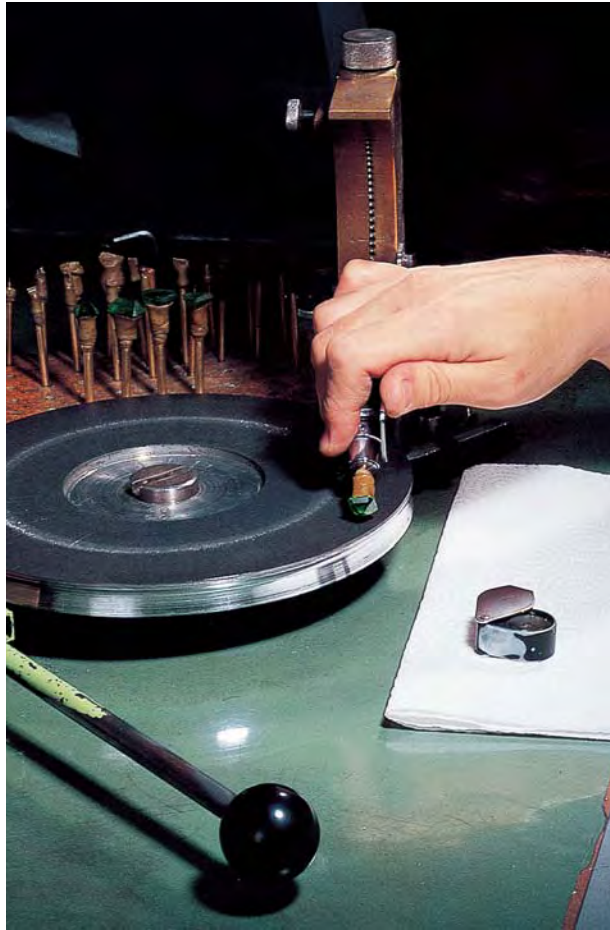
Figure 9. Once preformed, the pieces were delivered to the master cutter. Shown here is the slightly modified, classic Swiss jam-peg system that was used to facet the peridot suite. Photo by Jeff Scovil.
