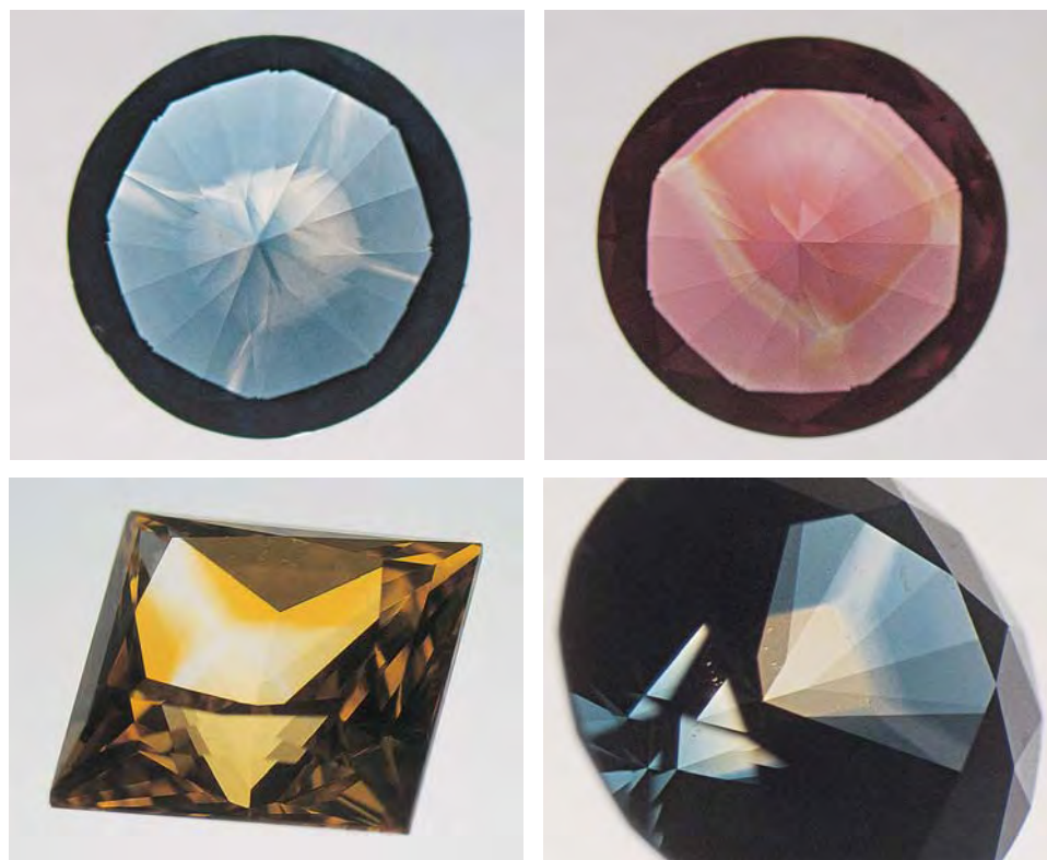
Figure 5. Colored synthetic diamonds often exhibit distinct color zoning due to differences in impurity contents between internal growth sectors. These four examples (0.17–0.68 ct) illustrate how these zoning patterns often appear as seen through the crown and pavilion facets. Immersing the material in a liquid (here, water) can aid in the observation of these patterns. Photos by J. E. Shigley; magnified 20 \times .
