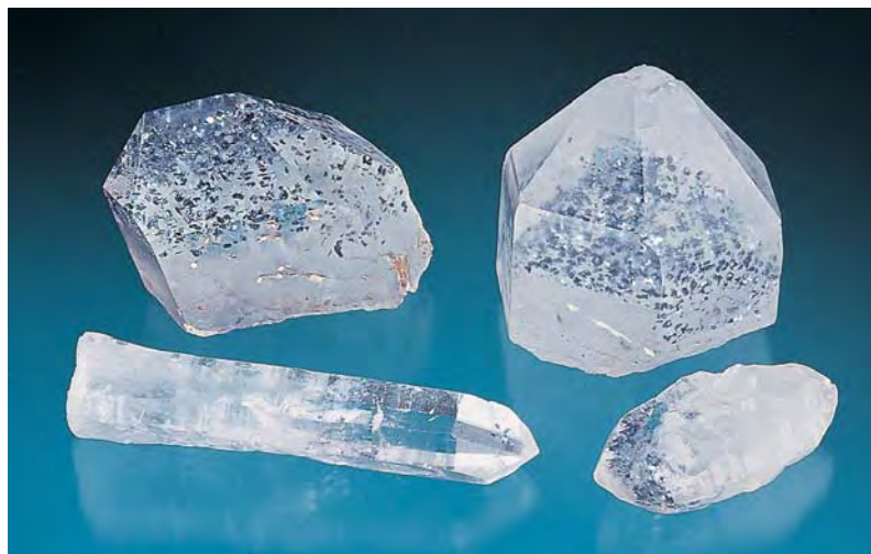
Figure 38. These Chilean quartz crystals contain phantoms formed by molybdenite inclusions. The largest crystal weighs 378.73 ct, while the longest one measures 65.8 mm. Courtesy of Russell E. Behnke and William W. Pinch; photo by Maha Tannous.
