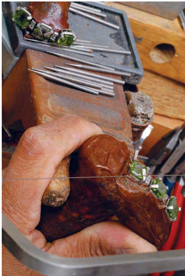
Figure 18. The setter uses a prong-pusher to bend the prongs one at a time over the crown at each corner (upper left). The prongs are then carefully shortened using a jeweler's saw (lower left and right). Photos by Robert Weldon.
