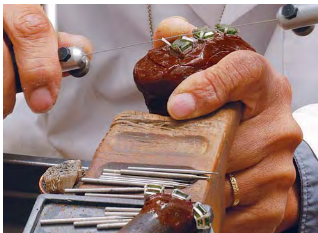
Figure 18. The setter uses a prong-pusher to bend the prongs one at a time over the crown at each corner (upper left). The prongs are then carefully shortened using a jeweler's saw (lower left and right). Photos by Robert Weldon.
