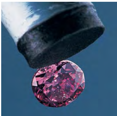
Figure 7. Because of iron-containing residue in surface cavities, this diamond could be suspended when touched by a magnet.
