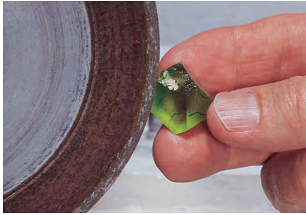
Figure 7. The sawn piece of rough is then ground against a diamond-impregnated wheel to produce the approximate shape and proportions of the finished gemstone. This step is crucial to the design of the final gem. Photo by Jeff Scovil.
