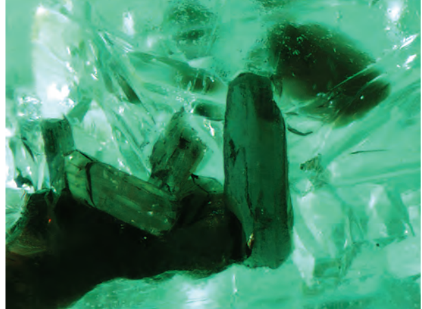
Figure 28. A few stones contained chlorite—like the crystal in the center here—as well as phlogopite. Photomicrograph by H. Zwaan; magnified 80 \times .
