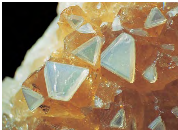
Figure 17. The adularescence shown by certain crystal faces of the heated citrine specimen provides an example of an interesting treatment-induced optical phenomenon. Photomicrograph by John I. Koivula for microWorld of Gems; magnified 10x.
