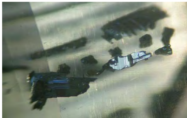
Figure 13. The bismuthinite inclusions in the rose quartz from Madagascar appeared metallic gray to black, and showed a variety of irregular forms. A network of needle-like inclusions, possibly rutile, was responsible for the asterism in this rose quartz. Photomicrograph by J. Hyrsl; the field of view is approximately 3 mm.
