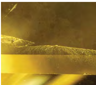
Figure 2. Heat treatment of the diamond in figure 1 may have created the unusual texture and flow structure visible within this fracture. Magnified 45x.
