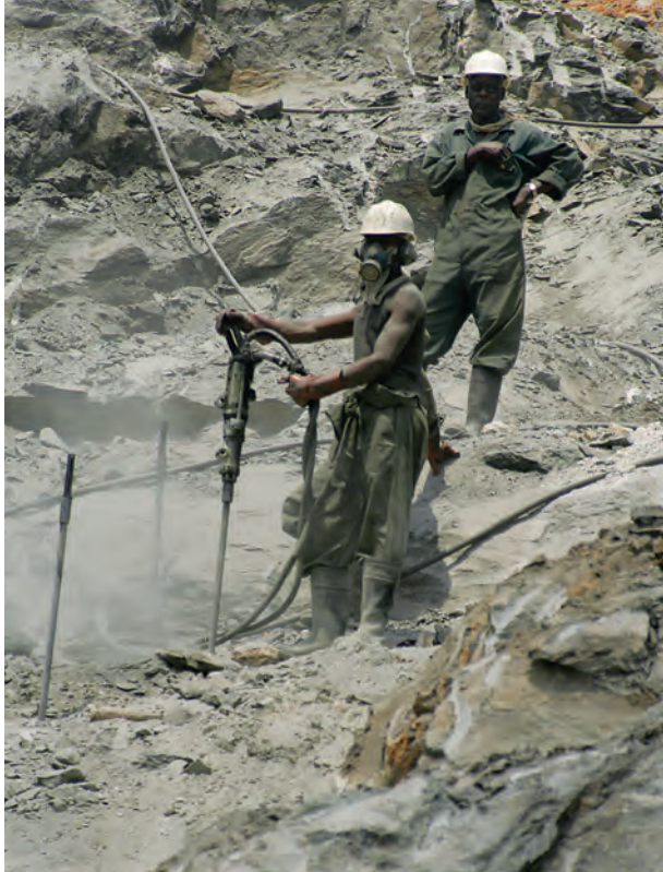
Figure 6. At the Grizzly mine, workers drill holes that will be filled with explosives to open up the area adjacent to an emerald-bearing zone. Photo by B. M. Laurs.
