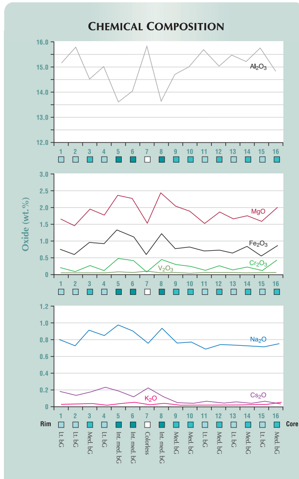
Figure 38. Electron-microprobe analyses of the Chantete emerald in figure 37 revealed systematic variations in the composition of the various growth zones. There was a good correlation between color and Cr content, with similar trends shown by Fe, Mg, and Na; the trends for all these elements were opposite that of Al. A significant increase in Cs was evident in the outer portion of the crystal.
