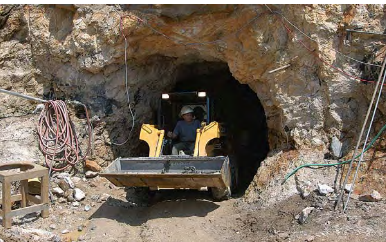
Figure 12. A small loader is used to remove pegmatite material from the underground workings at Mt. Mica. June 2005 photo by Brendan Laurs.
