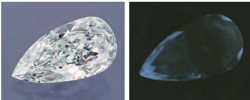
Figure 11. This 0.67 ct Light blue pear-shaped diamond (left) was submitted for a colored diamond grading report. A DiamondView phosphorescence image (right) shows weak blue phosphorescence concentrated near the head and point of the pear shape.
