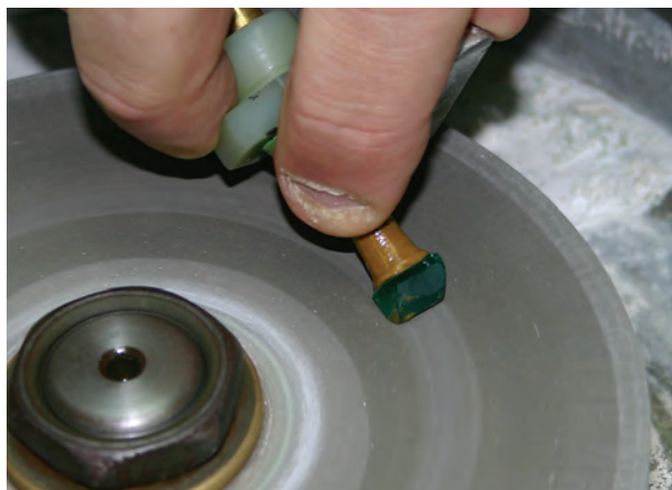
Figure 12. After they have been preshaped by Robogem, the emeralds are cut and polished by hand, using precise cutting and polishing wheels and equipment. Photo by H. Zwaan.
