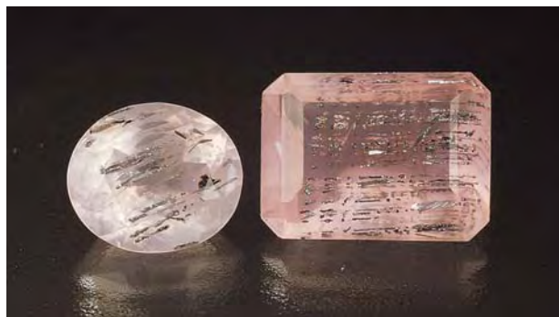
Figure 12. These faceted samples of rose quartz (5.74 and 12.55 ct) from the Itongafeno pegmatite in central Madagascar contain conspicuous inclusions of bismuthinite. Photo by J. Hyrsl.
