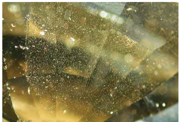
Figure 15. Some of the yellow hydrothermal synthetic sapphires showed "bread crumb" inclusions that were concentrated in a plane along the seed plate. These flake-like inclusions have not been seen in natural sapphires. Photomicrograph by G. Choudhary; magnified 30x.
