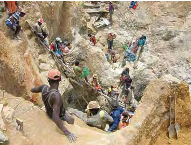
Figure 26. The main pit at Nandihizana measured about 75 m long and 14 m deep. The mined material was removed in buckets using ropes and ladders. Photo by F. Danet.
