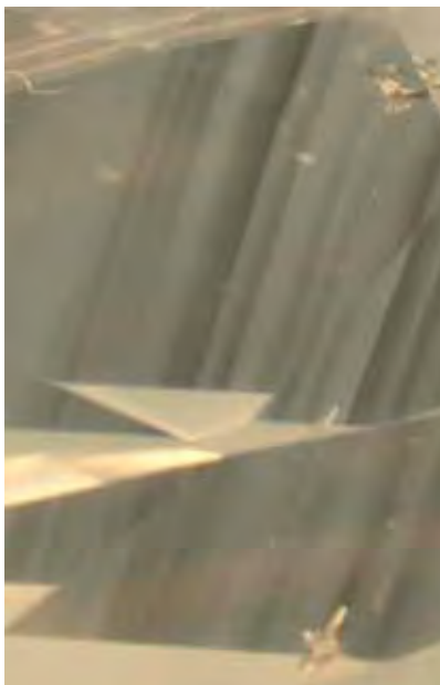
Figure 6. The submicroscopic inclusions in the diamond in figure 5 are concentrated in bands, something that is rarely seen in Fancy white diamonds. Magnified 15 \times .
