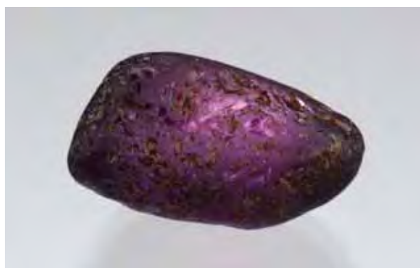
Figure 31. Although it has the appearance of a waterworn piece of gem rough, this 3.2 g sample was fashioned from synthetic sapphire. It was obtained in Tanzania from a multicolored parcel that was represented as Umba sapphire rough. Courtesy of Intimate Gems; photo by Robert Weldon.
