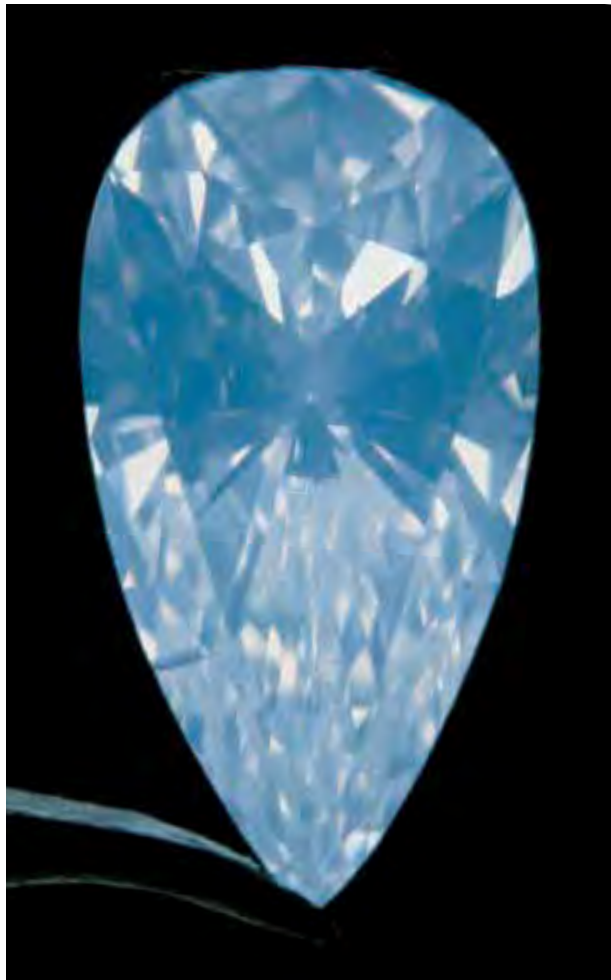
Figure 6. A whitish overall haziness believed to be the result of submicroscopic inclusions is also referred to as whitish graining in gemology. It appears to be related to the growth structure of the diamond. The transparency of this 5.68 ct diamond was noticeably affected when viewed face-up, which would result in a grade in the SI range even if no other inclusions were present. Photo by Vincent Cracco.
