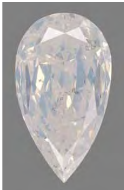
Figure 5. The color of this 30.87 ct Fancy white diamond is due to milky bands of submicroscopic inclusions. Also present are numerous partially graphitized stress fractures.
