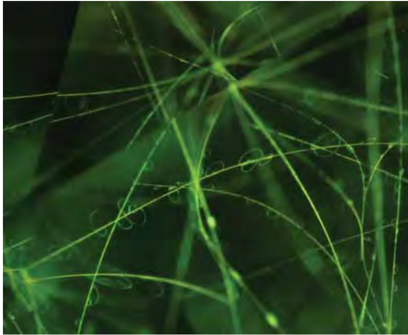
Figure 4. The demantoid in figure 3 contained striking inclusions composed of randomly oriented curved fibers encircled by small, bright, disc-like features. Magnified 50 \times .
