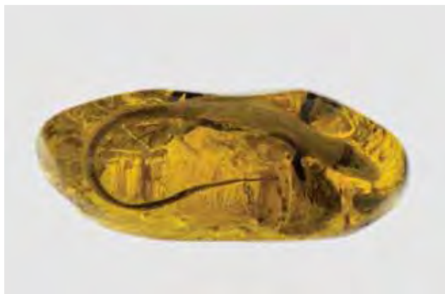
Figure 1. These two specimens proved to be imitations of amber with lizards enclosed. On the left, the lizard was encased in polystyrene; the sample on the right was an assembled piece consisting of a copal base, a plastic top, and a lizard molded between them.
