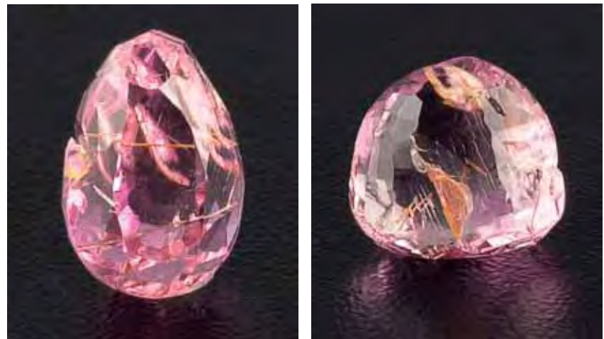
Figure 11. This 3.90 ct poudretteite (9.45 × 10.04 × 6.58 mm) is the first ever submitted to the GIA lab (face-up, left). Eye-visible orange-yellow epigenetic staining is present in both “fingerprints” and needle-like growth/etch tubes (pavilion up, right).
