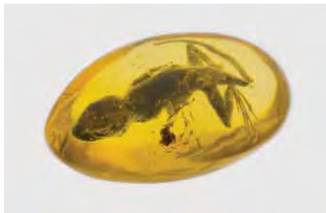
Figure 1. These two specimens proved to be imitations of amber with lizards enclosed. On the left, the lizard was encased in polystyrene; the sample on the right was an assembled piece consisting of a copal base, a plastic top, and a lizard molded between them.
