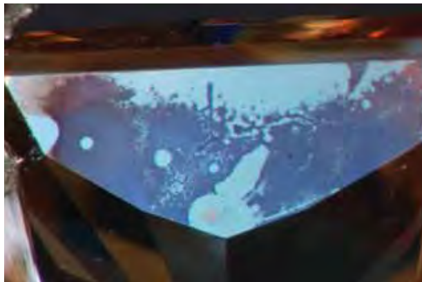
Figure 17. The film on the orange-coated diamond was damaged ("burned") over a relatively large area during the retipping process with a low-temperature solder. Photomicrograph by A. H. Shen; magnified 20 \times .
