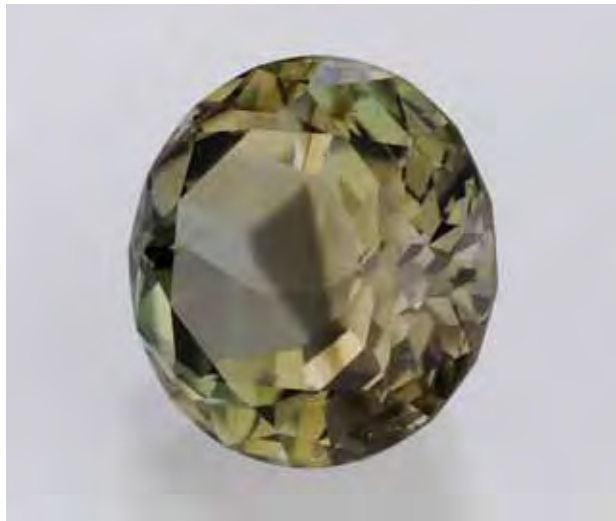
Figure 48. A distinct triangular color zone is visible in this 3.08 ct liddicoatite when it is viewed at an angle to the table. Courtesy of Intimate Gems; photo by Robert Weldon.
