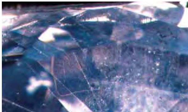
Figure 25. Sometimes surface features on the pavilion of a diamond are more visible when viewed through the table, as with these scratches in the coating on a 0.59 ct stone. Photomicrograph by S. F. McClure; magnified 26 \times .
