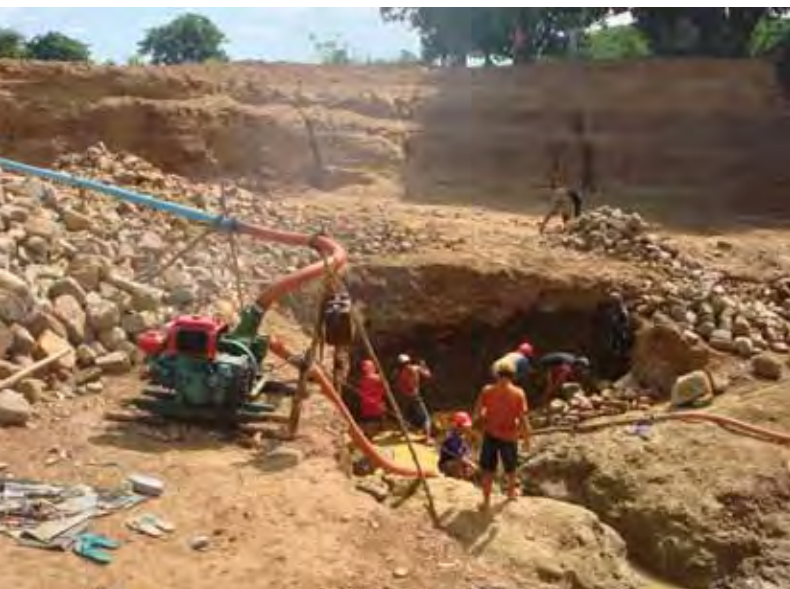
Figure 10. This alluvial mining operation for Piauí opal employs a pump to remove groundwater from the workings. Courtesy of Opalas Pedro II.
