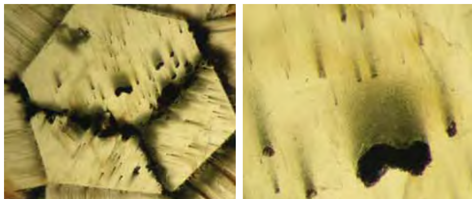
Figure 9. As seen here in transmitted light, two sets of growth channels are apparent in the trapiche tourmaline (left), one following the vertical growth direction of the pyramidal faces, and one nearly perpendicular to the prism. Some channels are empty, while others are filled with a black carbonaceous material (right). Photomicrographs by T. Hainschwang; magnified 10× (left) and 40× (right).
