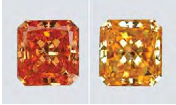
Figure 19. This orange-coated diamond (0.30 ct) was Fancy Vivid orange before the retipping test, but changed to Fancy Intense yellowish orange during exposure to the high-temperature solder. The sample also developed a burned appearance. Photos by Jian Xin (Jae) Liao (left) and Robison McMurtry (right).
