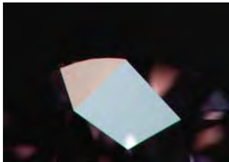
Figure 26. These coatings often have a bronze-colored appearance when viewed in reflected light (left), which makes their presence obvious when compared to the reflected-light appearance of an uncoated facet, here seen on the crown of the same diamond (right). Photomicrographs by S. F. McClure; magnified 23 \times .
