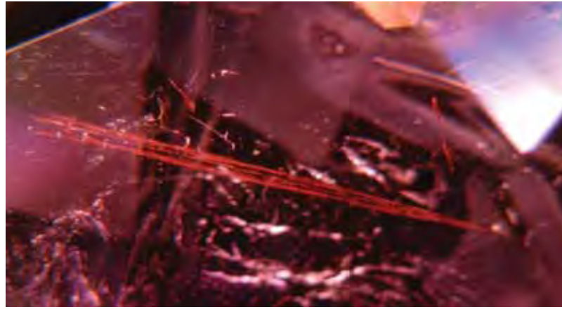
Figure 20. The DRC amethyst contained sprays of reddish needles that resemble the hematite inclusions commonly encountered in amethyst. Photomicrograph by Robert Weldon; magnified 10 \times .
