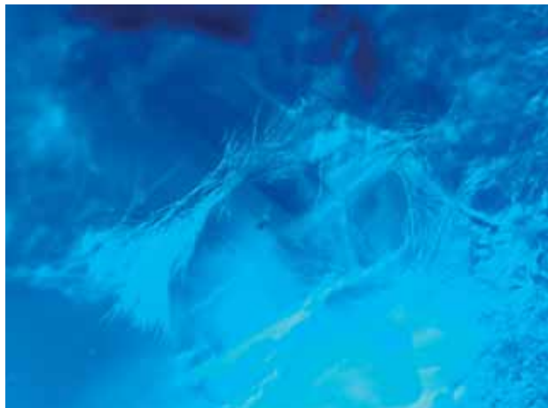
Figure 35. The blue glass pebble contained devitrified crystalline masses, which could incorrectly suggest a natural origin. Photomicrograph by E. A. Fritz; field of view 1.6 mm.
