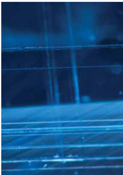
Figure 17. Unlike corundum growth tubes, which intersect at 60°/120°, growth tubes in kyanite intersect at 90°. Width of view 1.2 mm.
