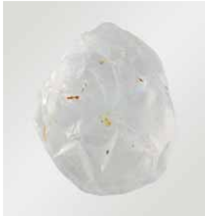
Figure 19. This crystal ( 27.30 \times 21.10 \times 19.10 mm), originally thought to be a diamond, proved to be phenakite.
