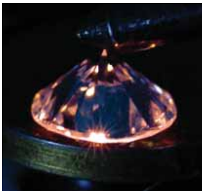
Figure 11. Orange-red sparks (electroluminescence) were obvious when the blue diamond was tested using a standard gemological conduction meter.
