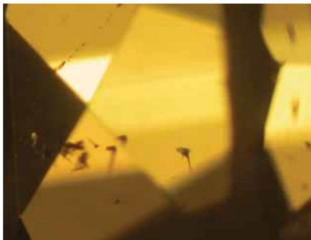
Figure 12. This diamond contains some nail-head spicule-like inclusions that are actually crystals with stress cracks at one end. Given the formation conditions of diamond, true nail-head spicules are not possible. Photomicrograph by C. Golecha; magnified 30 \times .
