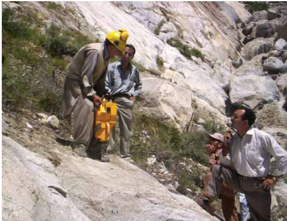
Figure 27. Drilling and blasting are used to prepare for an underground mining operation at the Ahmadabad ruby mine. Photo by Jim Clanin.
