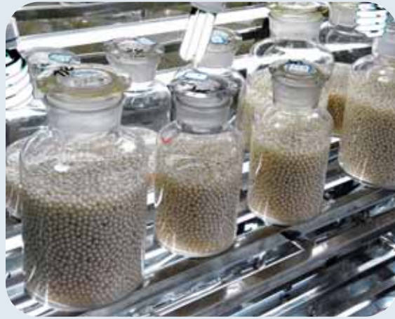
Figure A-1. Virtually all akoya cultured pearls are bleached to improve whiteness. The process involves immersion in a heated hydrogen peroxide solution combined with fluorescent illumination. Photo by Niels Ruddy Hansen.
