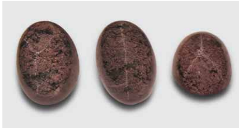
Figure 19. Depending on the viewing angle or the location of the light source, several subtle chatoyant bands can be seen in this 44.85 ct quartz cabochon from Brazil (shown in three different viewing positions). In the center, the cabochon is seen face-up with the light source perpendicular to the dome. The views on the left and right show the effects of moving the light source and tilting the stone, respectively. Photos by T. Hainschwang.
