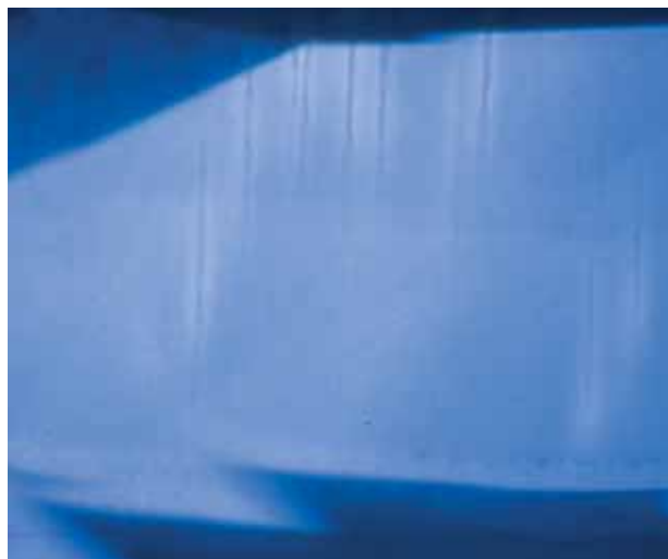
Figure 37. In a process referred to as chromophore cannibalization, the color of this blue sapphire is bleached directly adjacent to the parallel needle-like inclusions, indicating that the inclusions possessed a higher affinity for the chromophoric elements (Fe and Ti) than their sapphire host. This provides proof that the host sapphire is of natural color and that no heat treatment has taken place. Photomicrograph by J. I. Koivula; field of view 1.1 mm.
