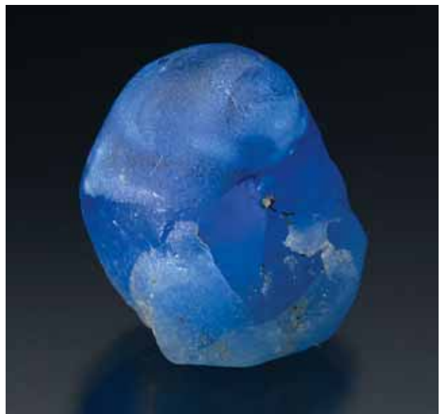
Figure 34. This 5.5 g pebble was represented as blue spinel from a new deposit in Afghanistan, but proved to be Co-bearing glass. Gift of Intimate Gems, GIA Collection no. 37273; photo by Robert Weldon.
