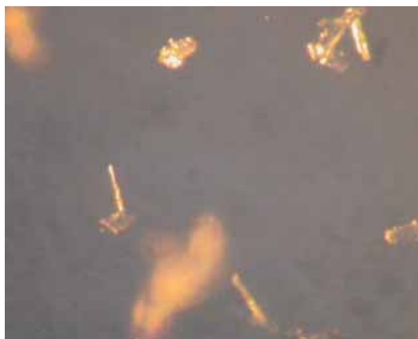
Figure 14. The aggregation patterns of these inclusions in quartz strongly resemble nail-head spicules at certain orientations. Photomicrograph by C. Golecha; magnified 35 \times .
