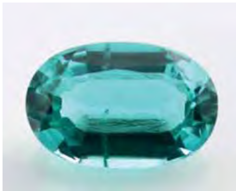
Figure 35. Tairus Created Gems represented this synthetic beryl crystal (0.5 g) and oval cut (0.42 ct) synthetic beryl as “Synthetic Paraíba,” an imitation of the highly valued copper-colored tourmaline. The characteristic wavy surface of the crystal and the undulating chevron patterns in the faceted specimen indicate hydrothermal origin. Photos by C. Golecha.
