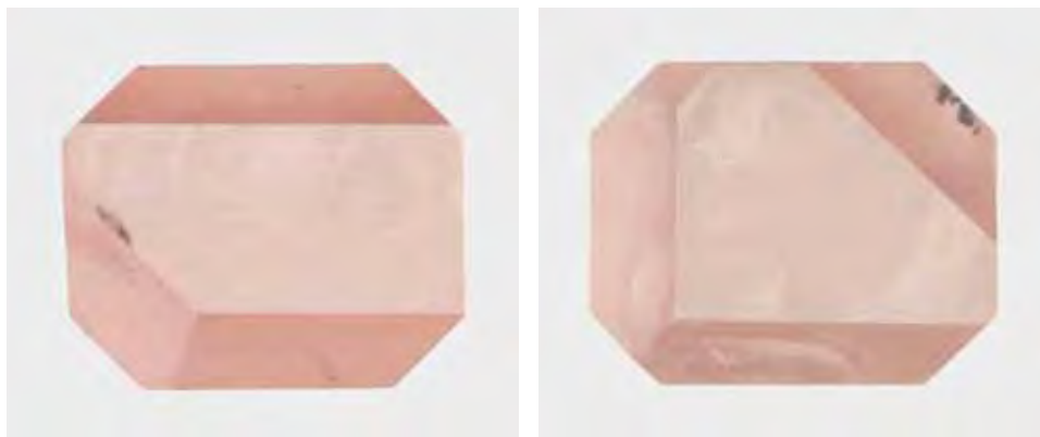
Figure 3. These two partially polished CVD crystals (1.05 and 1.20 ct) had a tabular morphology that is characteristic of CVD synthetic diamonds. Photos by Jian Xin (Jae) Liao.
