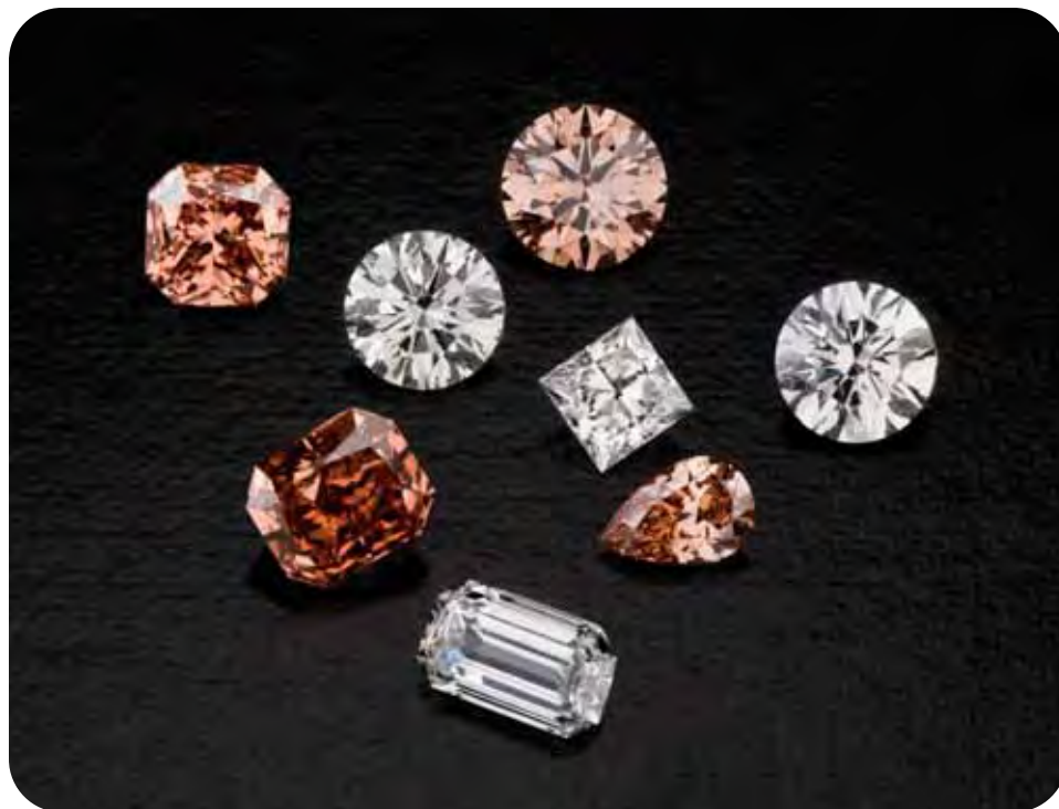
Figure 1. The latest-generation CVD synthetic diamonds produced by Apollo Diamond Inc., which are now available in the gem market, showed significant improvement in quality compared to those reported by Wang et al. in 2003. These representative samples weigh 0.24–0.67 ct. Photo by Robert Weldon.
