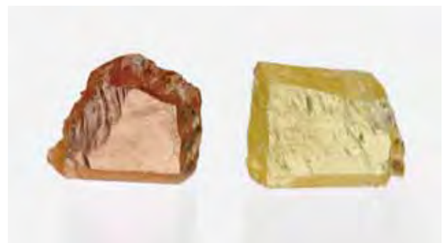
Figure 18. These two slabs (~8 mm tall) were cut from the same piece of rough, and oriented with the c-axis in the plane of the slices. The brownish orange slab is unheated, while the yellow slice was heated for two hours at 550°C.
