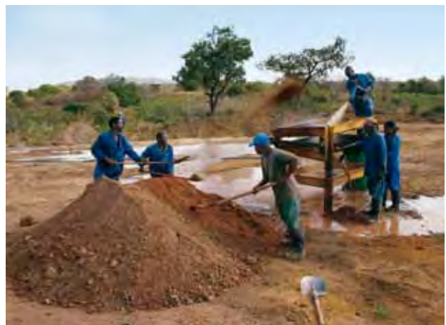
Figure 31. Material from test pits on the Mozambique Gems claim is first wet-screened and then hand picked for tourmaline. Photo by J. C. Zwaan.
