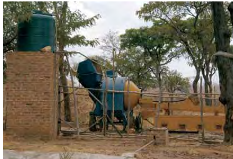
Figure 7. The washing plant that is also used to process material from the secondary deposits consists of a cement mixer followed by a series of vibrating screens. The water tank is filled from a small reservoir made in a seasonal stream that flows through the mining area. Photo by B. M. Laurs.
