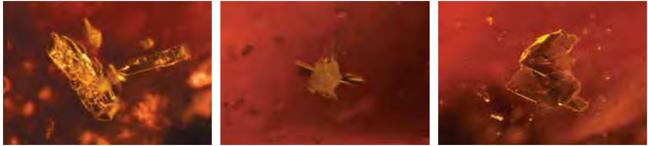
Figure 10. Transparent angular crystals of quartz were relatively common inclusions in the spessartine from Tanzania (left, field of view 0.8 mm). The translucent white spheroidal mass (center, 0.09 mm in diameter) was identified by Raman analysis as zircon; it is surrounded by minute tension fractures. Less common were angular subhedral inclusions of transparent-to-translucent brown mica (right, 0.63 mm in longest dimension). Photomicrographs by J. I. Koivula.
