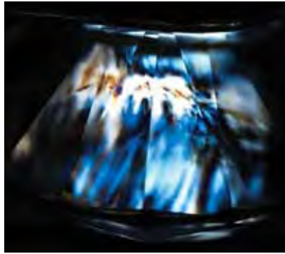
Figure 4. Examination between crossed polarizers revealed an irregular strain pattern in this CVD synthetic diamond, which was submitted to the Carlsbad lab for a grading report. Field of view 3.7 mm.
