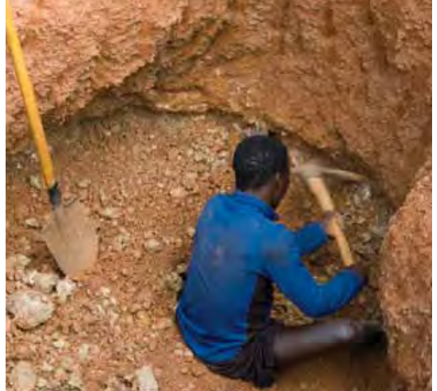
Figure 12. When they reach the tourmaline-bearing layer, the miners search for the gems by digging through the gravels with a pick. Photo by B. M. Laurs.
