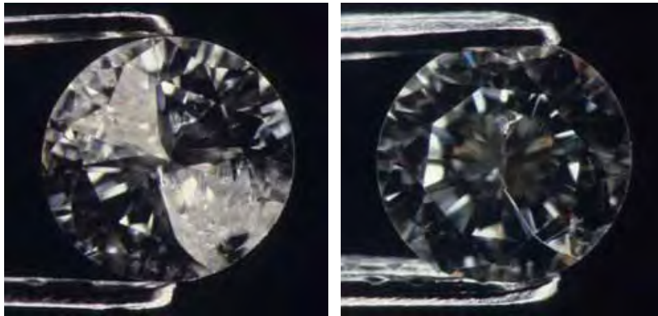
Figure 16. Introduction of a glass filler into this 0.30 ct diamond's cleavage cracks produced a dramatic change in apparent clarity (before filling, left; after filling, right). Photomicrographs by John I. Koivula.
