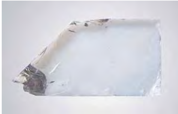
Figure 16. This 0.81 ct piece of light blue rough, originally sold as tanzanite, proved to be manganaxinite. Photo by J.-M. Arlabosse.
