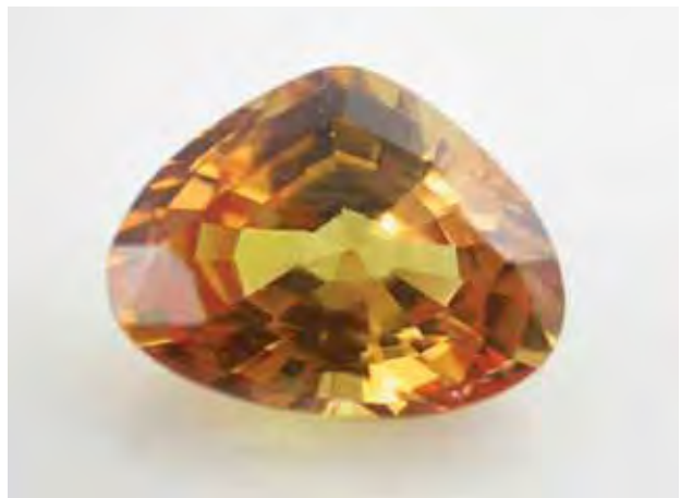
Figure 28. This 4.78 ct synthetic sapphire shows a brownish orange color similar to that observed in beryllium diffusion-treated corundum.
