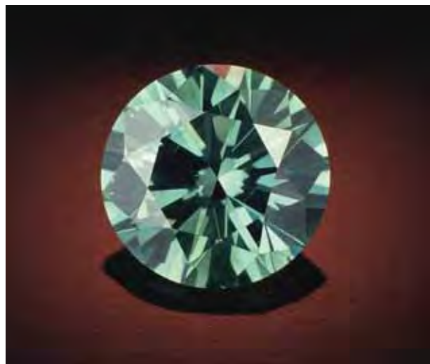
Figure 3. This attractive green diamond (3.06 ct) owes its color to irradiation. Photo by Robert Weldon.
