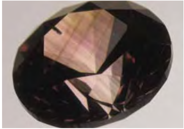
Figure 5. Intersecting sets of purple and brown lamellae can be seen in this 0.43 ct Fancy brownish purple-pink diamond. Photomicrograph by J. E. Shigley; magnified 5 \times .
