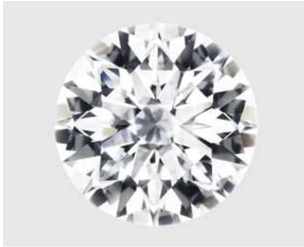
Figure 2. This 0.54 ct colorless type IIa diamond showed strong phosphorescence. Photo by H. Ito.
