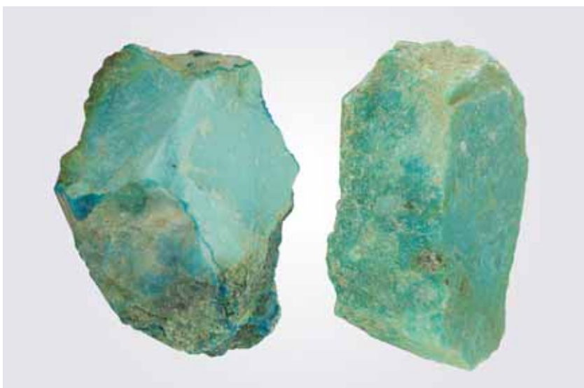
Figure 10. Chemical analysis of these two samples of bluish green plagioclase feldspar (45.38 and 46.90 mm in longest dimension) suggested that they were colored by copper.
