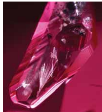
Figure 14. Another included crystal (identified as corundum) in the ruby contained a fan-shaped spray of needles. Field of view 0.63 mm.
