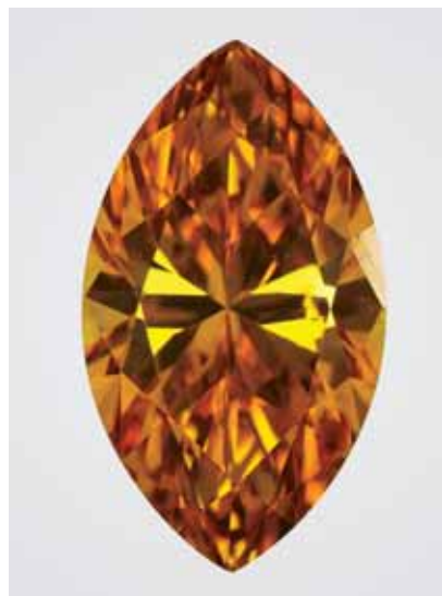
Figure 1. The deep orange color of this 0.90 ct treated diamond was likely influenced by a very strong 594 nm absorption.
