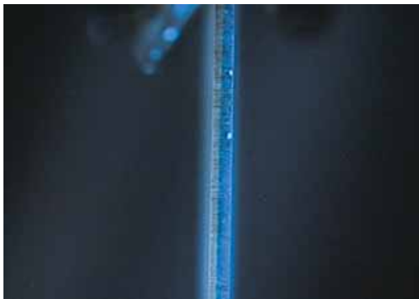
Figure 52. Sample A, when observed from the side in the DiamondView instrument, shows two different fluorescence zones, a sign of growth in layers. Photo by P. Lefèvre, © SSEF.
