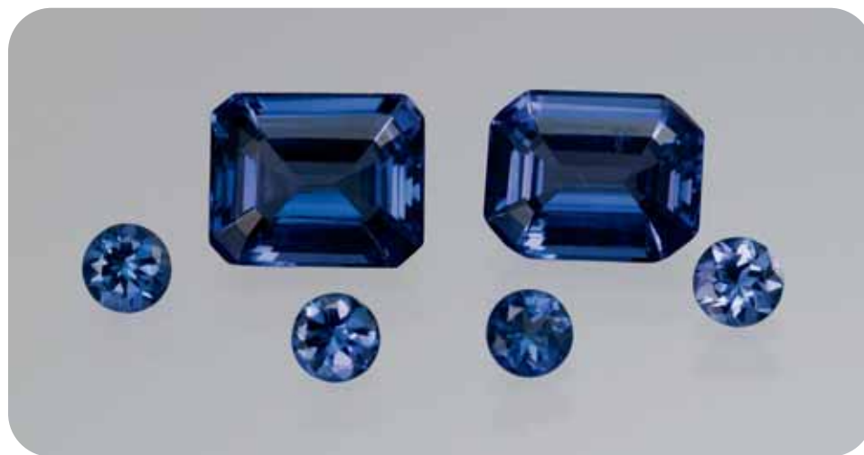
Figure 2. Omi Gems brought these tanzanites to the lab's attention because they suspected some form of treatment. Even the 4–5 mm stones were strongly colored. All proved to be coated, but it was very difficult to detect the coatings on the two larger tanzanites (3.01 and 3.21 ct). Photo by C. D. Mengason.
