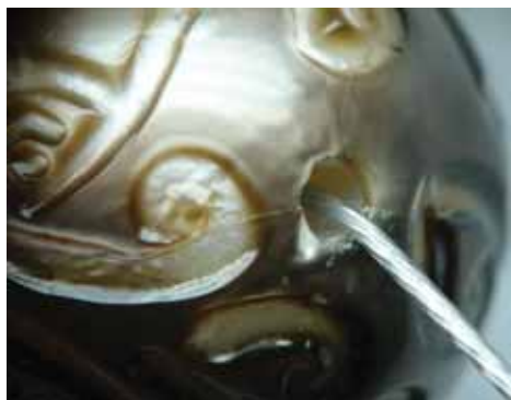
Figure 25. With reflected light, it was obvious that the cultured pearls had been coated with a transparent, colorless substance (left, magnified 20 \times ). Small fissures and exposure of the white shell bead nucleus were seen in areas with thin nacre (right, magnified 12 \times ). Photomicrographs by S. Singhamroong, © Dubai Gemstone Laboratory.
