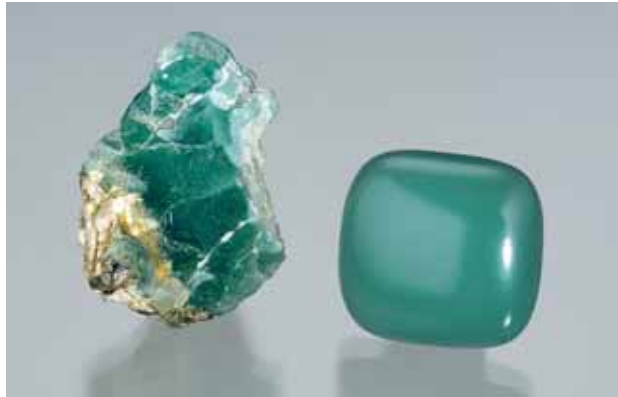
Figure 18. These Cr/V-bearing mica samples (3.33 g and 16.54 ct) from northern Pakistan were identified as consisting predominantly of paragonite. Photo by Robert Weldon.
