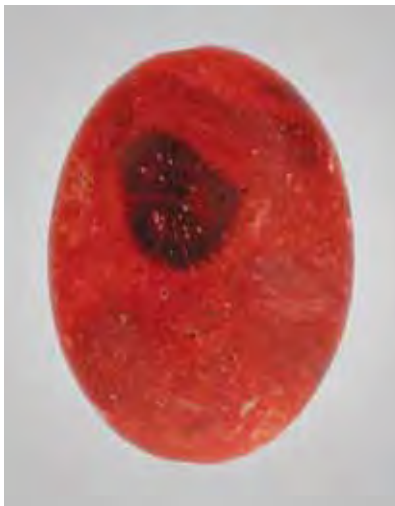
Figure 4. Unlike the bead in figure 3, this sample (8.65 ct) proved to consist of pieces of coral and other natural materials held together with a plastic binder.
