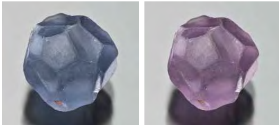
Figure 3. Resembling color-change garnet from Bekily, Madagascar, this ~1 cm fluorite is violetish blue in daylight (left) and purplish pink in incandescent light (right). Photos by Robert Weldon.
