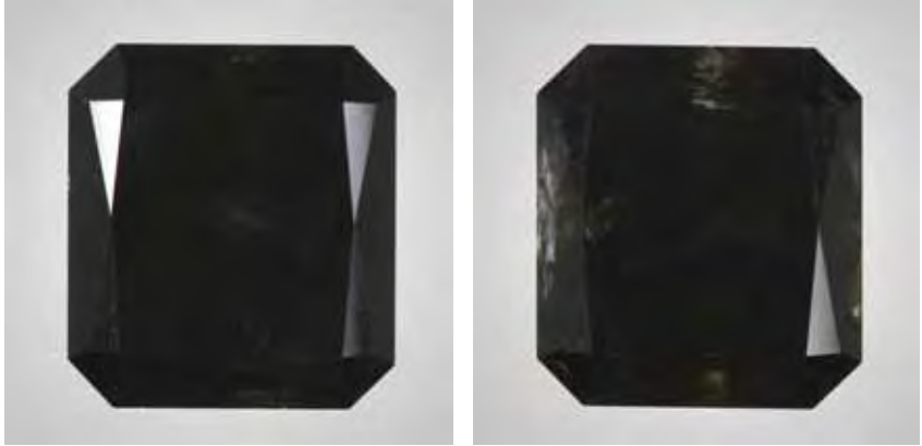
Figure 6. The black color of these diamonds (2.69 and 2.72 ct) was caused by dense inclusions of hydrogen clouds.
