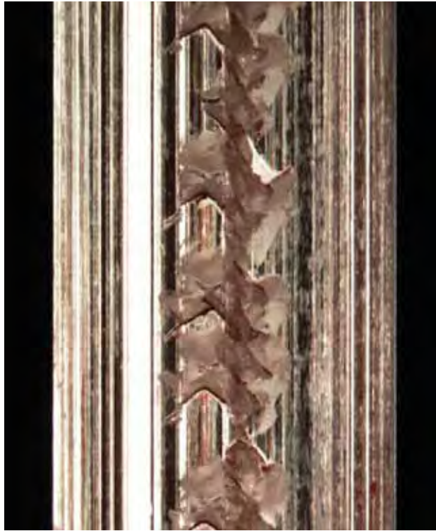
Figure 43. The spiral dislocation pattern appeared to be epigenetically filled with off-white to reddish brown debris that was probably a mixture of clay minerals and iron oxides. Photomicrograph by J. I. Koivula; field of view 9.7 mm tall.
