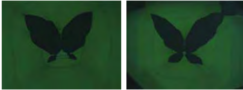
Figure 8. The symmetry of the DiamondView images indicates that the two black diamonds were cut from the same crystal. Butterfly ~3 mm wide.
