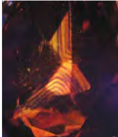
Figure 2. The Brazil-law twinning in this citrine is visible to the unaided eye using only fiber-optic light (left); it is also more easily seen with fiber-optic light than between crossed polarizers (right). Field of view ~7.9 mm.
