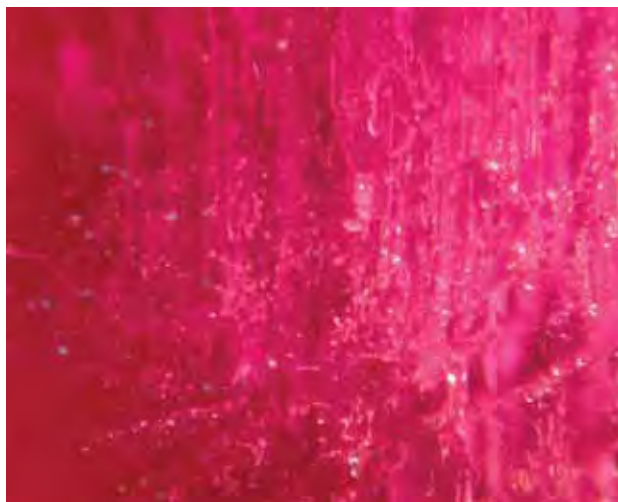
Figure 47. Some of the globular and tubular inclusions in the 3.50 ct synthetic ruby were not arranged in intersecting planes, as shown here. Also note the scattered blue pinpoints. Photomicrograph by G. Choudhary; magnified 80 \times .
