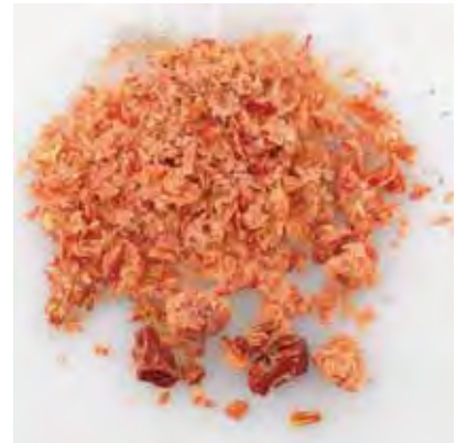
Figure 5. After it was soaked in methylene chloride to remove the plastic, the bead in figure 4 disintegrated into fragments.
