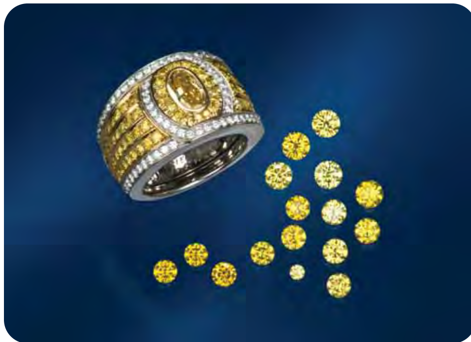
Figure 1. The loose synthetic diamonds shown here, from Chatham Created Gems (San Francisco), illustrate some of the yellows produced by HPHT growth. Many are similar in hue and intensity to the natural yellow diamonds in this ring, which is courtesy of Alan Friedman, Beverly Hills, California. The loose synthetics weigh 0.05–0.30 ct; the Fancy Intense yellow center diamond in the ring is 1.09 ct, and the 93 yellow melee weigh a total of 1.12 ct. Photo by Robert Weldon.
