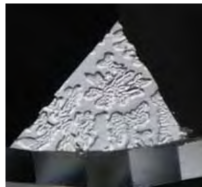
Figure 13. The burn on this extra facet resembles ferns or flowers and has surprising depth of relief, readily seen at the facet edges. Field of view ~0.7 mm.
