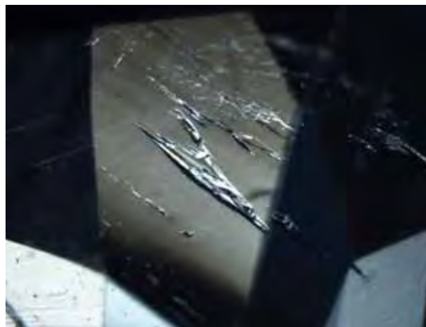
Figure 2. Multi-phase fluid inclusions are a common feature in natural aquamarine. Photomicrograph by C. P. Smith; magnified 65 \times .
