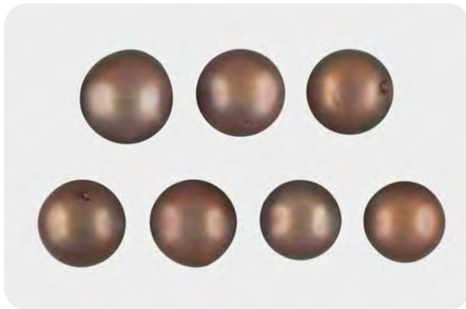
Figure 1. These seven Tahitian cultured Chocolate Pearls (10.50–12.53 mm), treated by Ballerina Pearl Co. using a proprietary bleaching method, were studied to evaluate their durability to various conditions of consumer wear. The samples are in order (CCP-1 to CCP-7) from left to right, top to bottom. Composite photo by Suchada Kittayachaiwattana.
