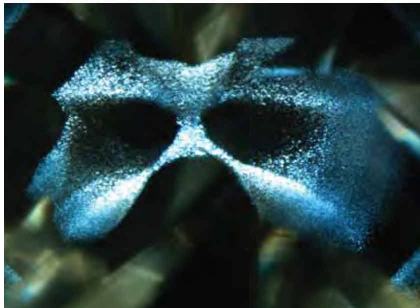
Figure 14. Discovered in a brownish green type Ia diamond, this hydrogen cloud has a unique three-dimensional shape reminiscent of a Venetian party mask. Field of view ~2.9 mm.
