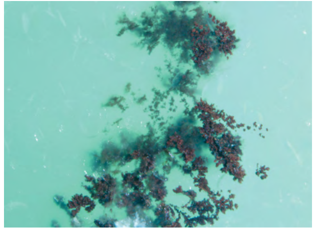
Figure 29. Interesting dendritic patterns are rarely seen in fashioned chrysoprase. In these samples, they were formed by inclusions of manganese oxides, which here appear red-brown in reflected light. Photomicrograph by R. Befi; image width 5.9 mm.
