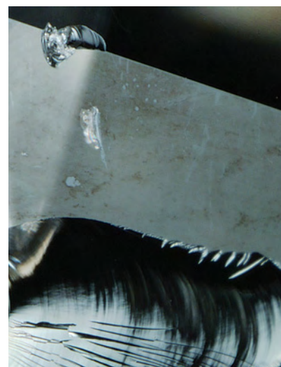
Figure 2. In reflected light, the coating on the surface of this 2.36 ct cubic zirconia is clearly visible. Also, the chips look conchoidal, in contrast to the typical step-like appearance of diamond. Field of view 1.7 × 1.3 mm.
