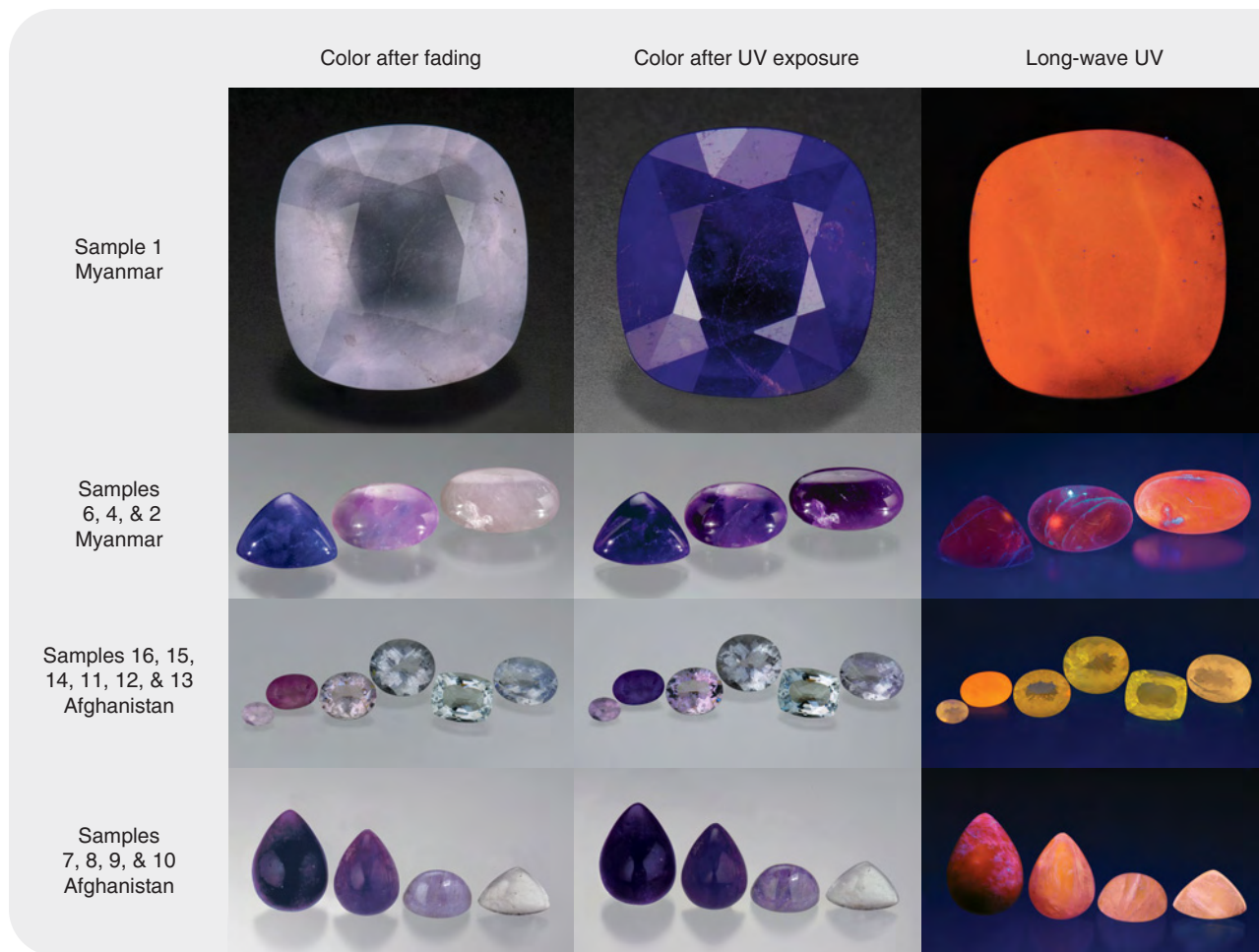
Figure 1. These samples of Burmese and Afghan hackmanite/sodalite, which were studied for this report, are shown in their desaturated color state, after exposure to short-wave UV radiation, and during exposure to long-wave UV. See table 1 for sample weights. Photos by Robert Weldon.
