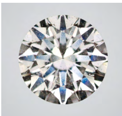
Figure 1. This 0.31 ct cubic zirconia from Serenity Technologies is reportedly coated with nanocrystalline synthetic diamond.
