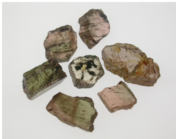
Figure 3. Seven andalusite specimens (0.81–3.87 ct) were polished as slices for inclusion studies and RI readings. Photo by G. Choudhary.
