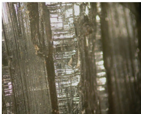
Figure 5. Many of the andalusite samples displayed strong etching that varied from irregular to square or rectangular (left). Also common were striations on the prism faces (right). The two-directional striations indicate the presence of twinning or various stages of overgrowth. Photomicrographs by G. Choudhary; magnified 60× (left) and 45× (right).
