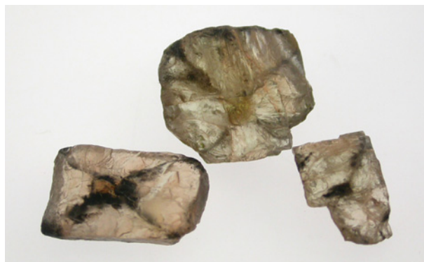
Figure 6. The chialstolite samples, here ranging from 3 to 6.5 mm thick, displayed a characteristic black cross pattern at the basal pinacoid with a square-to-rectangular core. The unusual transparency of these chialstolites made them particularly interesting. Photo by G. Choudhary.
