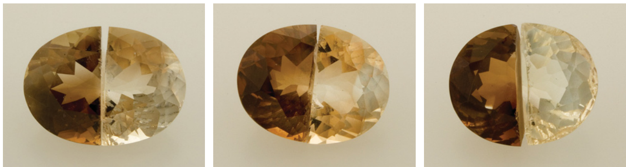
Figure 33. Three samples of brown topaz were sawn in half, and one piece from each pair was subjected to fade testing: in daylight for 80 hours (19.18 ct, left), in incandescent light for 80 hours (21.03 ct, center), and by exposure to long-wave UV radiation for 40 hours (21.29 ct, right). Thermal fading is probably responsible for some of the decolorization shown by the topaz exposed to the incandescent bulb. The UV-faded sample showed the most pronounced change. Composite photo by Adirote Sripradist.
