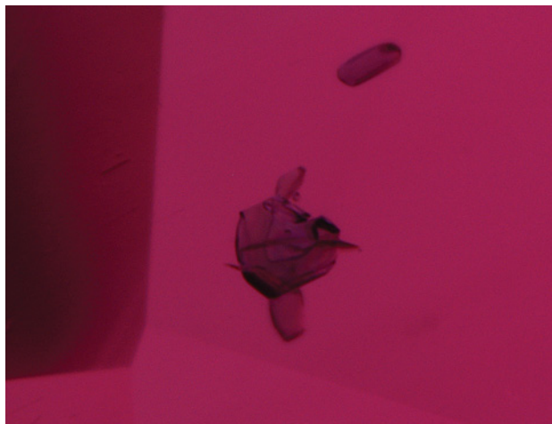
Figure 29. Rounded blue-gray to grayish blue crystals in a few of the Mozambique rubies yielded a Raman spectrum of an amphibole, close to that of pargasite. Similar inclusions are known to occur in Winza rubies. Photomicrograph by J. I. Koivula; the largest crystal is 0.17 mm long.
