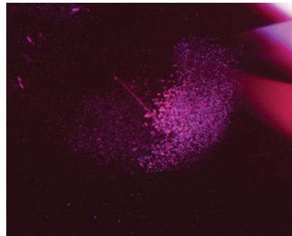
Figure 28. Some of the Mozambique rubies hosted epigenetically stained tubules and dense clouds consisting of reflective platelets and short needles that were reminiscent of sapphires from Uмба (left, image width 1.8 mm, by J. I. Koivula). Also seen were particulate clouds made up of small disk-shaped inclusions (center, image width 1.6 mm, by S. F. McClure). Dense planar clouds were present in several of the Mozambique rubies (right, image width 3.5 mm, by S. F. McClure).
