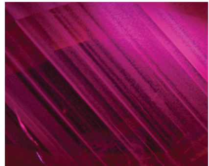
Figure 28. Some of the Mozambique rubies hosted epigenetically stained tubules and dense clouds consisting of reflective platelets and short needles that were reminiscent of sapphires from Uмба (left, image width 1.8 mm, by J. I. Koivula). Also seen were particulate clouds made up of small disk-shaped inclusions (center, image width 1.6 mm, by S. F. McClure). Dense planar clouds were present in several of the Mozambique rubies (right, image width 3.5 mm, by S. F. McClure).
