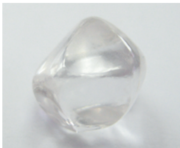
Figure 38. Despite its outward appearance resembling a natural octahedral diamond crystal, this 2.5 g sample is a synthetic sapphire. Photo by N. Ahmed, © Dubai Gemstone Laboratory.
