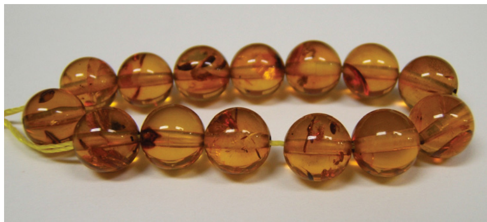
Figure 6. A yellowish brown color resulted from treating 14 beads of “lemon” yellow Colombian copal (1.03–1.05 ct) with an experimental two-stage heating process (180°C and 20 bars, at 20 hours for each stage). Photo by A. Abduriyim.
