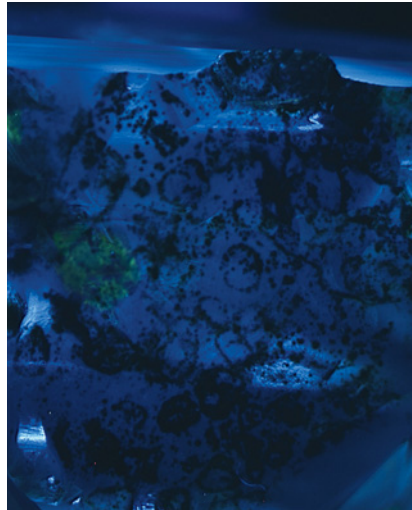
Figure 8. These green radiation stains, observed on the surface of a Fancy gray-green faceted diamond, exhibit patterns that resemble the outlines of grains that likely surrounded the stone while it was buried in an alluvial deposit (left). A DiamondView image from a different part of the same stone shows an overall blue fluorescence with inert zones corresponding to the location of the radiation stains (right). Left field of view is 3.23 mm high.
