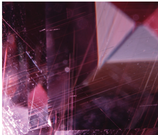
Figure 25. Oriented needles were present in the Kenyan color-change garnets. Photomicrograph by D. Beaton; field of view 2.6 mm.
