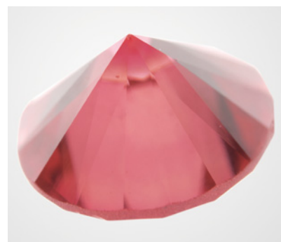
Figure 2. A distinct pink color zone is present at the culet of the red diamond, indicating irradiation and annealing at moderate temperatures to introduce NV centers.
